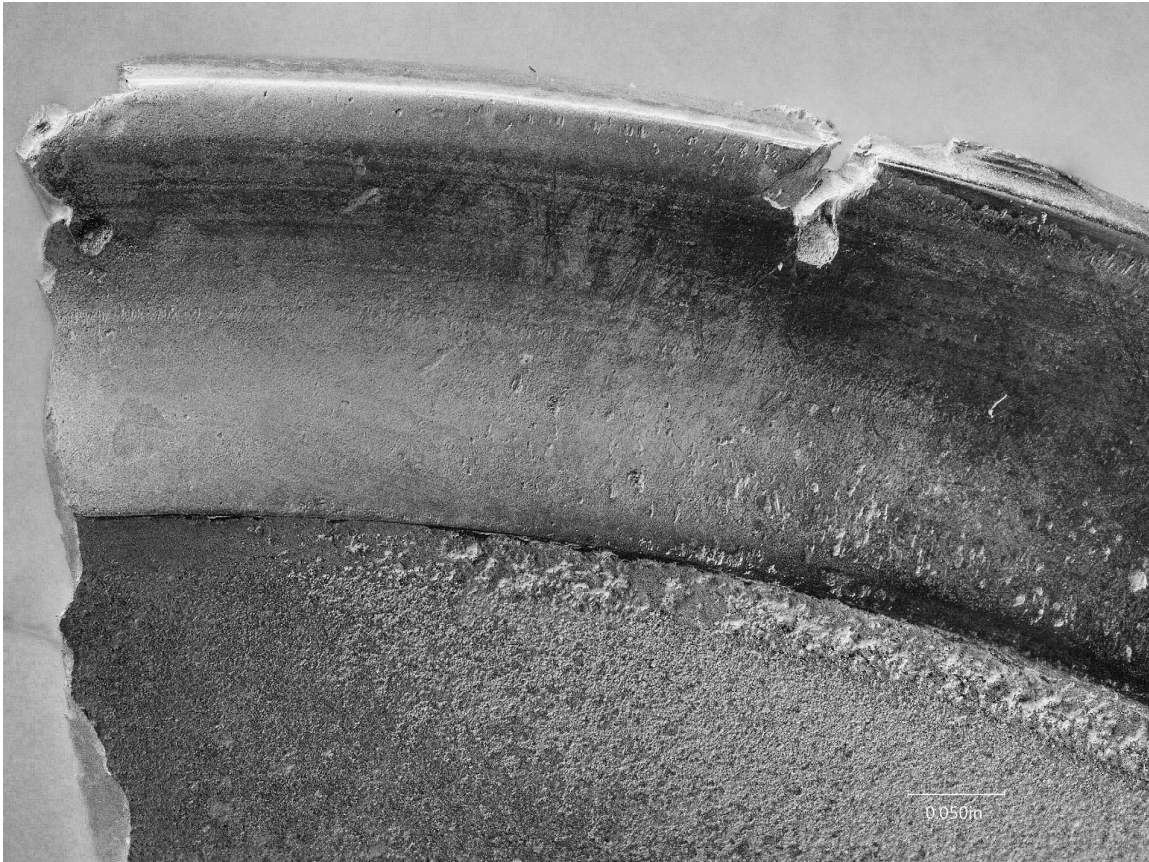
Figure 10 Digital microscope image of the seal face or seat of the valve near the origin of the radial rim crack.
