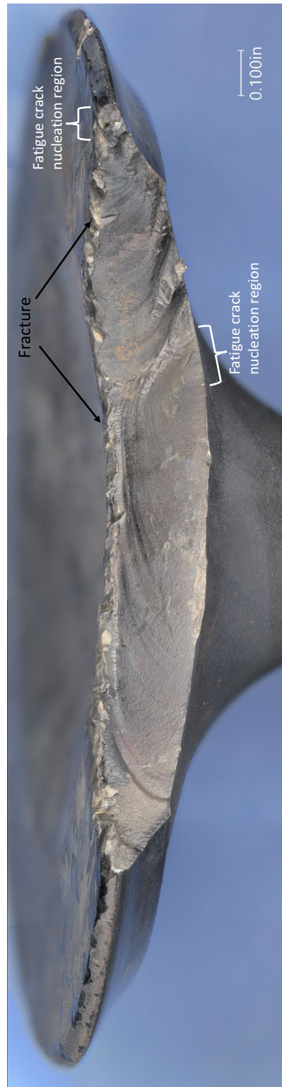
Figure 4 Overall digital microscope image of the number 1 intake valve fracture surfaces with the initiation or nucleation regions identified.
