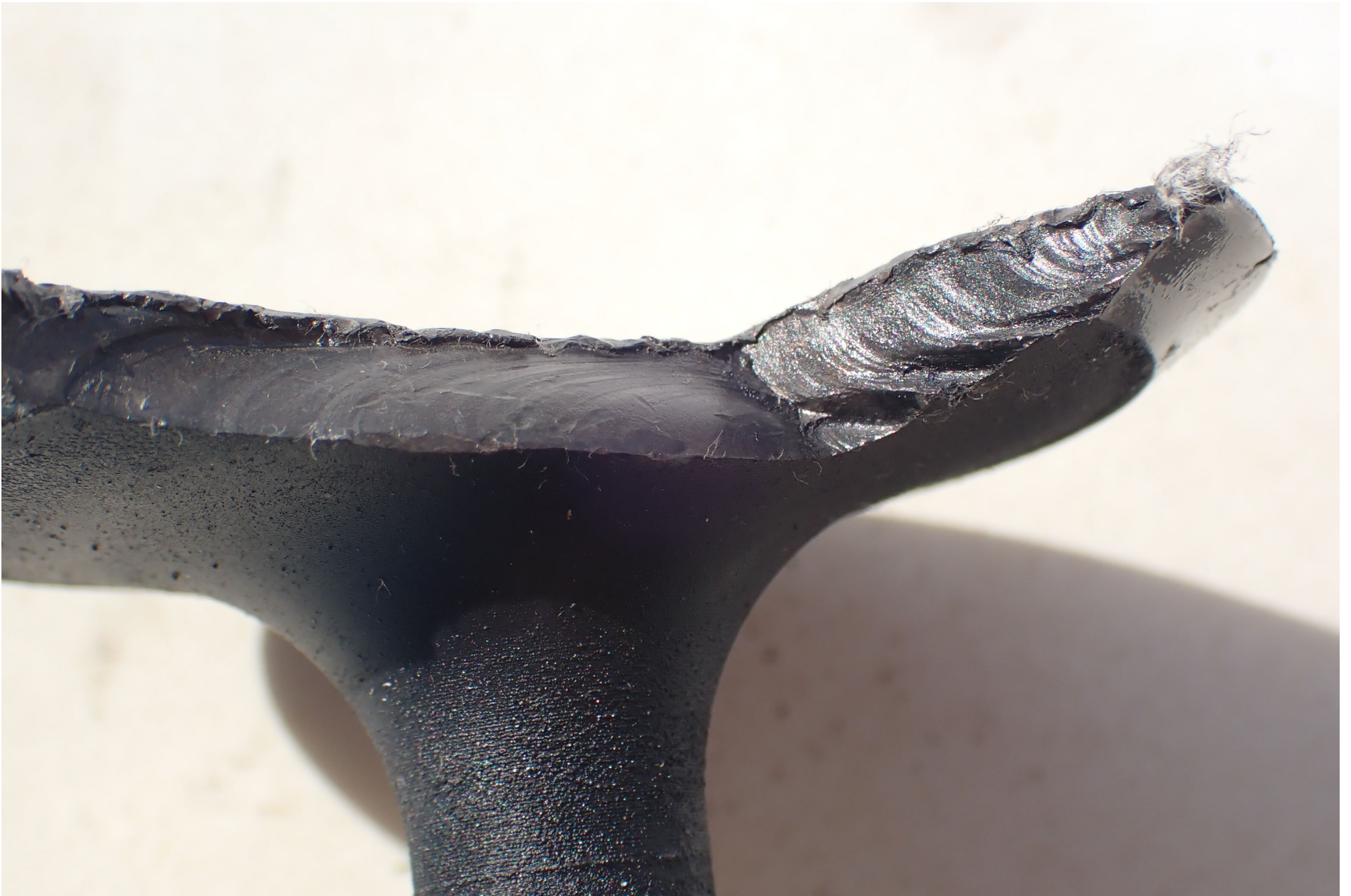
Photo 9 – Intake Valve Fracture Surface
