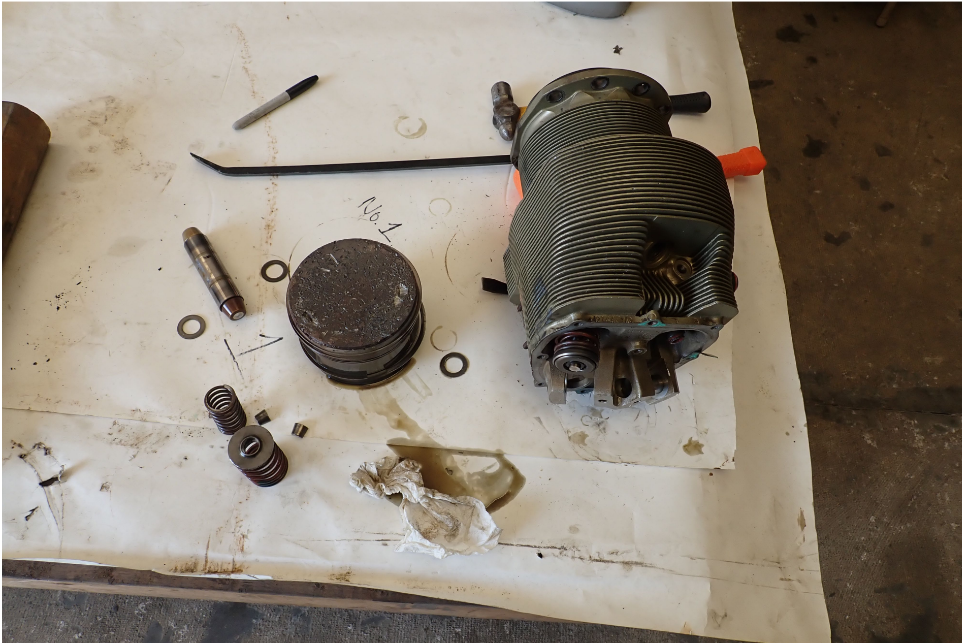
Photo 6 – No. 1 Cylinder Disassembled
