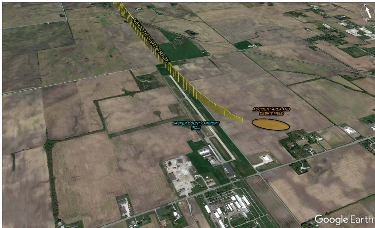
Figure 2. Final segment of accident flight track overlaid on satellite imagery (profile view).
