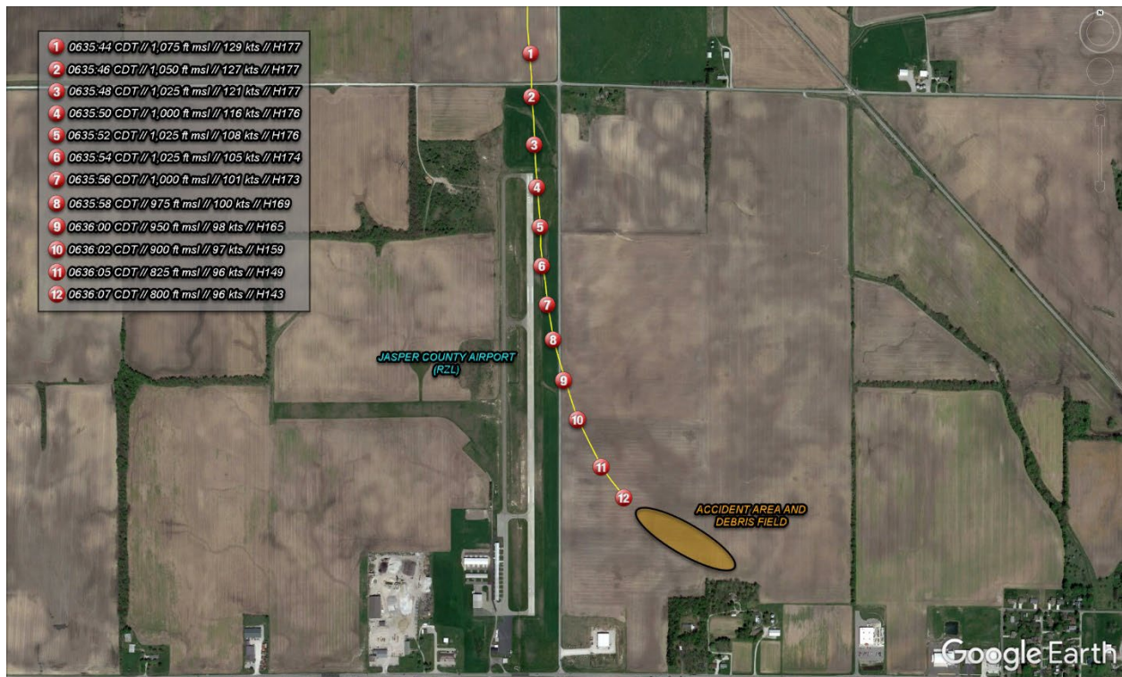
Figure 3. Final segment of accident flight track overlaid on satellite imagery - with time, altitude, ground speed, and heading information indicated.
