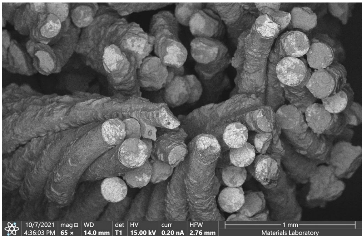
Figure 6 – Backscattered electron (BE) micrograph of a typical area of the fractured wires in Figure 4.
