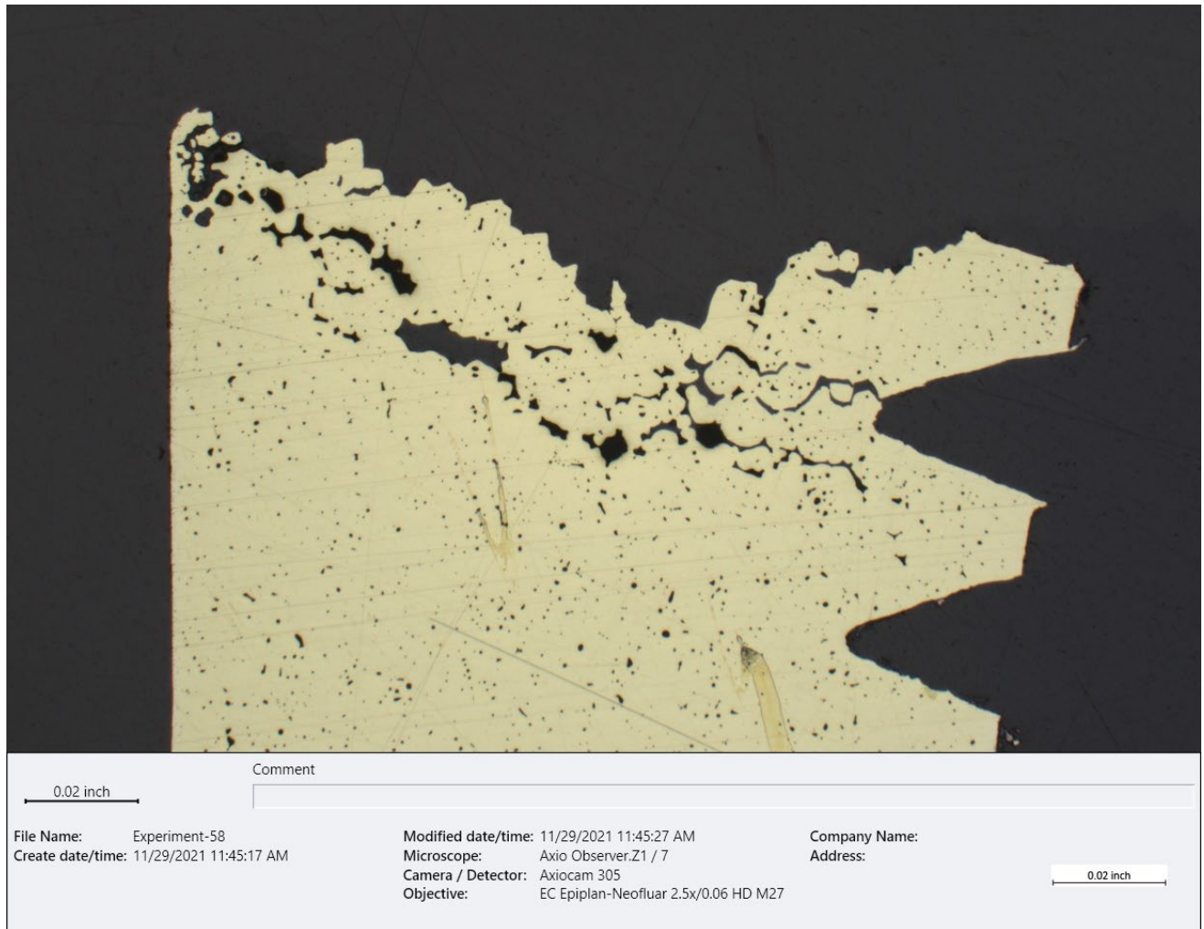
Figure 21 – Bright-field (BF) optical micrograph of a cross section of one side of the turnbuckle fracture surface, showing subsurface intergranular cracking (~25X, as-polished).
