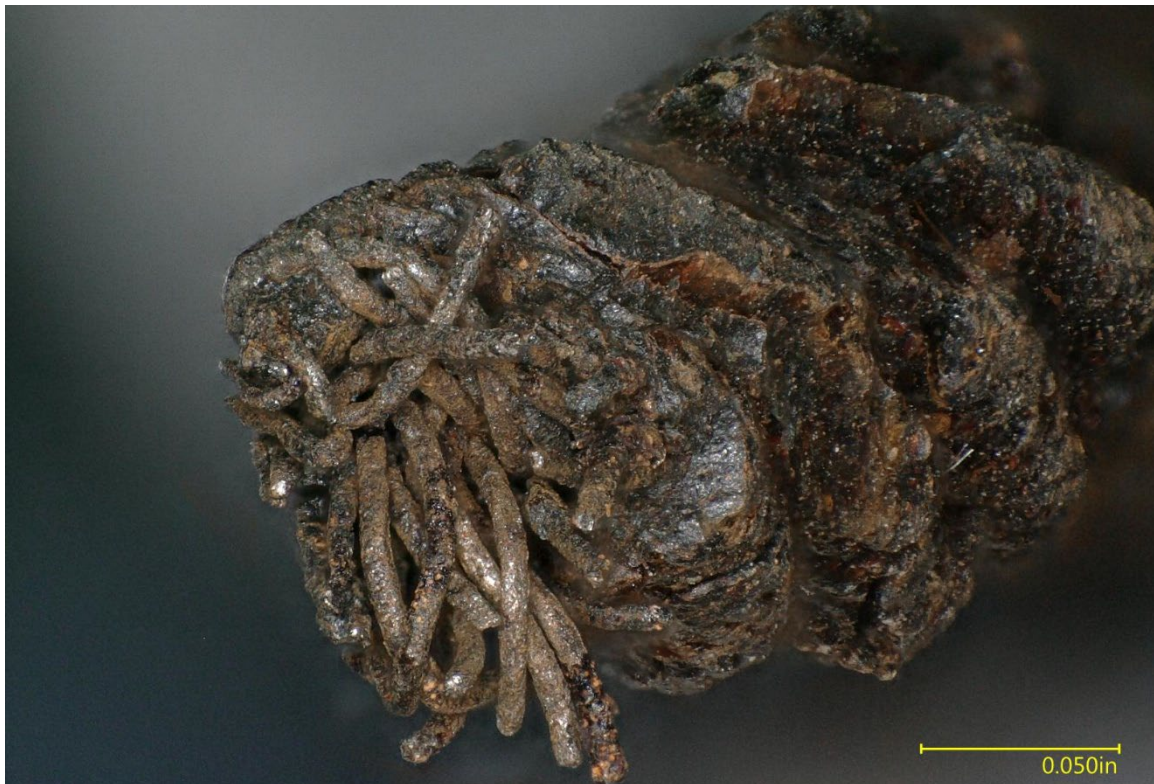
Figure 11 – Fracture surface of the middle remnant facing the short segment.
