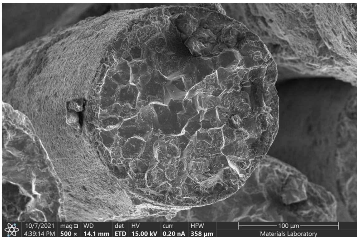
Figure 7 – SE micrograph of one of the fractured strands in Figure 5, showing intergranular fracture.
