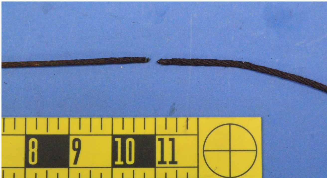
Figure 2 – Closer view of the cable fracture towards right in Figure 1.
