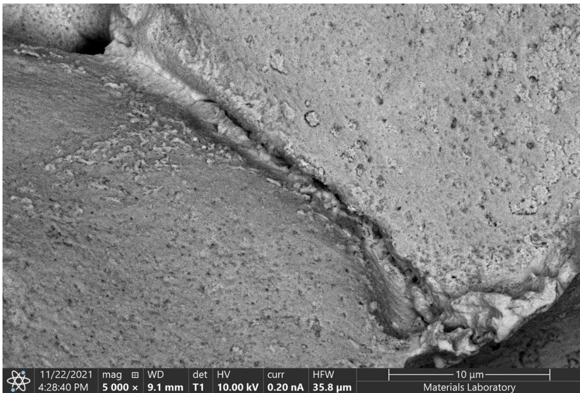
Figure 20 – BE micrograph of a triple point between facets, consistent with dissimilar materials.
