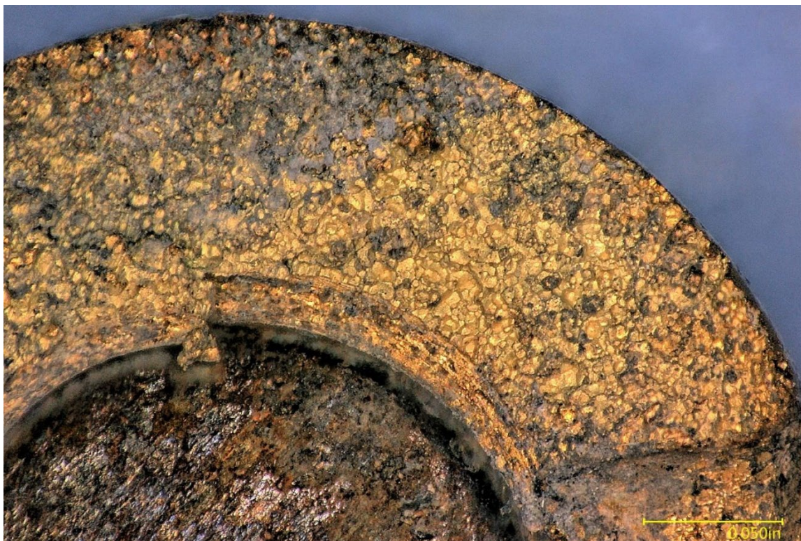
Figure 17 – View of a quadrant of the turnbuckle fracture, showing a faceted surface morphology.
