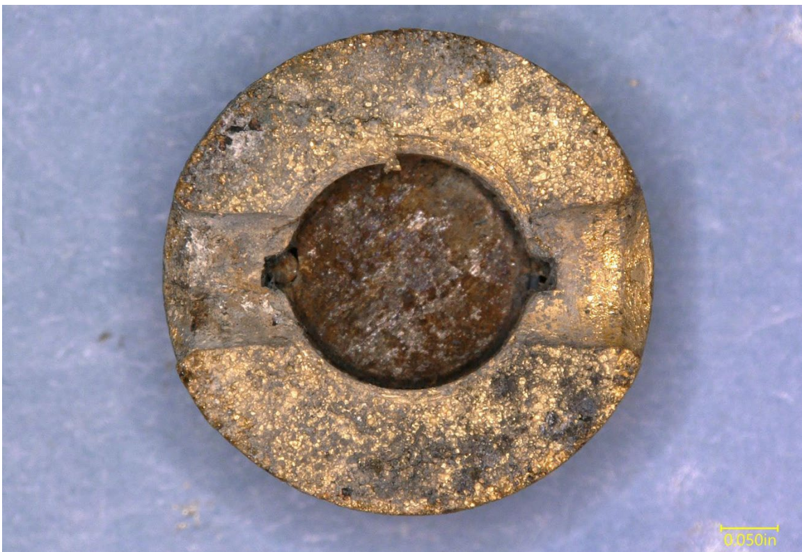
Figure 16 – View of the fracture surface of the cable turnbuckle.
