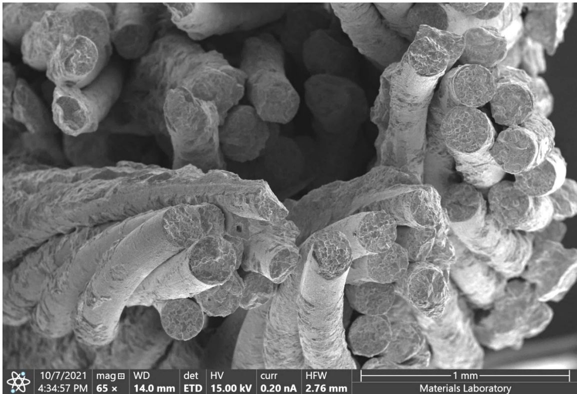
Figure 5 – Secondary electron (SE) micrograph of a typical area of the fractured wires in Figure 4.
