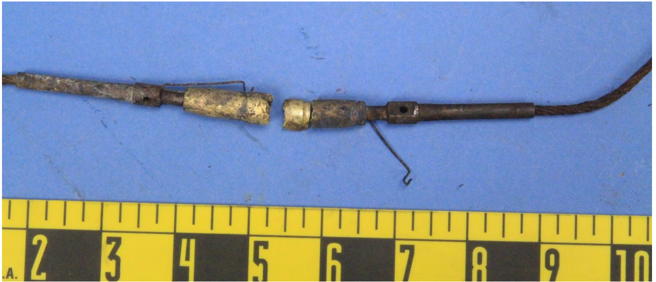
Figure 15 – View of the fractured turnbuckle (after sectioning and cleaning).
