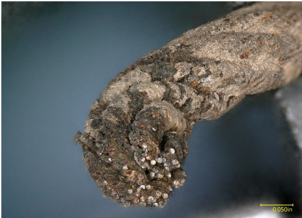
Figure 4 – Fracture surface of the cable from Figure 3 (long remnant).
