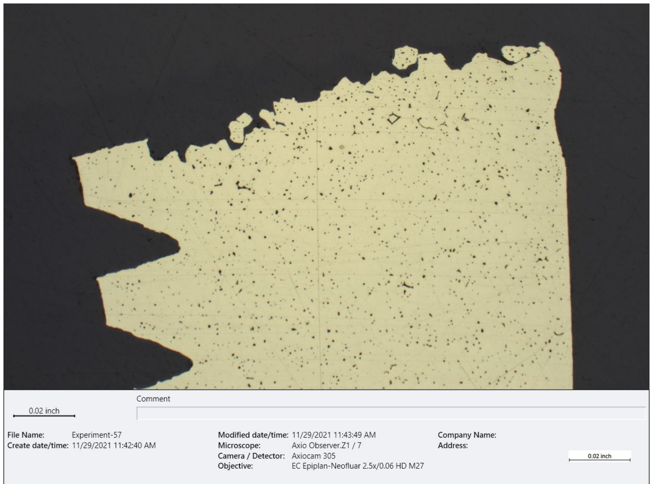
Figure 24 – BF optical micrograph of the opposite turnbuckle fracture surface (~25X, as-polished).
