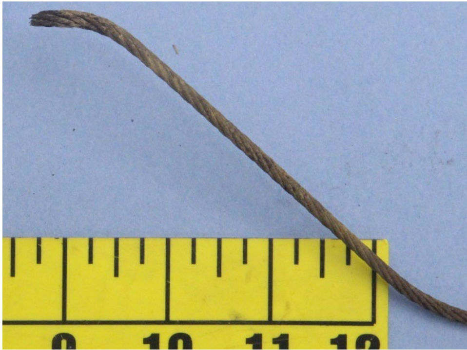
Figure 3 – Closer view of the fracture towards the longer fragment side (left in Figure 1).
