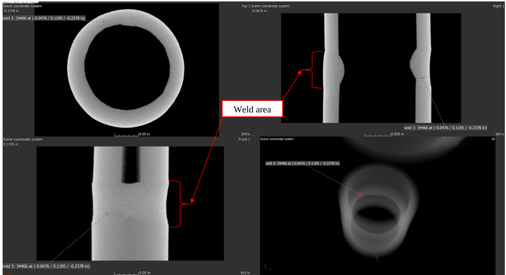
Figure 10 Engine pressure measurement tube weld – void 3 overview
