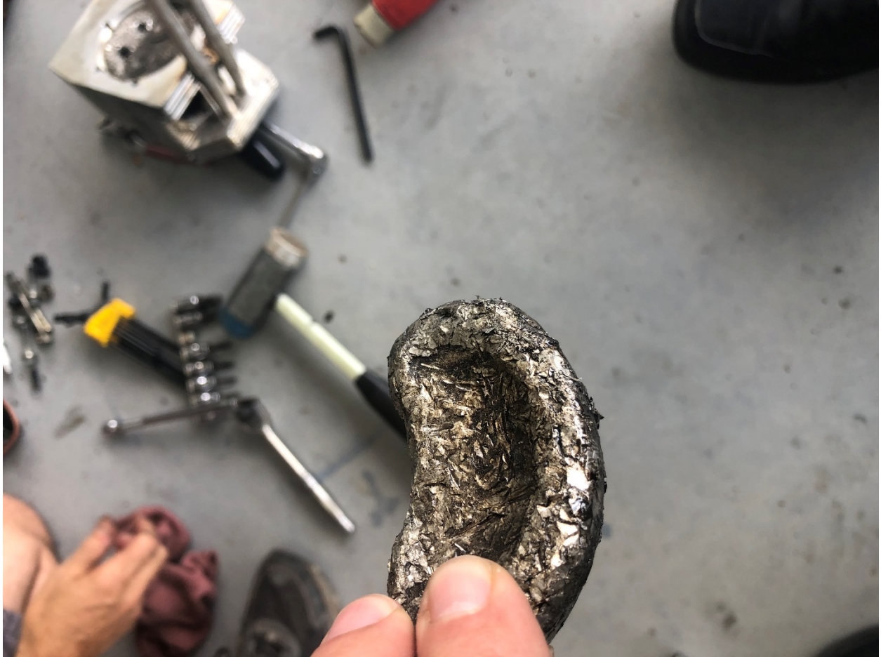
Photo 3: Close-up View of Number One Piston
