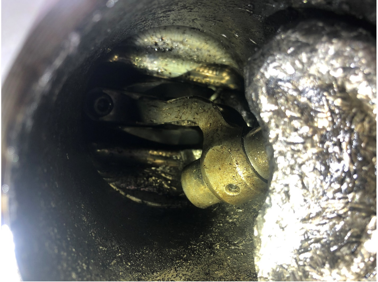
Photo 2: Remains of Number One Piston
