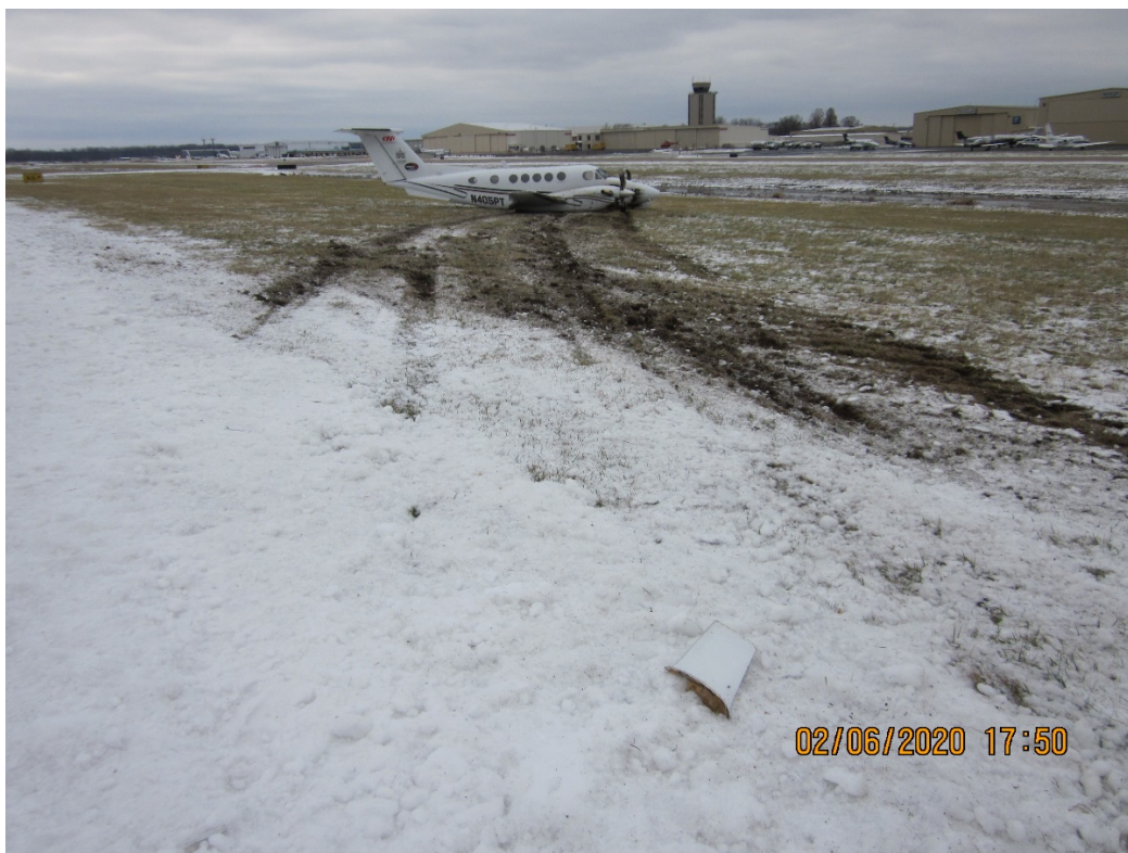
Figure 3: Skid Marks in Grass and Airplane Where it Came to Rest (Courtesy of FAA)
