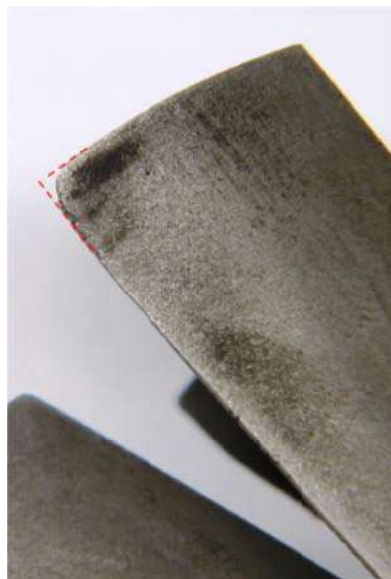
Figure 3: Representative leading edge tip erosion found on the stage 1 compressor blades. The red dashed line shows the approximate original profile of the leading edge tip.
