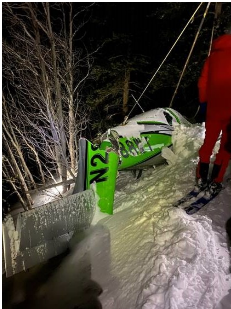
Photo 5 - Supplied close-up photo of the separated empennage with the fuselage in the background.
