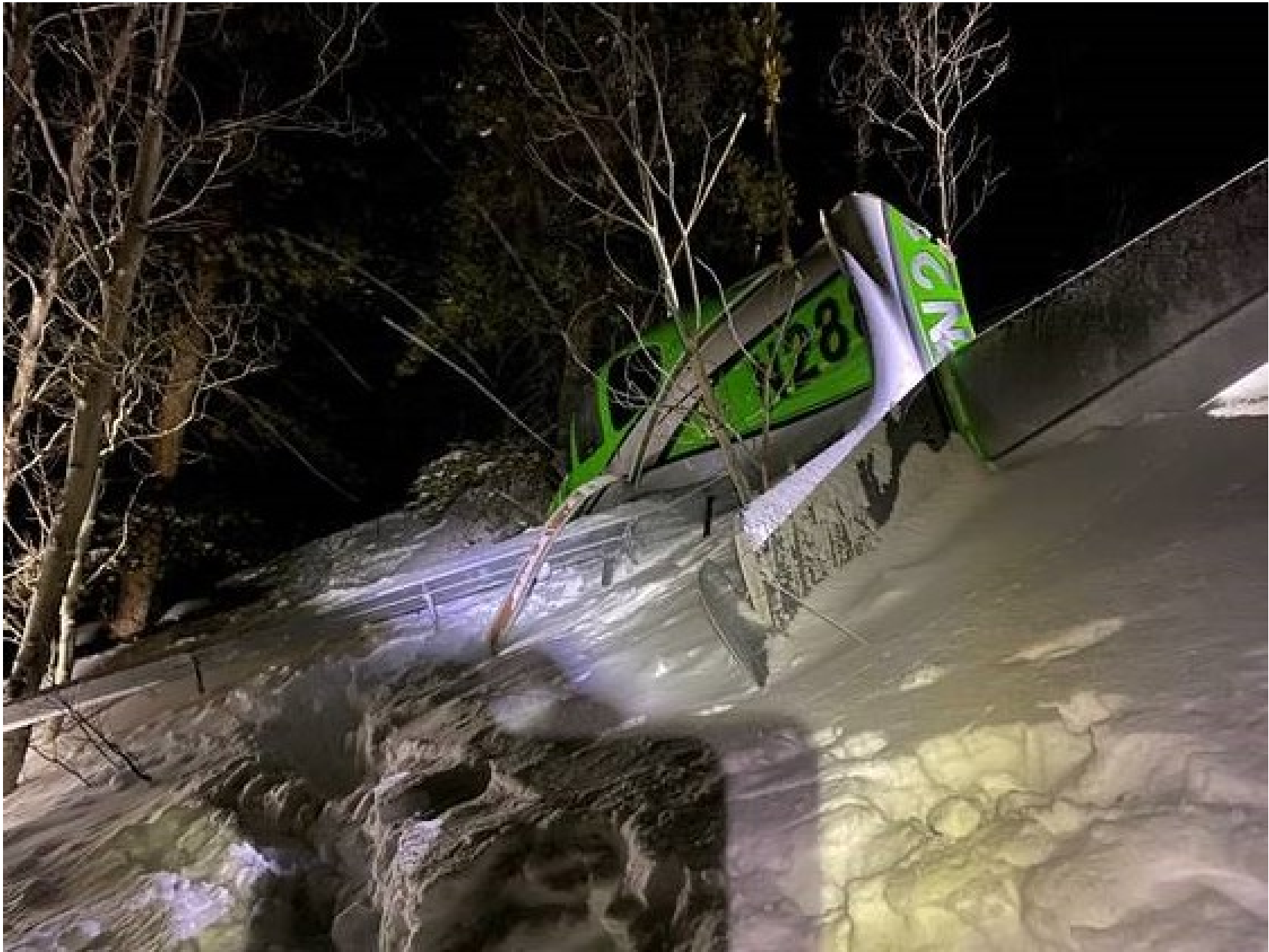
Photo 4 - Supplied close-up photo of the separated empennage with the fuselage in the background.
