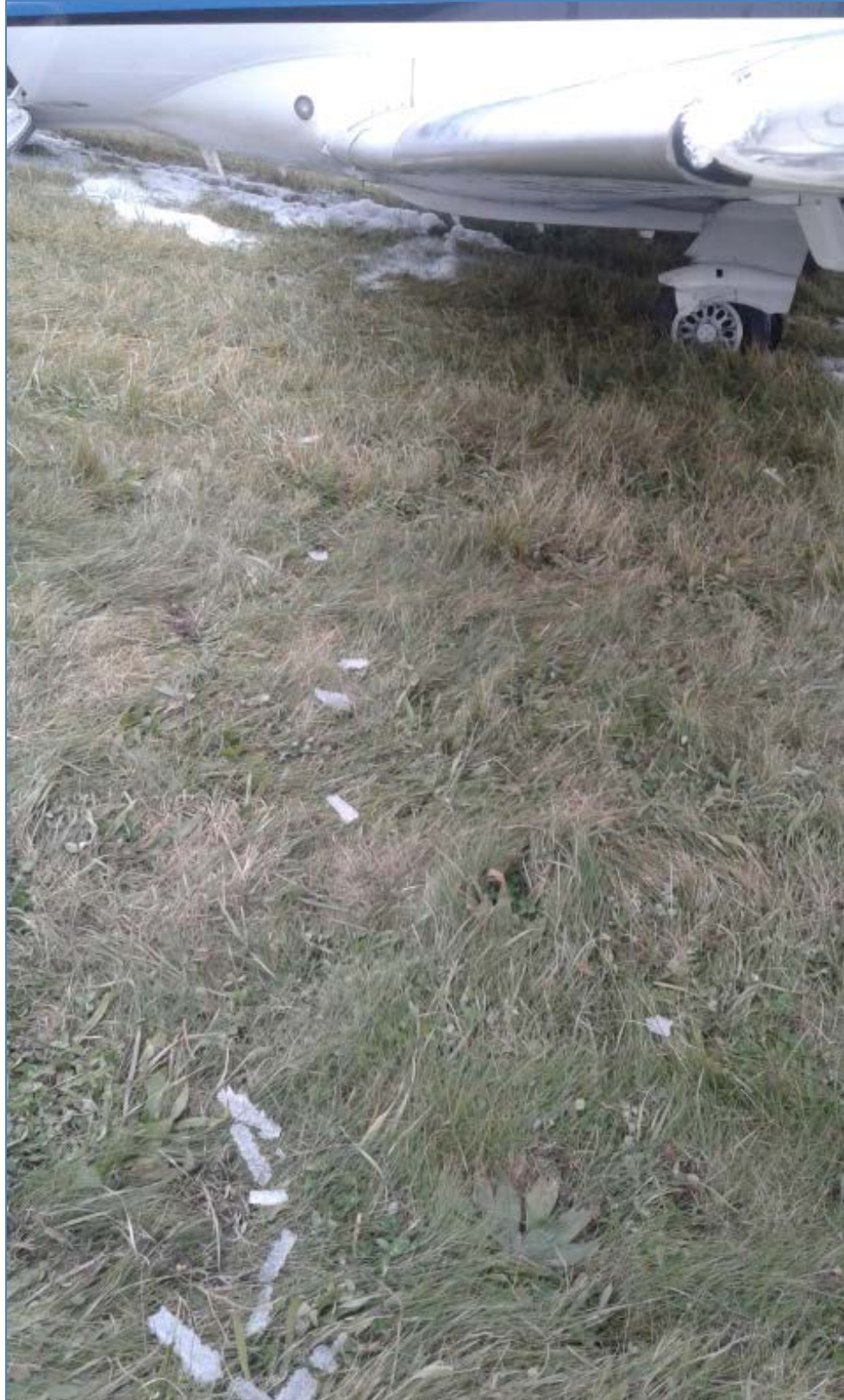
Figure 29 - Pieces of ice that fell from left wing between TKS seams
