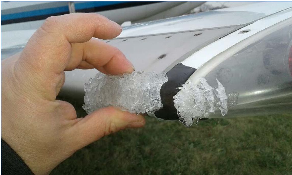
Figure 28 - Left wing with ice on tip and between TKS seems
