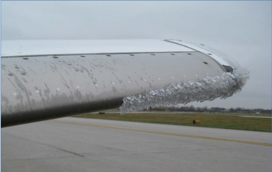
Figure 27 - Left wing tip with ice
