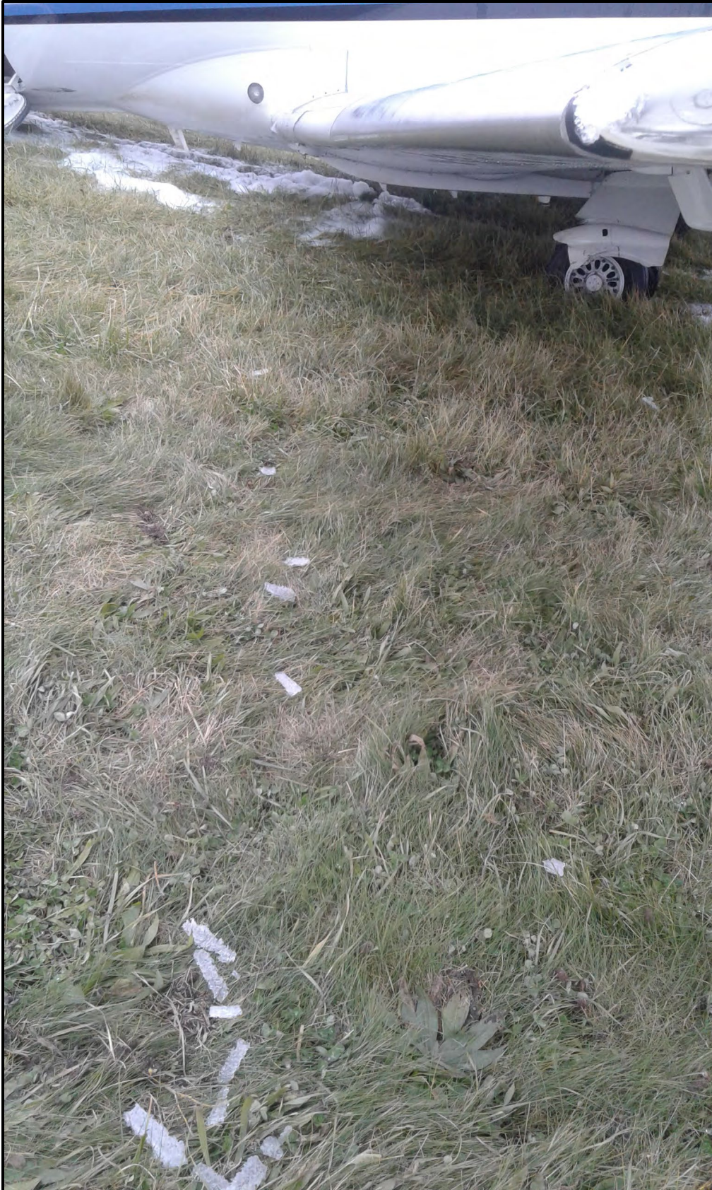
Figure 12: Photo of Ice on Ground after the Accident (source: FAA)
