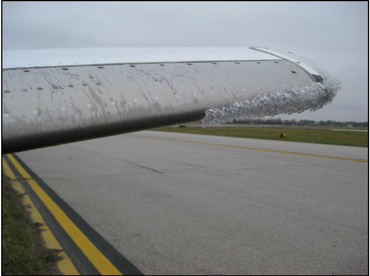
Figure 11: Photo of Ice on Left Wingtip after the Accident (source: FAA)
