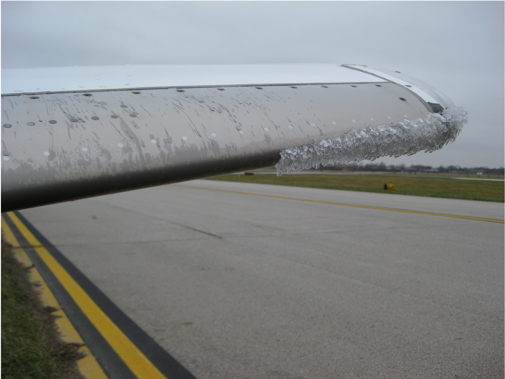
Photo 5 - Supplied close-up view of ice on the left outboard wing.
