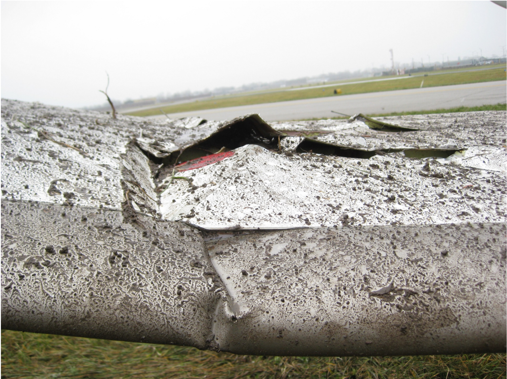
Photo 4 - Supplied close-up view of damage to the right outboard wing.
