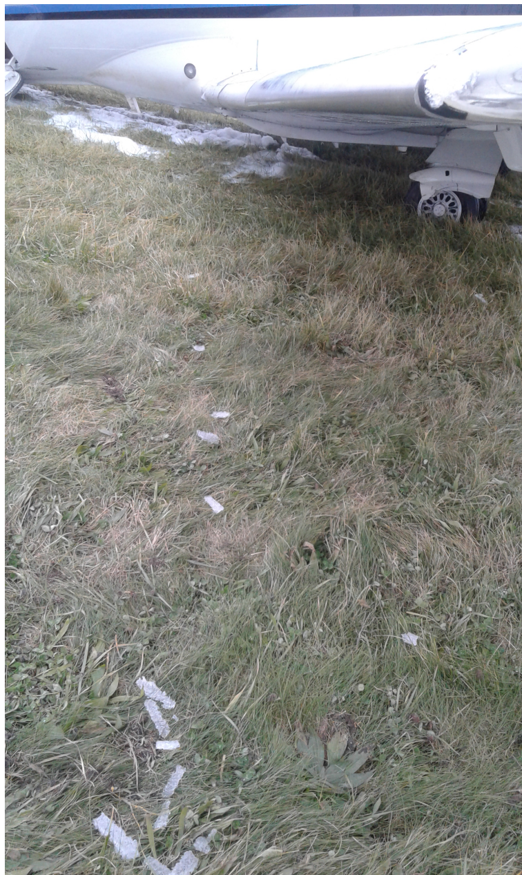
Photo 7 - Supplied view of ice on the ground under the leading edge of a wing.
