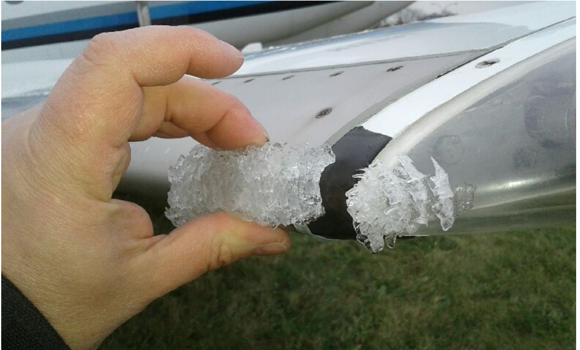
Photo 8 - Supplied close-up view of ice on the leading edge of the outboard left wing.
