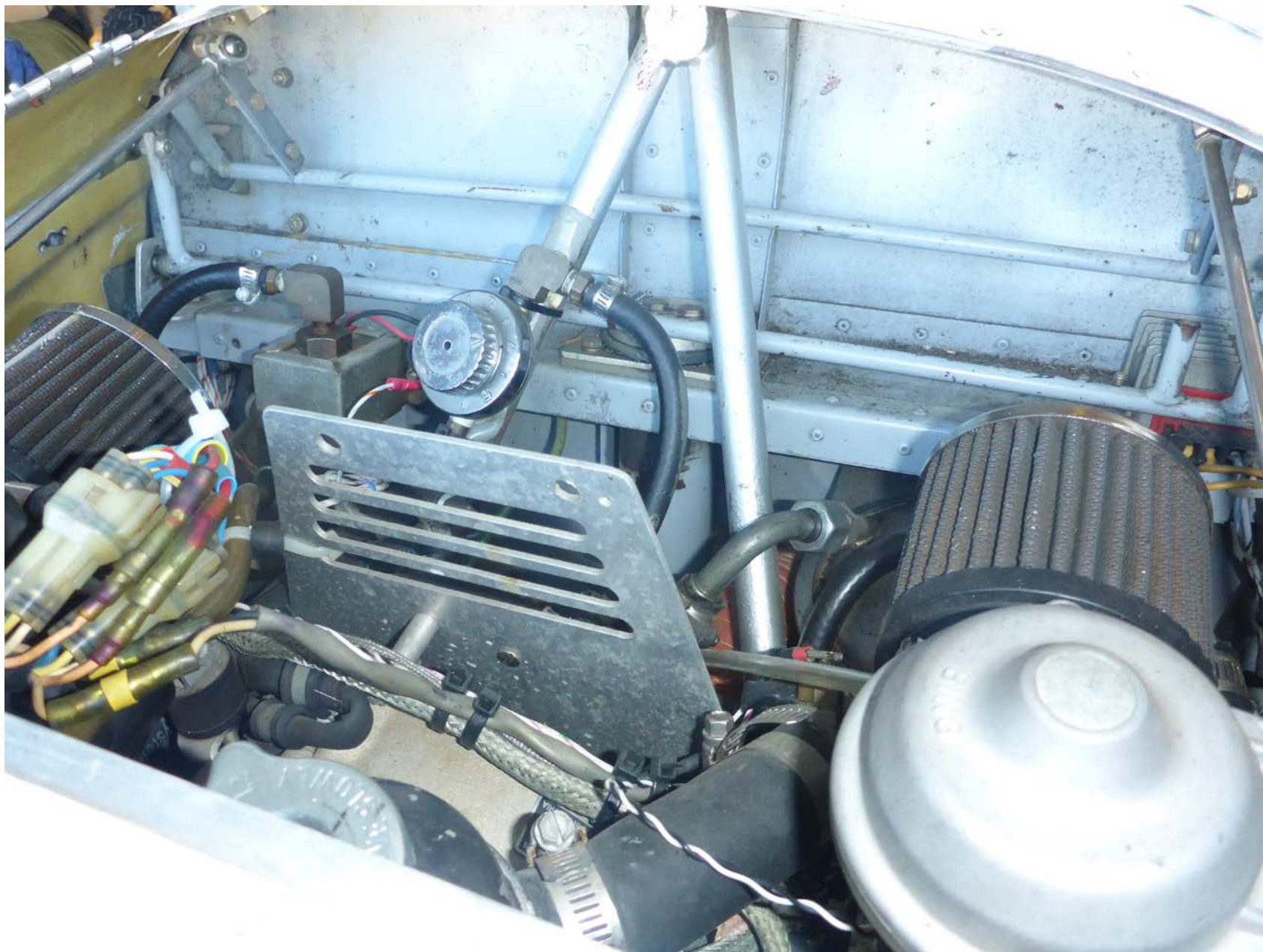
Photo 3 – Air Filters (Rotech Photo)
