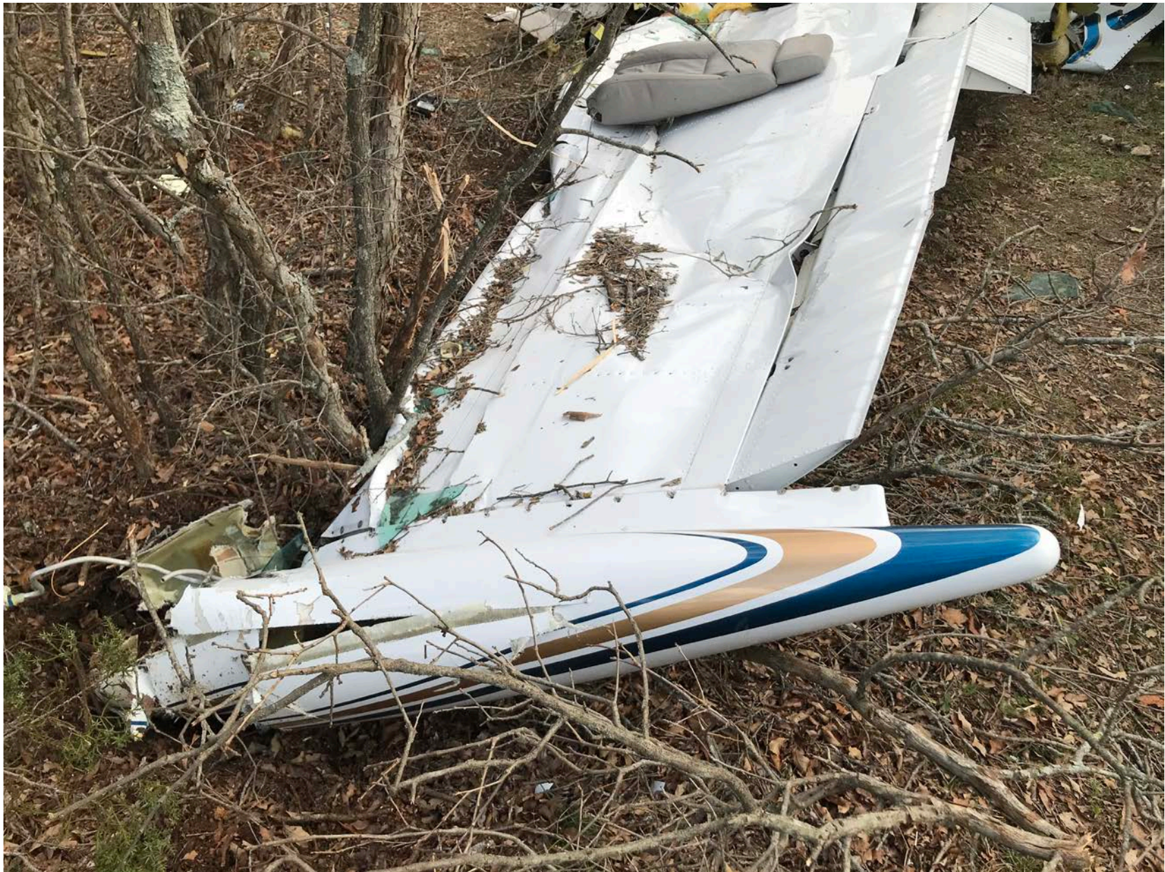
Photo 3 – Left wing damage
