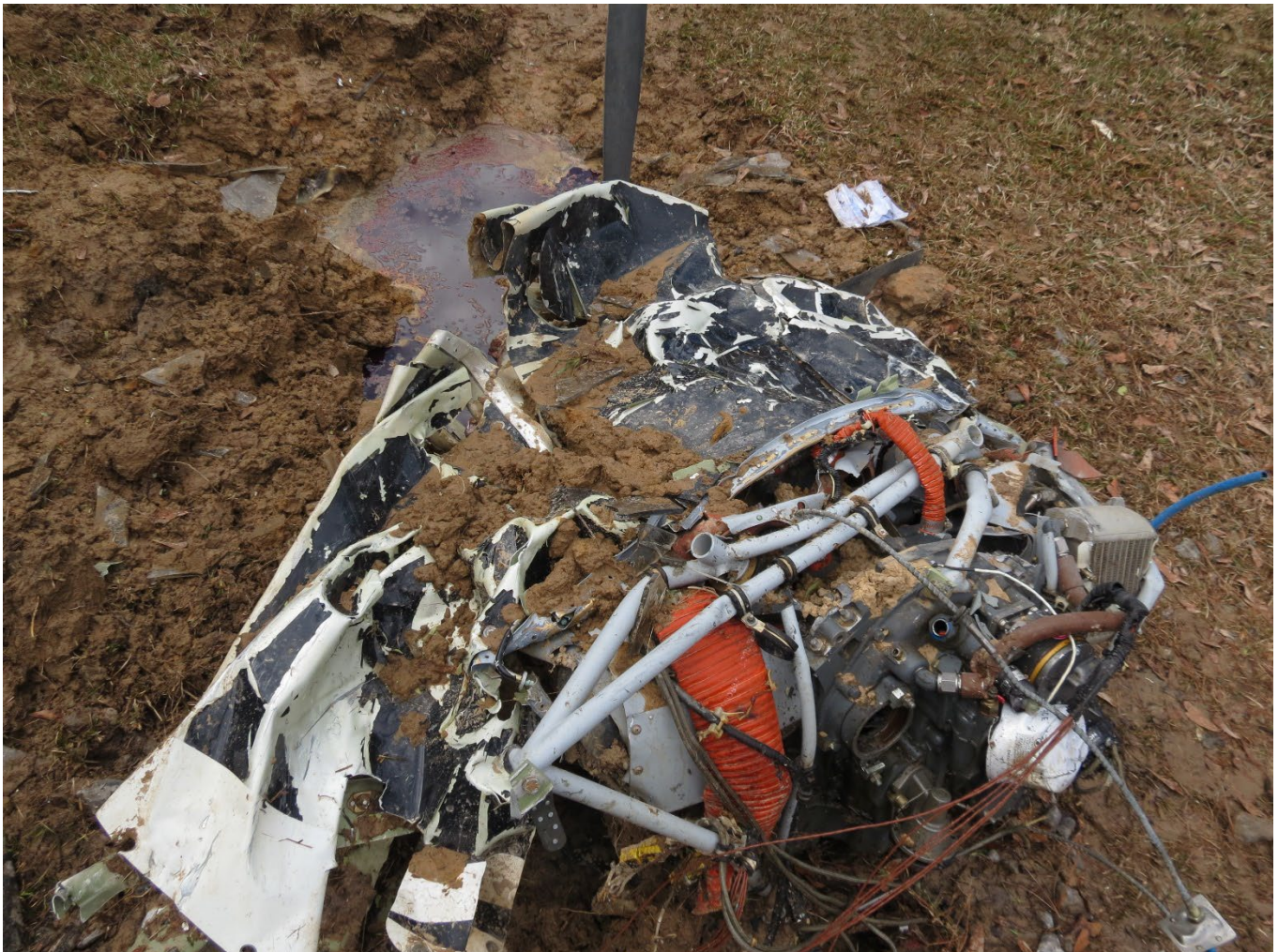
Photo1: Engine at Accident Site
