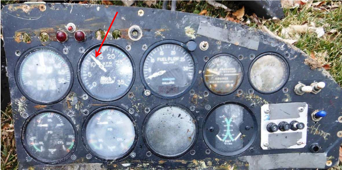
Photo #1 – Engine instrument panel with both RPM indicators at approximately 1200
