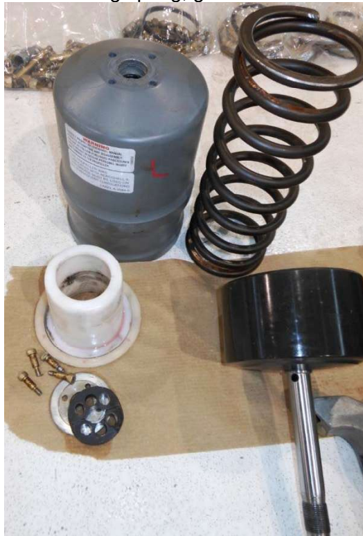
Photo #12 – Left feathering spring, guides and start lock components
