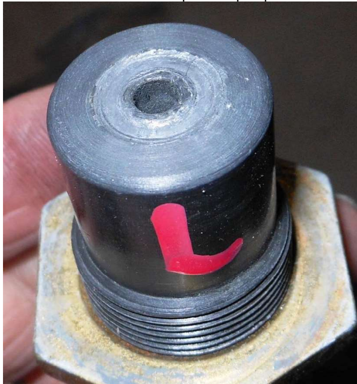
Photo #10 – Left low pitch stop impression
