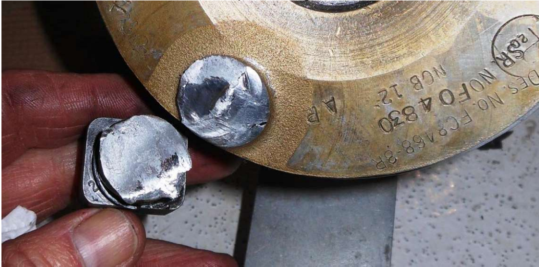
Photo #17 – L3 pitch change knob fracture
