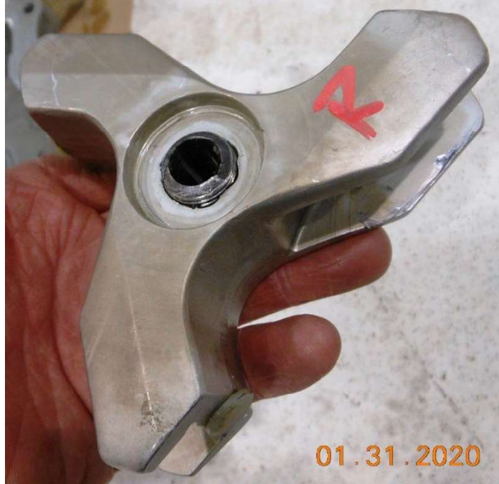
Photo #28 – Right fork with pitch change rod segment in threads
