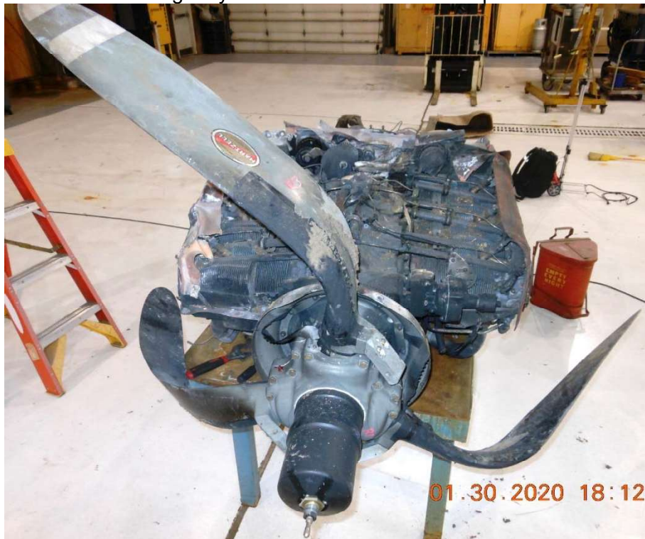
Photo #26 – Right hydraulic unit condition after spinner removal
