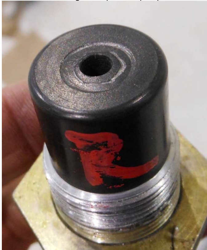
Photo #30 – Right low pitch stop impact mark
