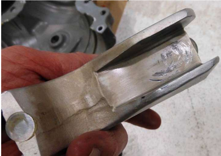
Photo #29 – Right fork impact marks in slot
