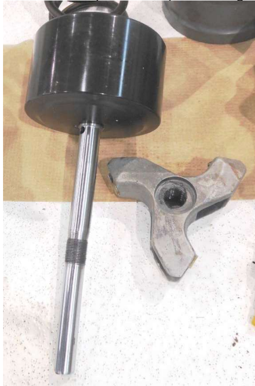
Photo #11 – Left piston and pitch change rod
