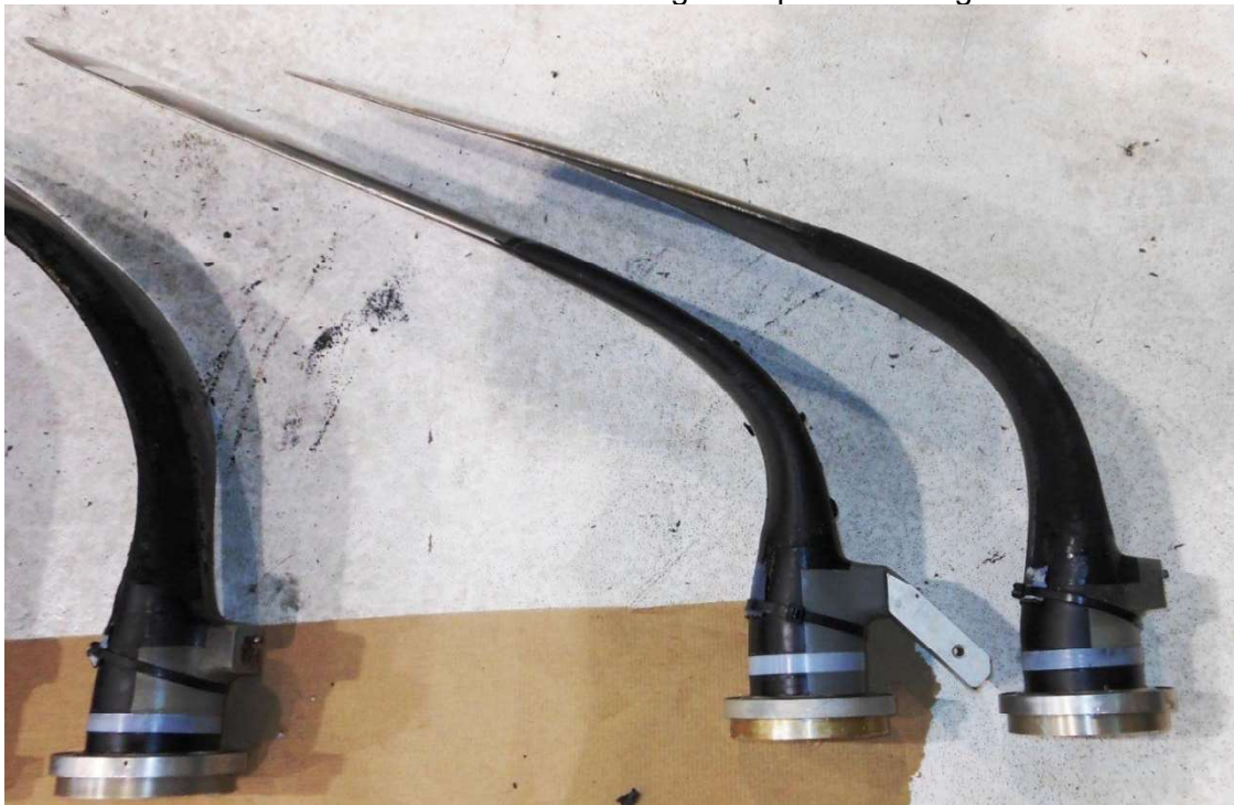
Photo #6 – L3 and R3 blade damage comparison – edge view
