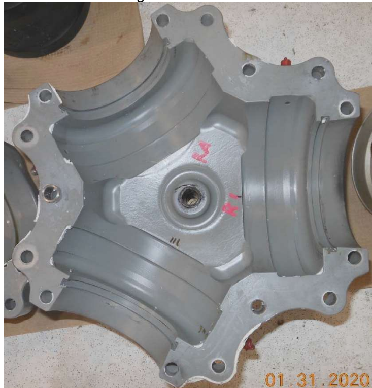
Photo #32 – Right aft hub half internal surface
