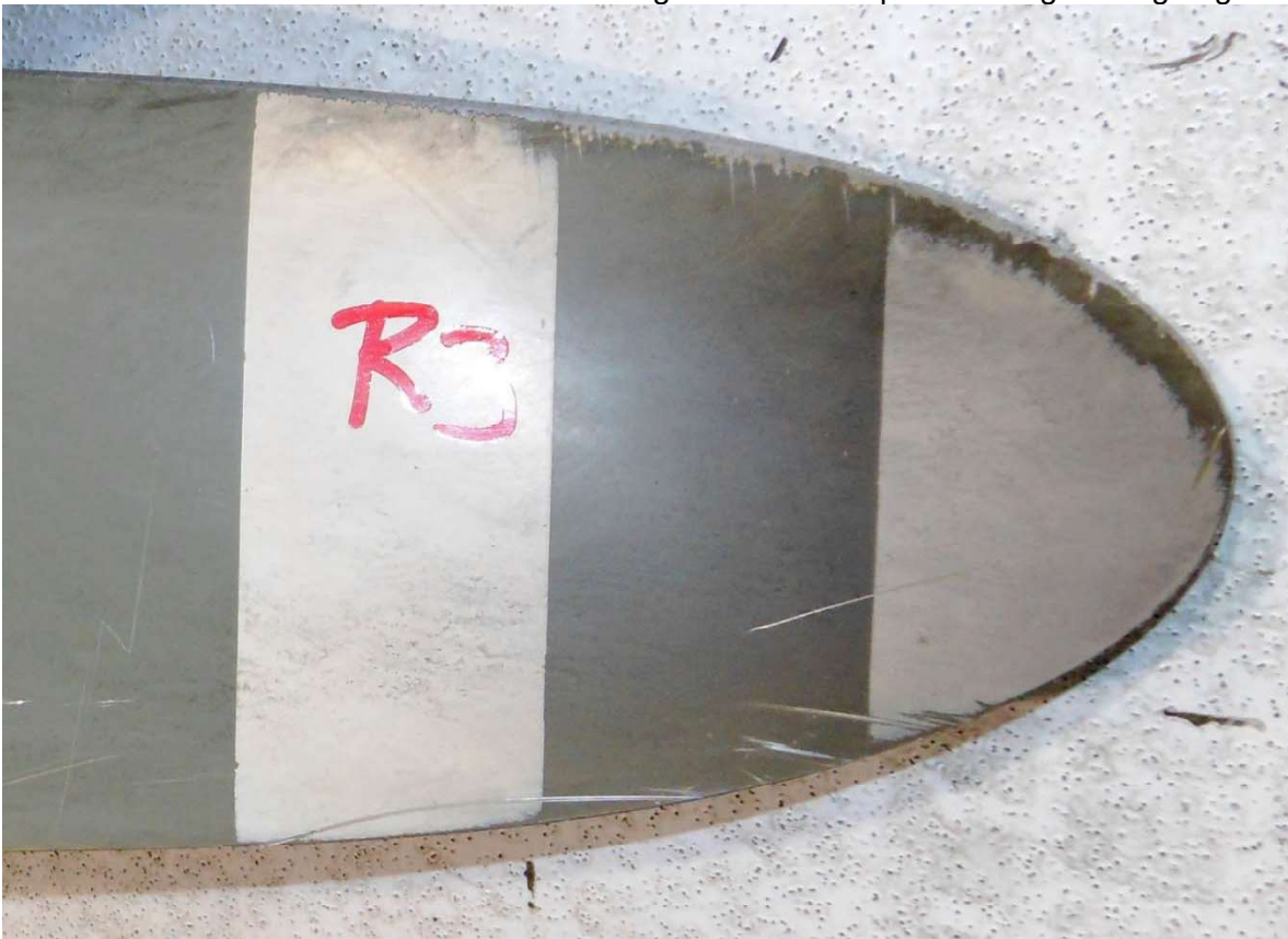
Photo #38 – R3 chordwise/rotational scoring camber side tip area along leading edge
