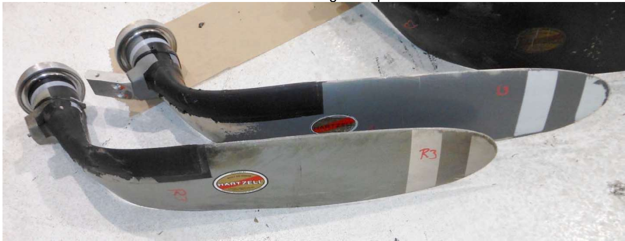
Photo #5 – L3 and R3 blade damage comparison – camber side
