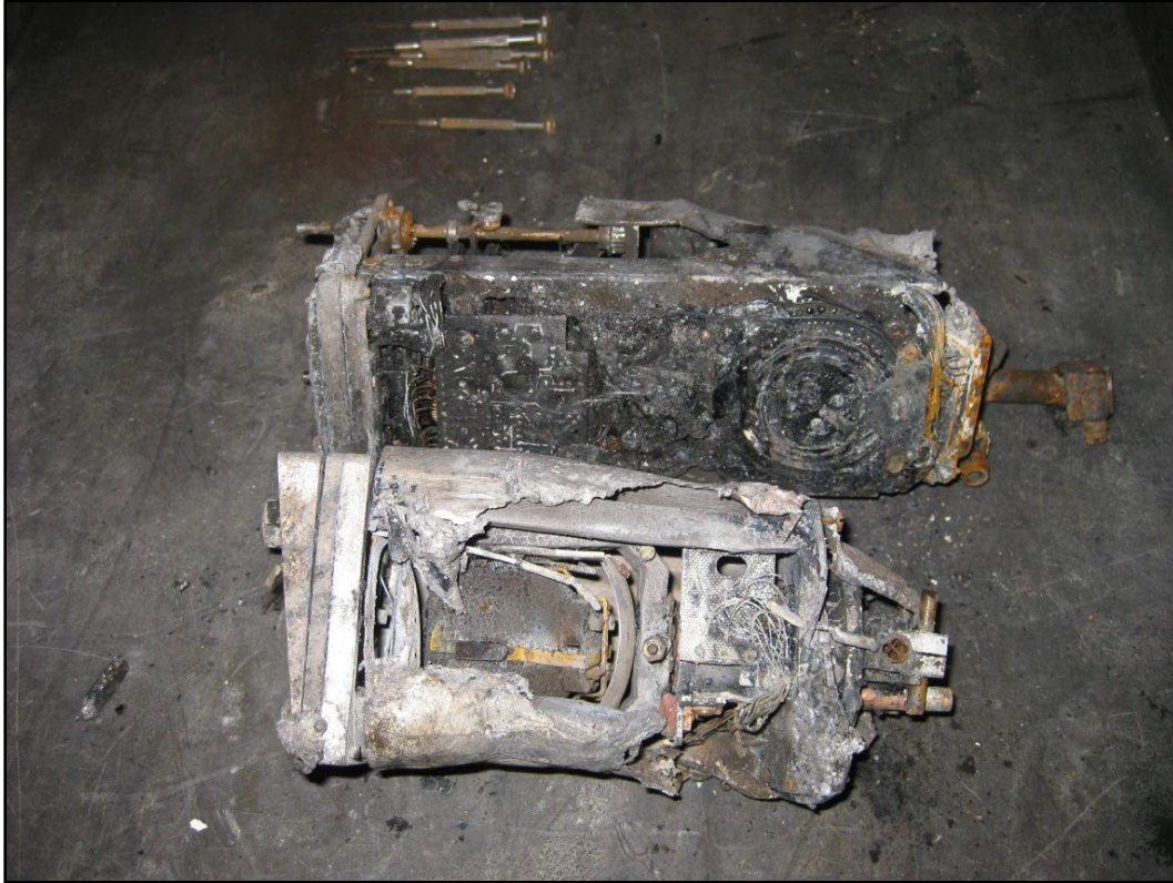
Figure 11 - Attitude Indicator (foreground) and HSI (background)
