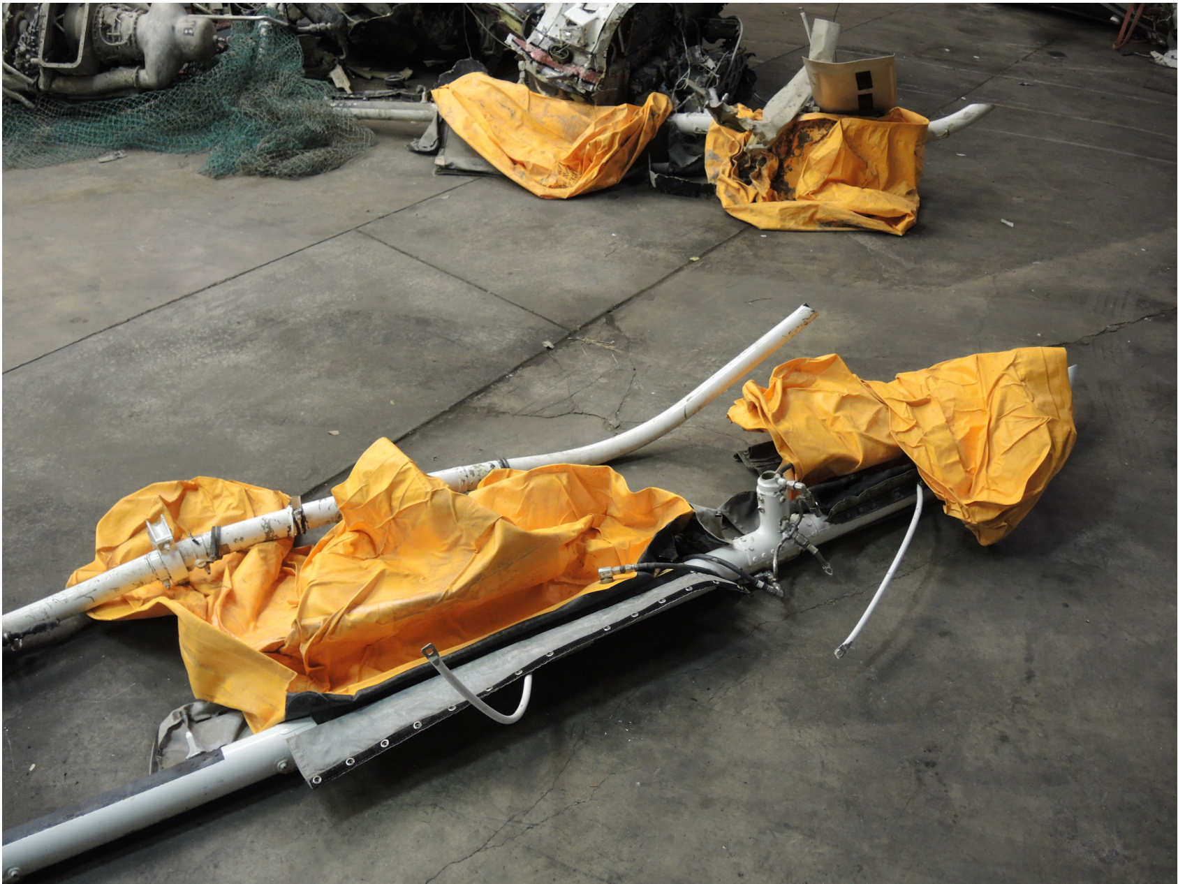
Photo 4 – Parts of the emergency flotation system
