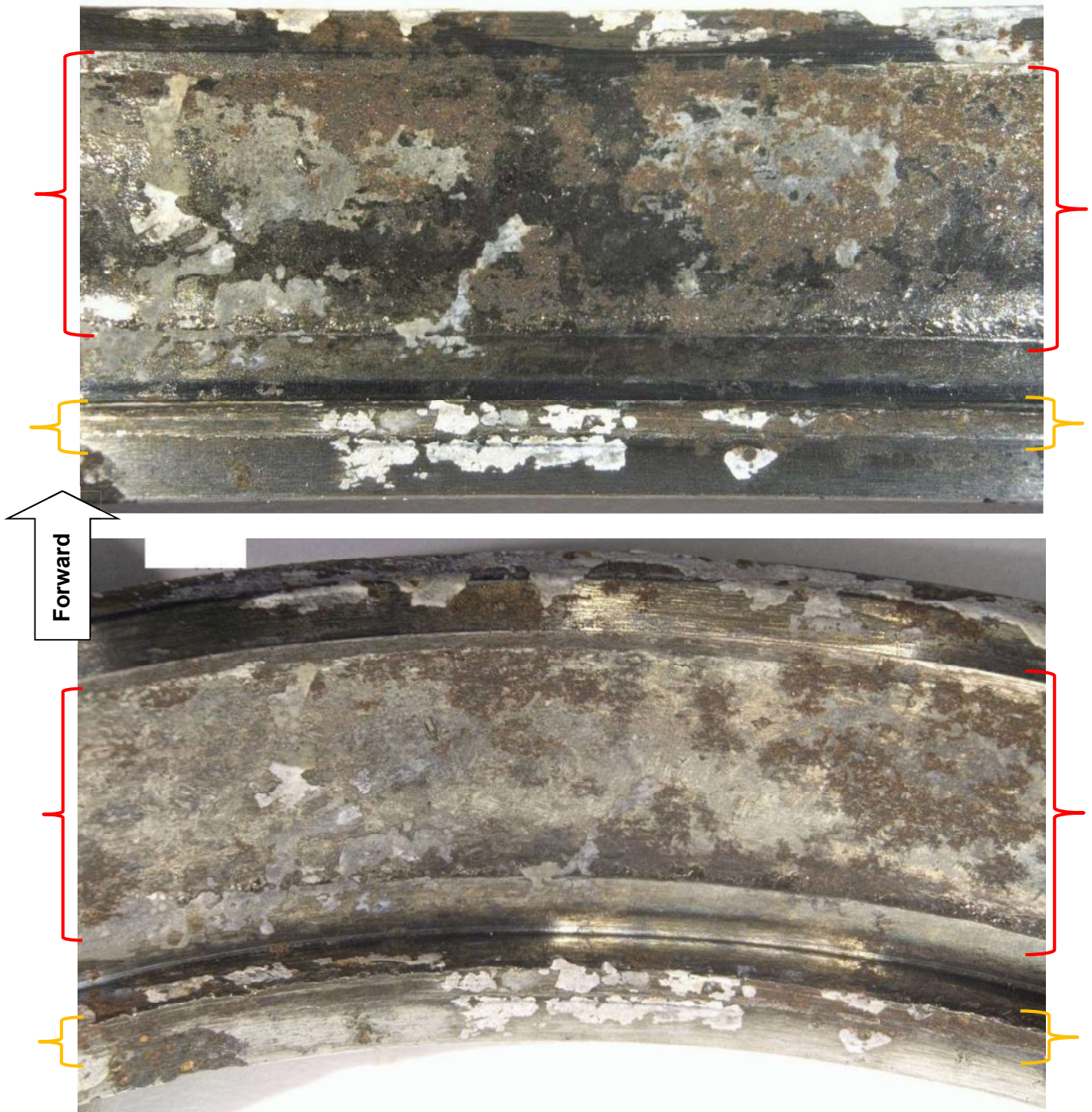
Figure 33. Detailed inboard looking outboard and oblique views of the No. 4 bearing outer ring raceway. Red braces mark the location of material removal at the roller path, and the orange braces mark rub damage on the aft shoulder corner.
