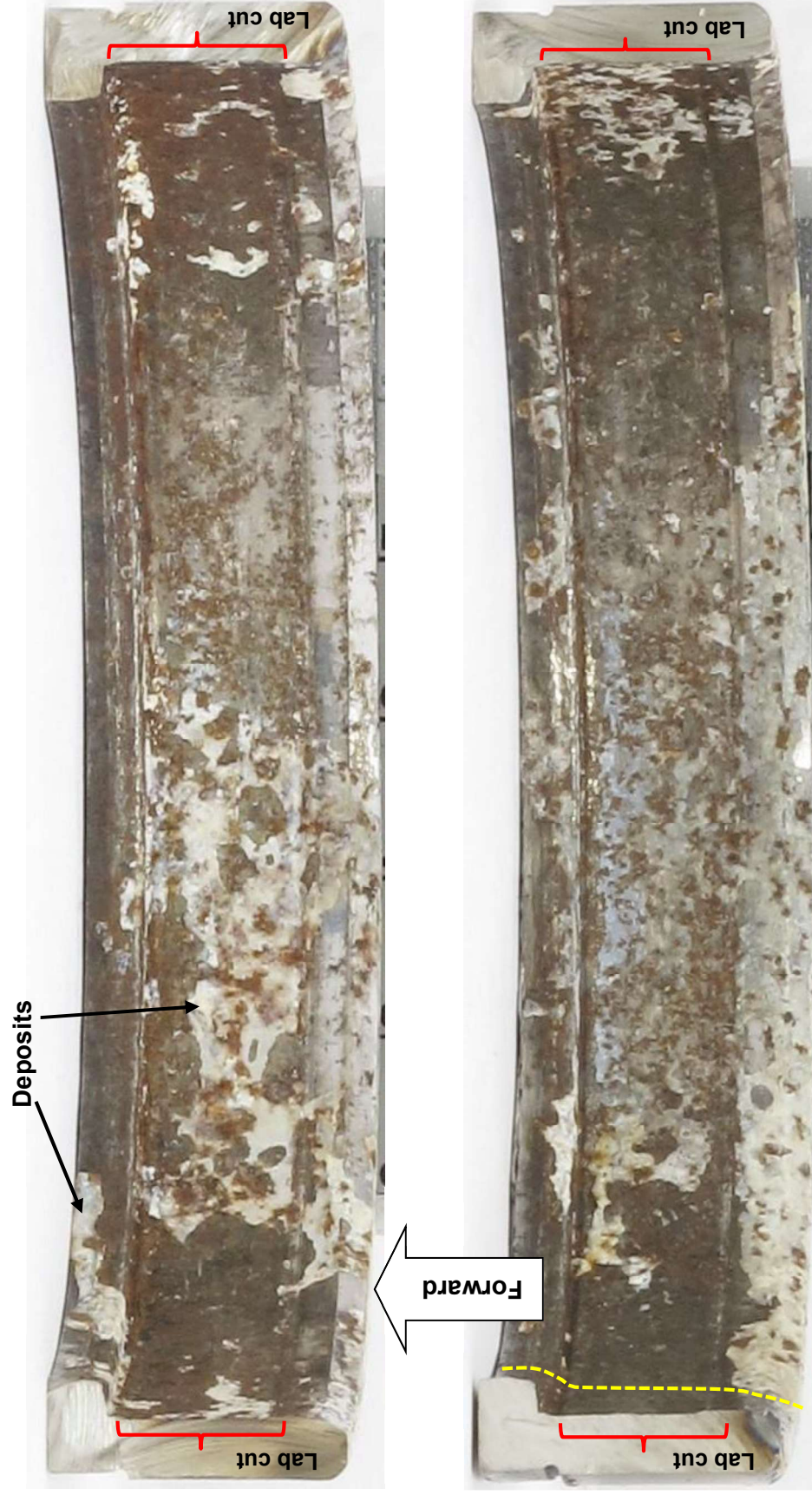
Figure 26. Two views of the No. 3 bearing outer ring, after it was sectioned and cleaned, showing the condition of the outer raceway surface. Red braces mark the location of material removal at the roller path, and the yellow dashed line marks the plane of metallographic evaluation (see Figure 29).
