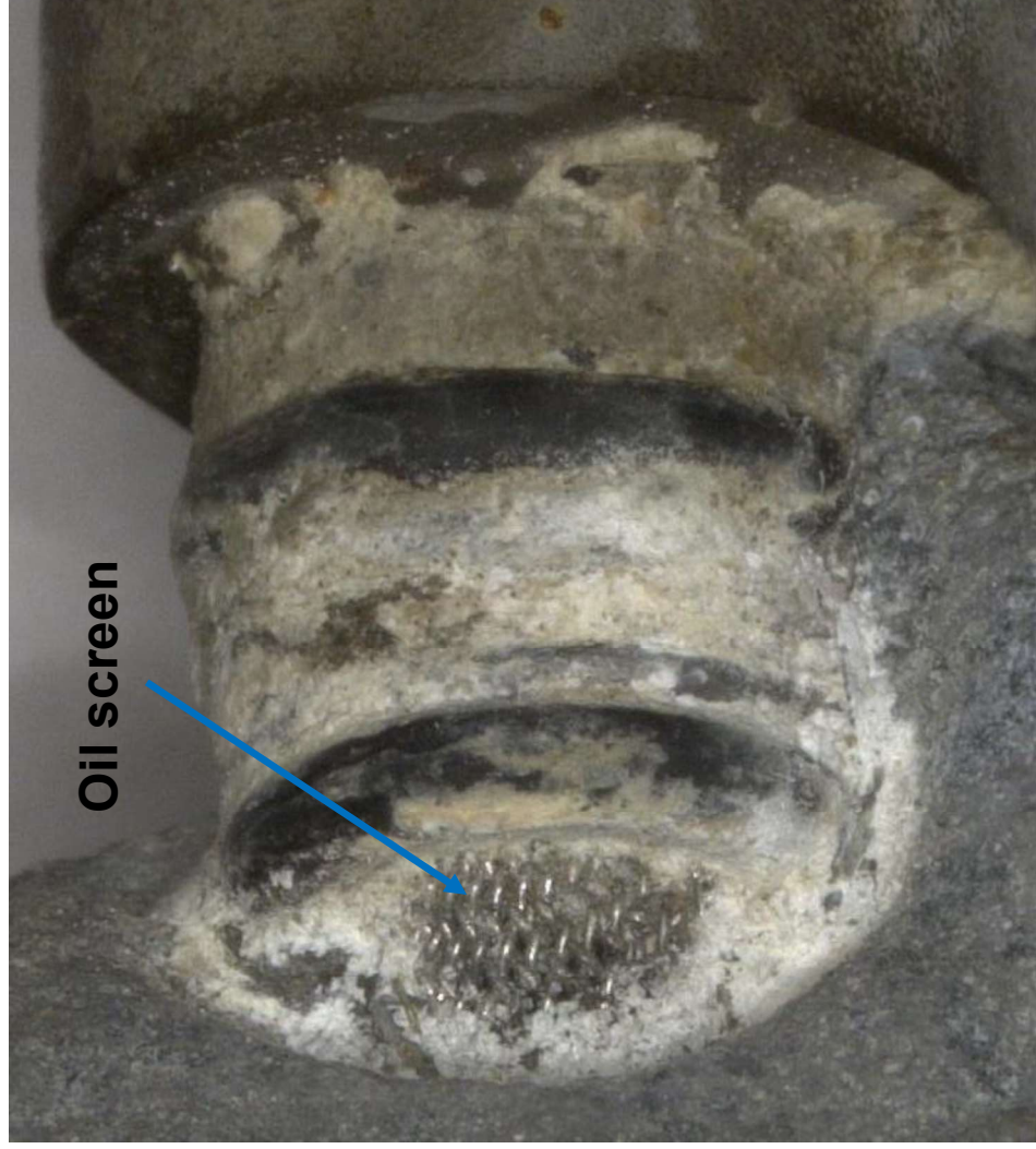
Figure 59. Detailed views of the oil screen and a blocked passage of the gearbox housing (see locations J and K in the previous figure, respectively).
