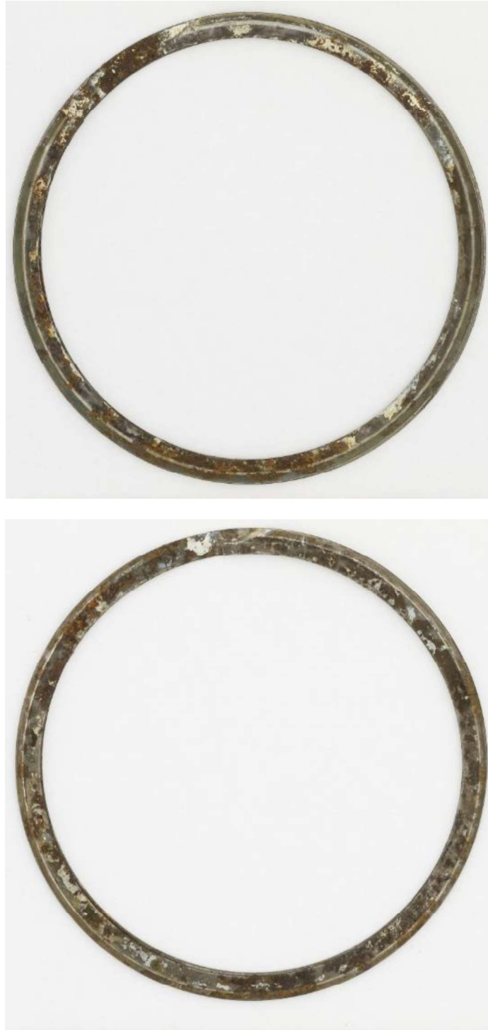
Figure 74. General condition of the forward (top) and aft (bottom) sides of the No. 4 bearing retaining ring.
