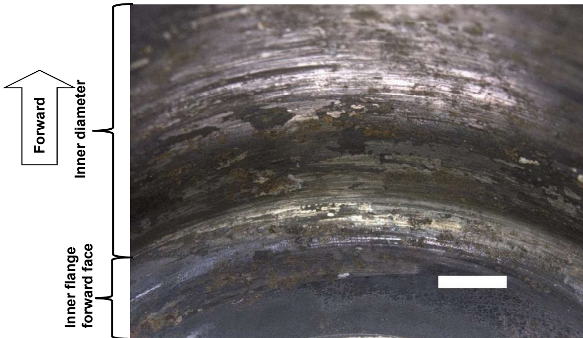
Figure 9. Detailed view of the inner diameter and inner flange forward face, which exhibited circumferential rub.
