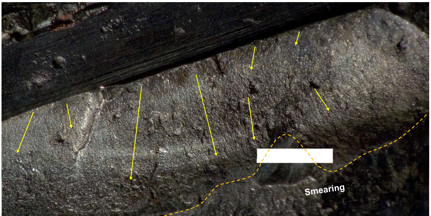
Figure 12. Detailed views of fracture surfaces at gear tooth number 2 after cleaning. The yellow arrows mark the direction of fatigue progression, and the orange dotted line marks the transition from fatigue to smearing damage.
