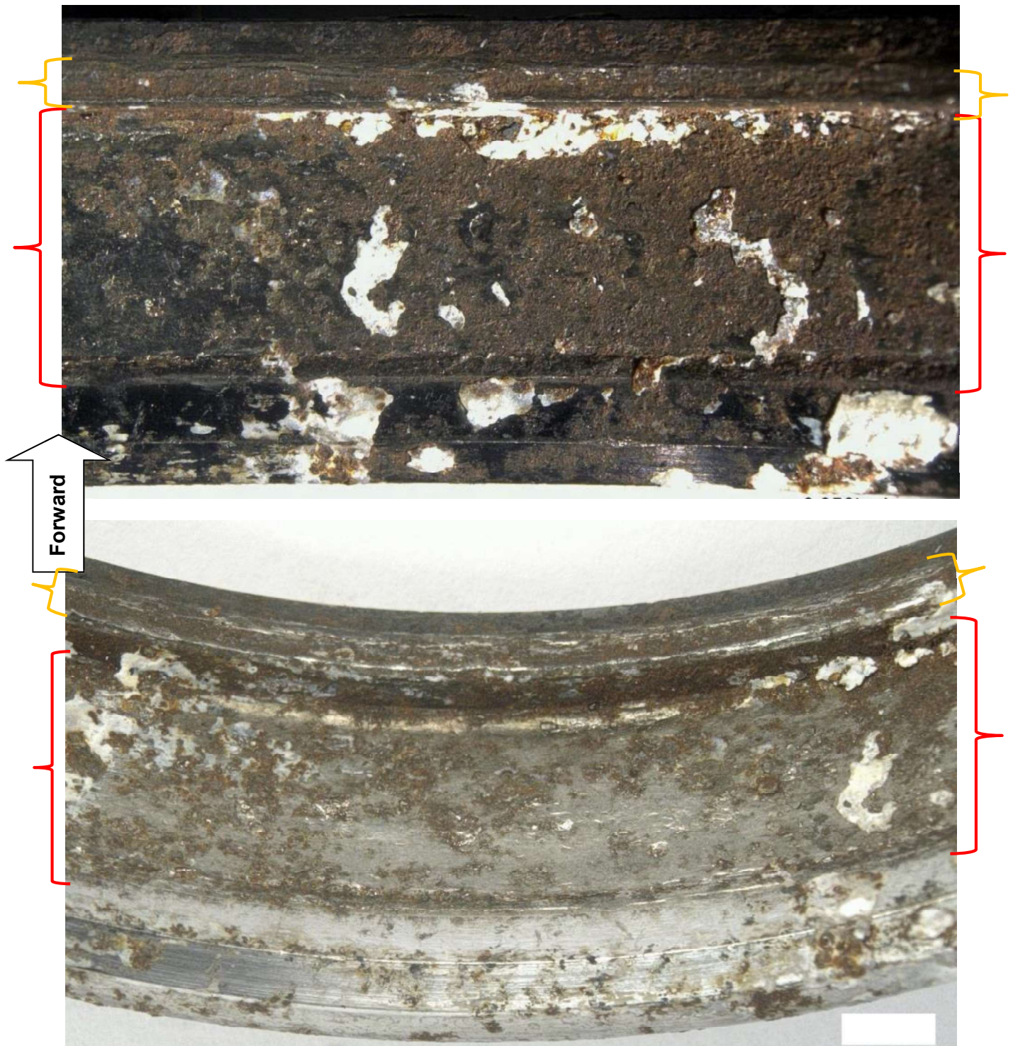
Figure 27. Detailed inboard looking outboard and oblique views of the No. 3 bearing outer ring raceway. Red braces mark the location of material removal at the roller path, and the orange braces mark rub damage on the forward shoulder corner.
