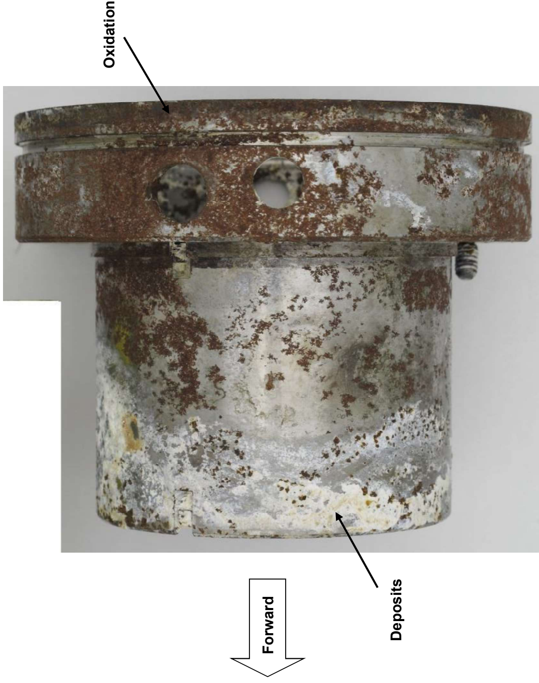
Figure 24. General condition of the bearing-stepped pinion cage after cleaning.
