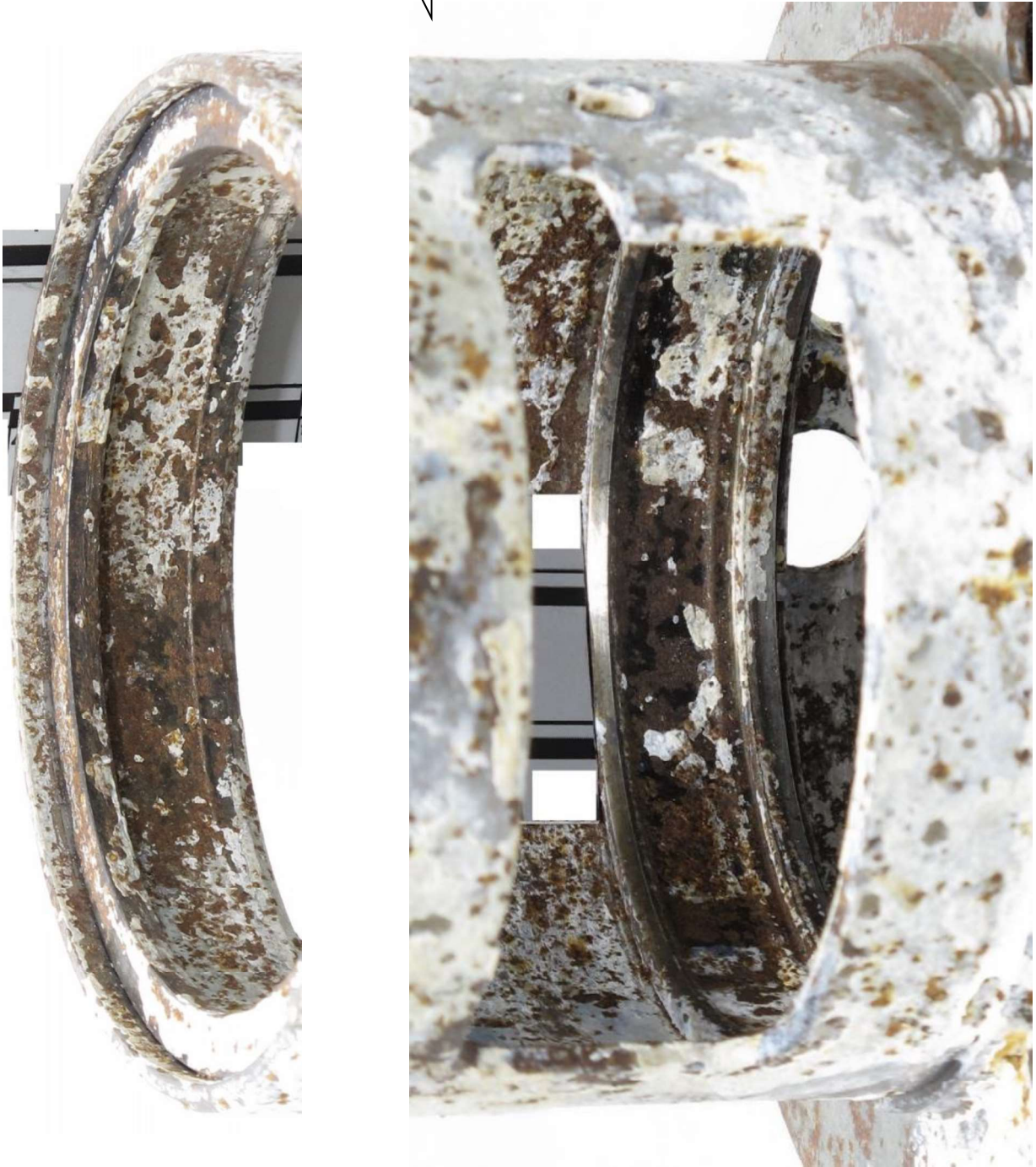
Figure 25. Detailed views of the No. 3 bearing (left) and No. 4 bearing (right) outer rings assembled in the bearing-stepped pinion cage.
