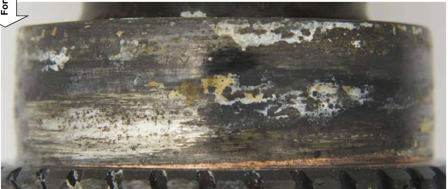
Figure 6. Detailed views of No. 4 bearing journal, which exhibited circumferential rub. Each image shows the part rotated ~90° from the previous.
