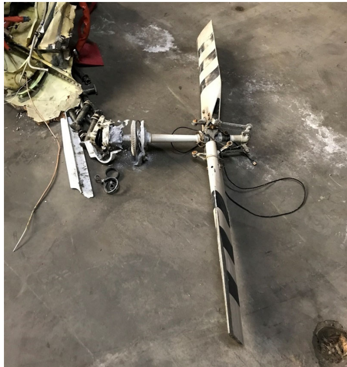
Figure 4. The recovered tail rotor and tail rotor gearbox.
