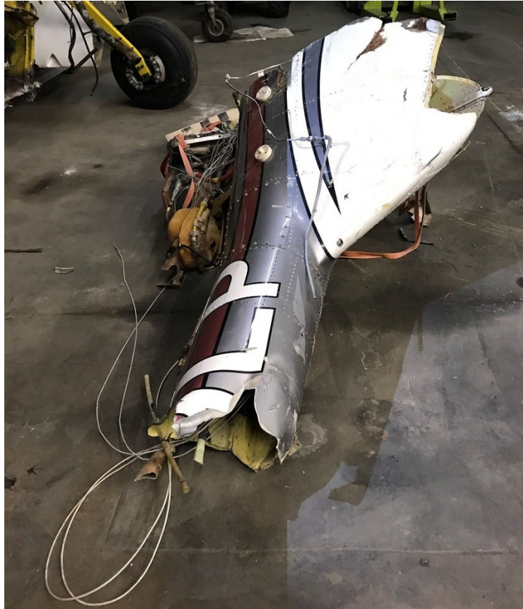
Figure 2. The separated section of intermediate fuselage and tail boom.
