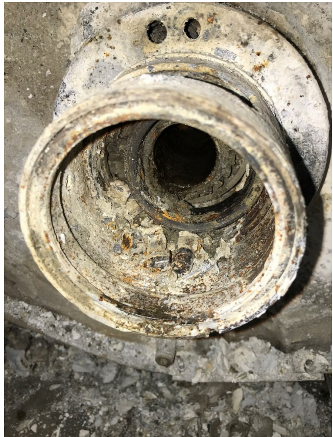
Figure 8. Roller elements from the No. 4 bearing found in the bearing support housing.
