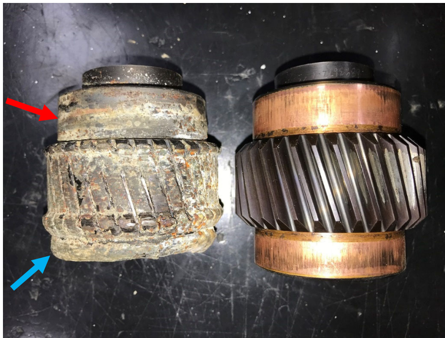
Figure 13. A comparison of the recovered power turbine pinion gear (left) and an exemplar power turbine pinion gear (right). The blue arrow points to the No. 3 bearing shoulder and the red arrow points to the No. 4 bearing shoulder.
