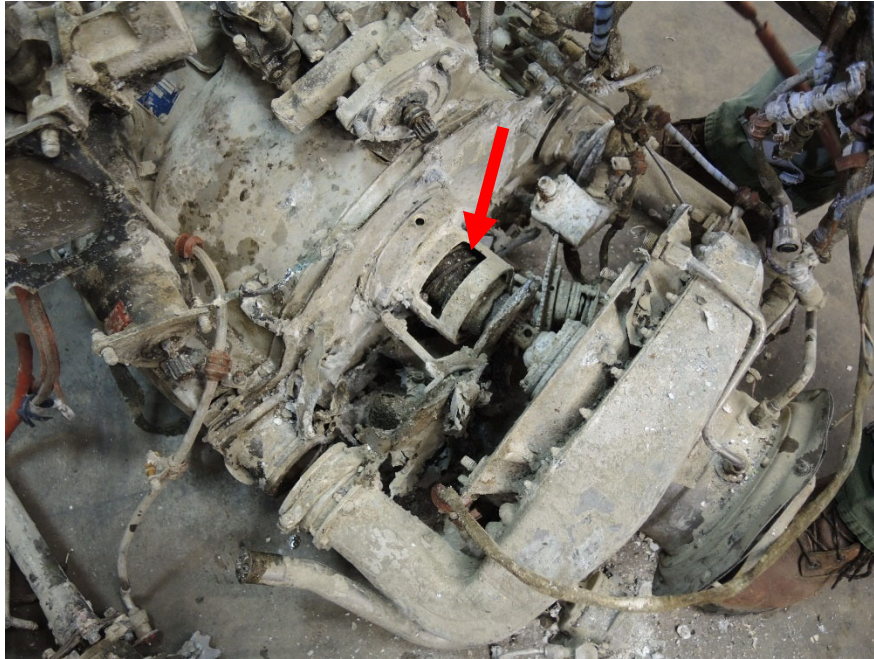
Figure 6. A view of the area where the engine accessory gearbox housing is normally present. The red arrow points to the area of the power turbine pinion gear and the Nos. 3 and 4 roller bearings.
