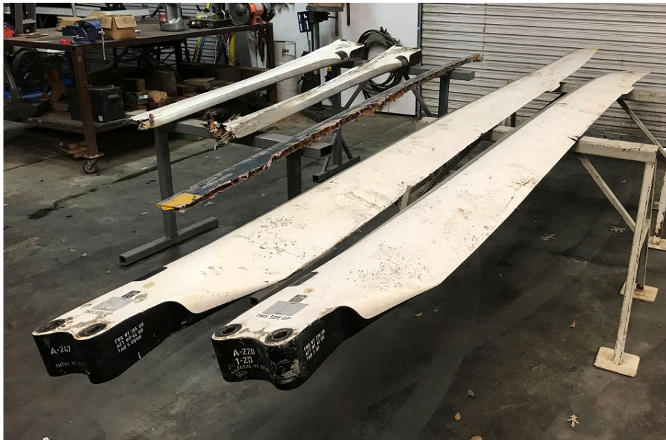
Figure 3. The recovered main rotor blades.
