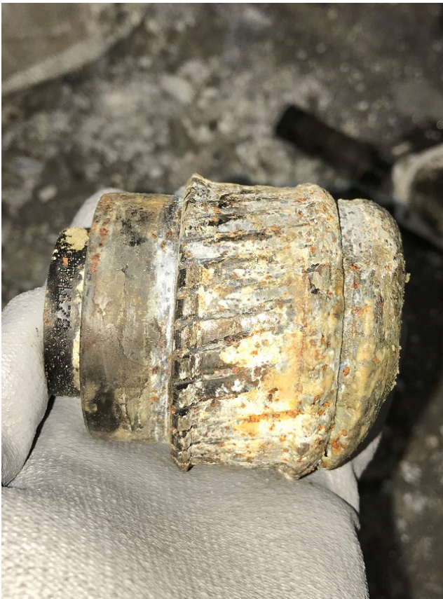
Figure 7. The recovered power turbine pinion gear exhibited smearing damage.
