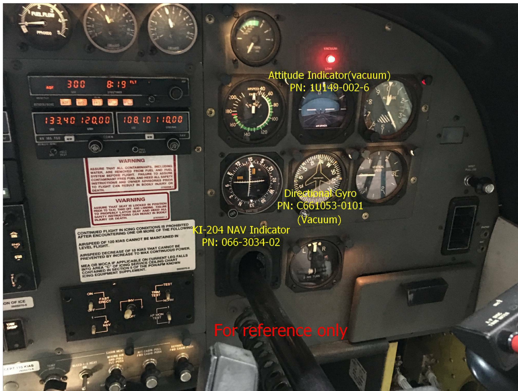
Photo 3 – Right Side of Cockpit Instrument Panel Prior to Accident
