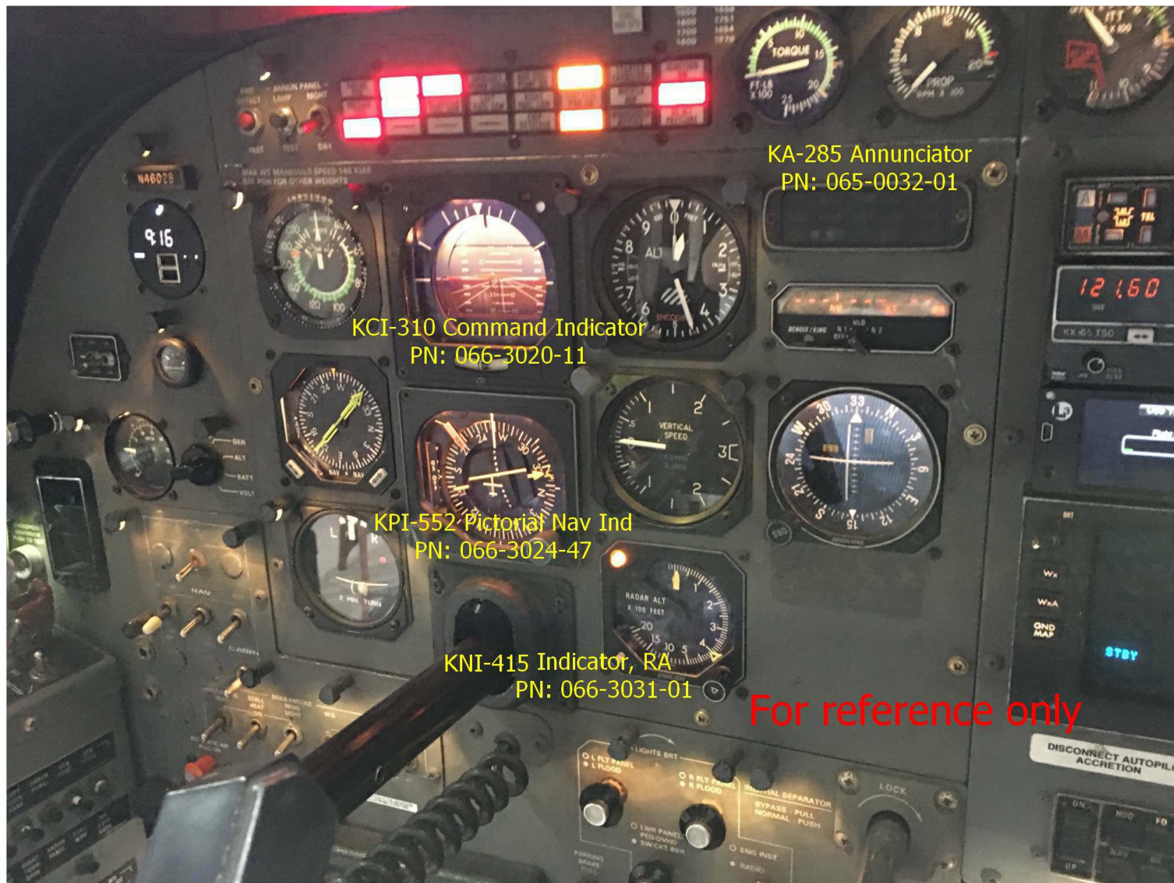
Photo 1 – Left Side of Cockpit Instrument Panel Prior to Accident
