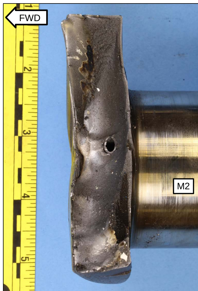
Figure 1. Overall view of the submitted crankshaft pieces (above) with a closer view of the fracture surface on the aft piece (right).
