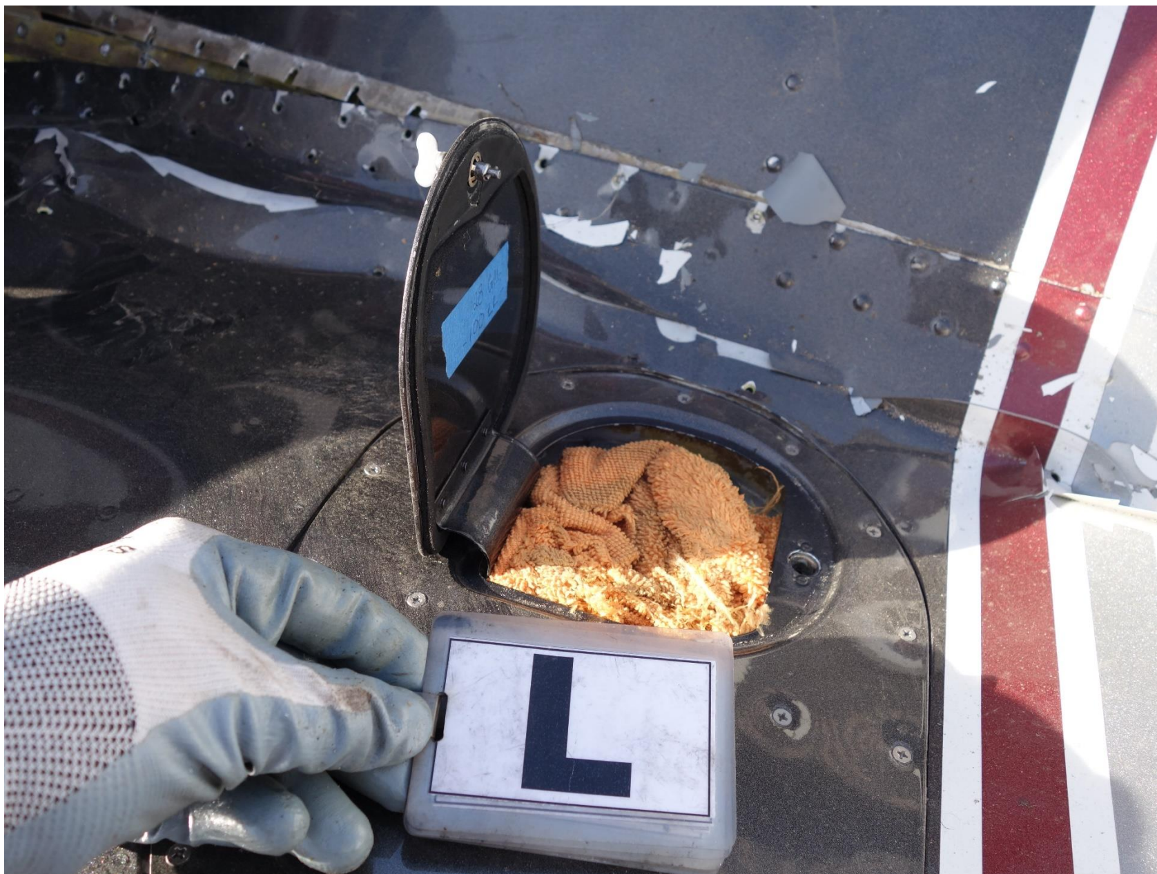
Photo 3 – Rag Over Left Fuel Cap (Piper Photo)
