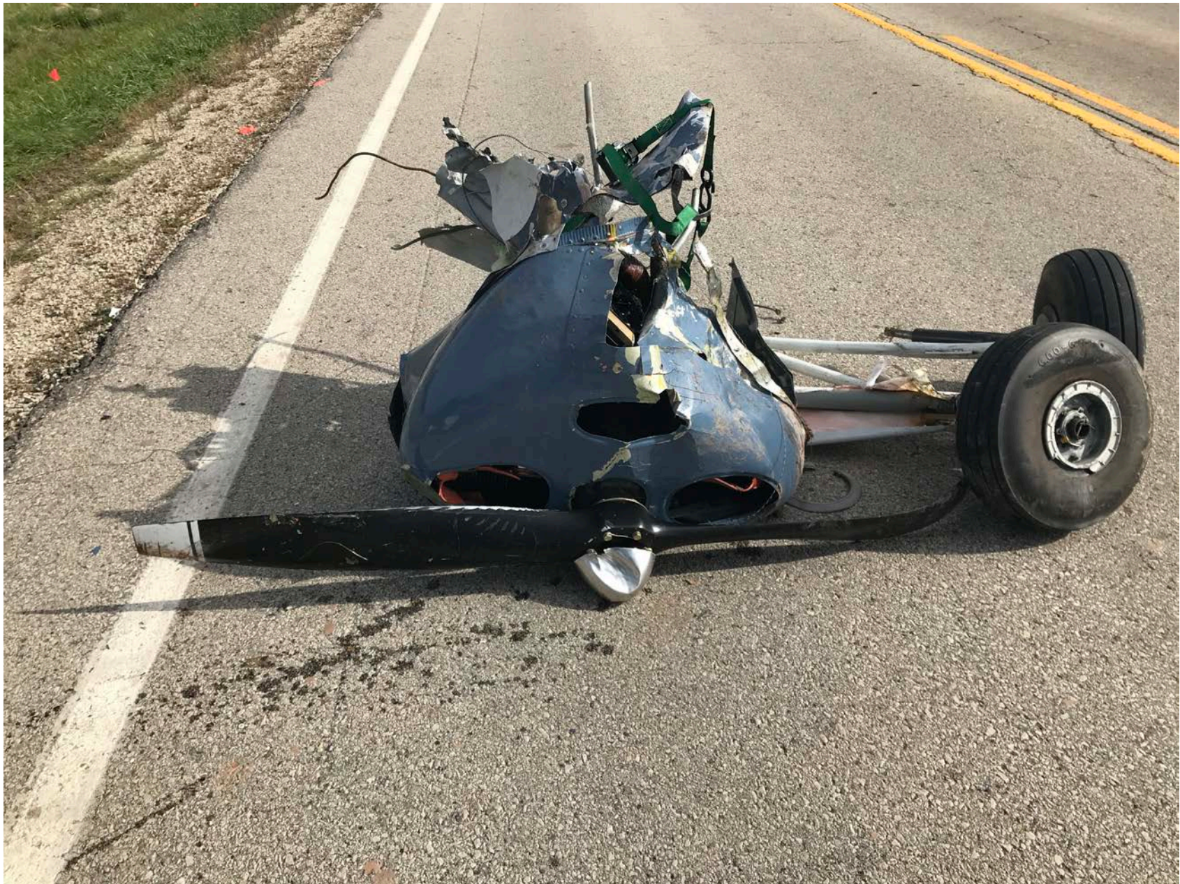
Photo 9 – Engine and propeller and landing gear recovered to the road
