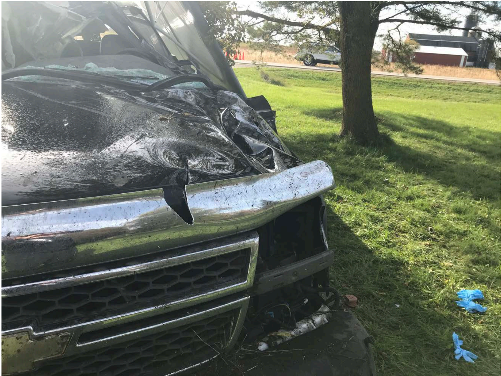
Photo 13 – Front left of truck with propeller slash marks and impact damage
