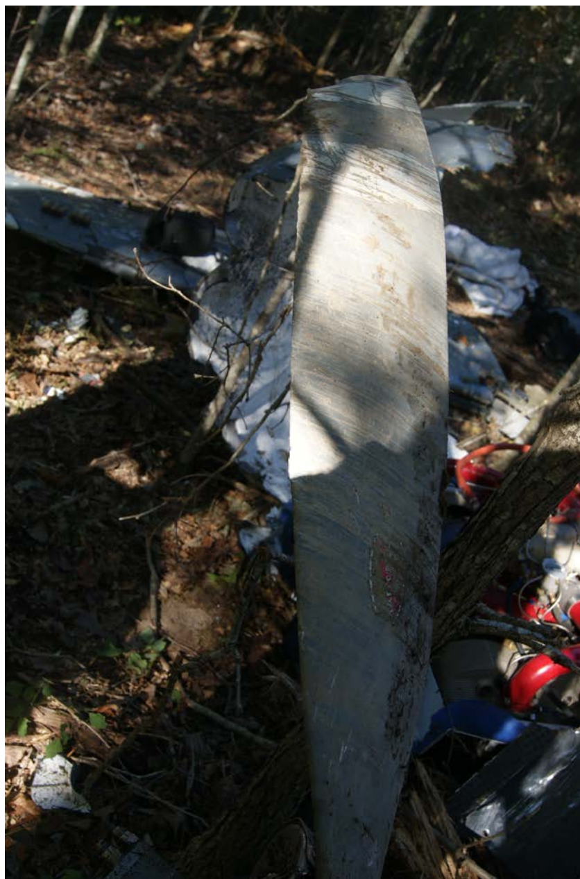
Photo 10 – Propeller blade “B.” Note 90° chordwise scratches on cambered surface (NTSB photo)
