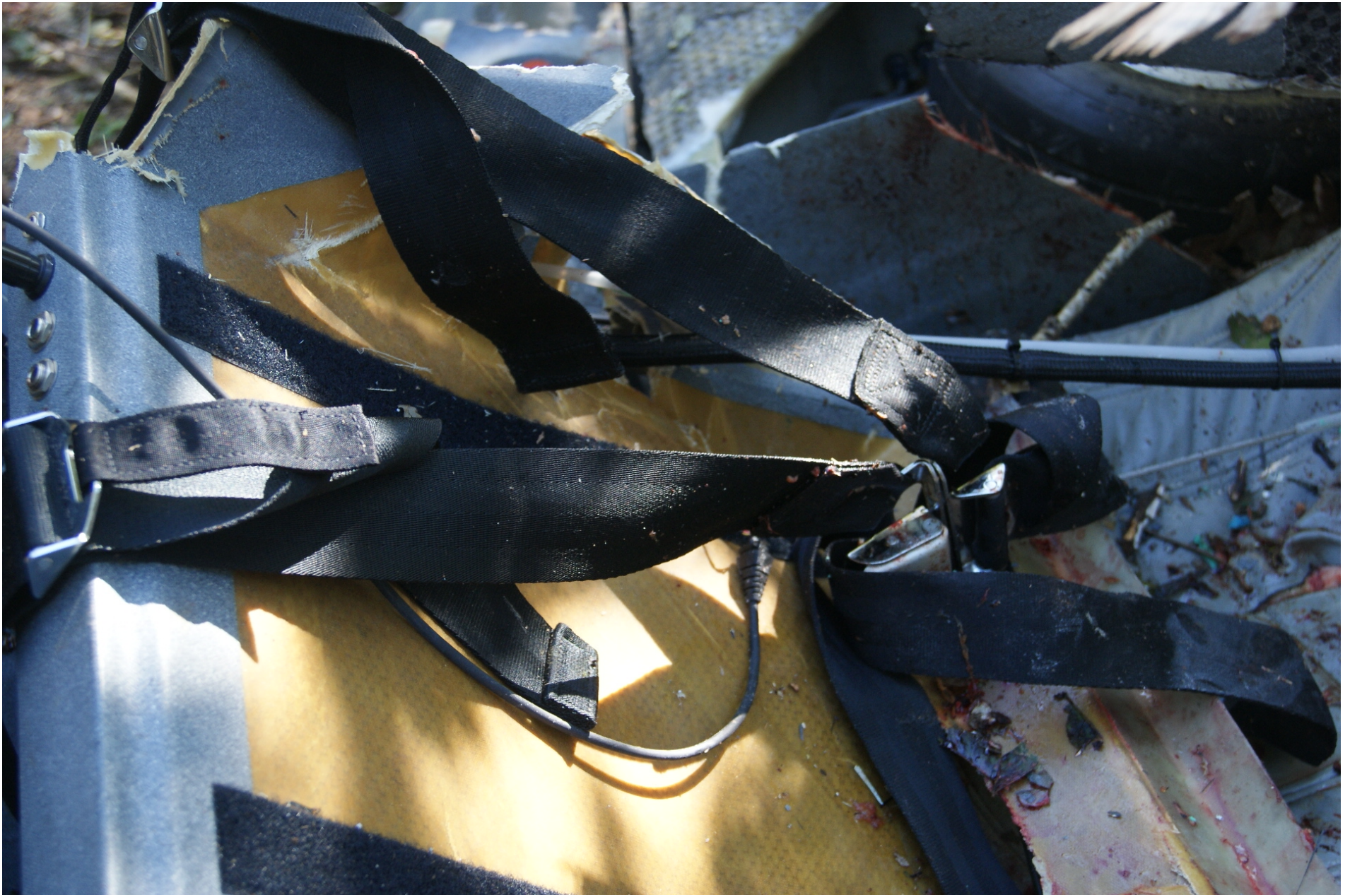
Photo 14 –4-point restraint system showed evidence of use (NTSB photo)
