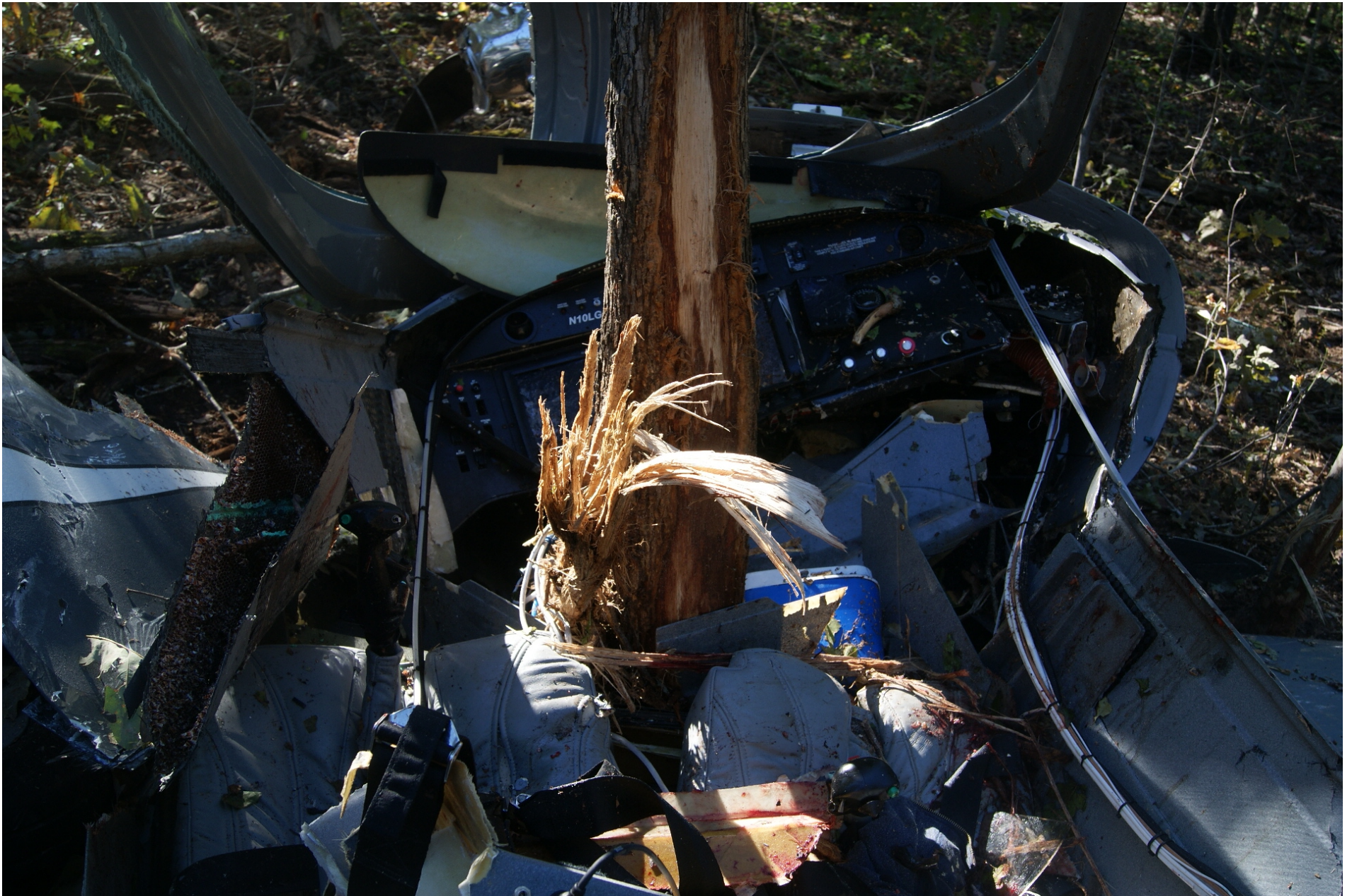
Photo 2 – Tree stump coming straight up through cockpit floor, further consistent with near-vertical descent (NTSB photo)
