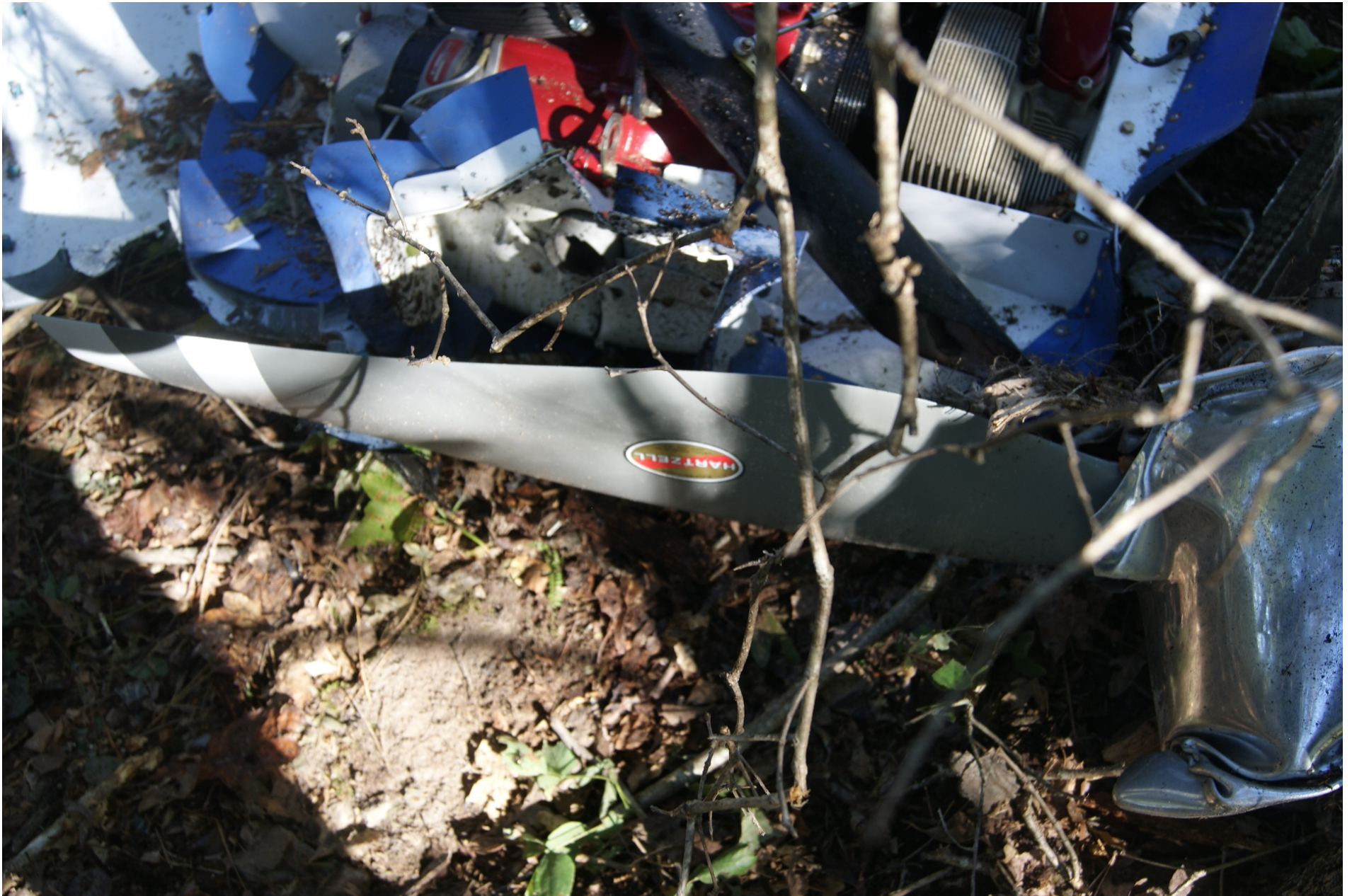
Photo 8 – Propeller spinner. Note the direction the spinner tip is crushed (NTSB photo)
