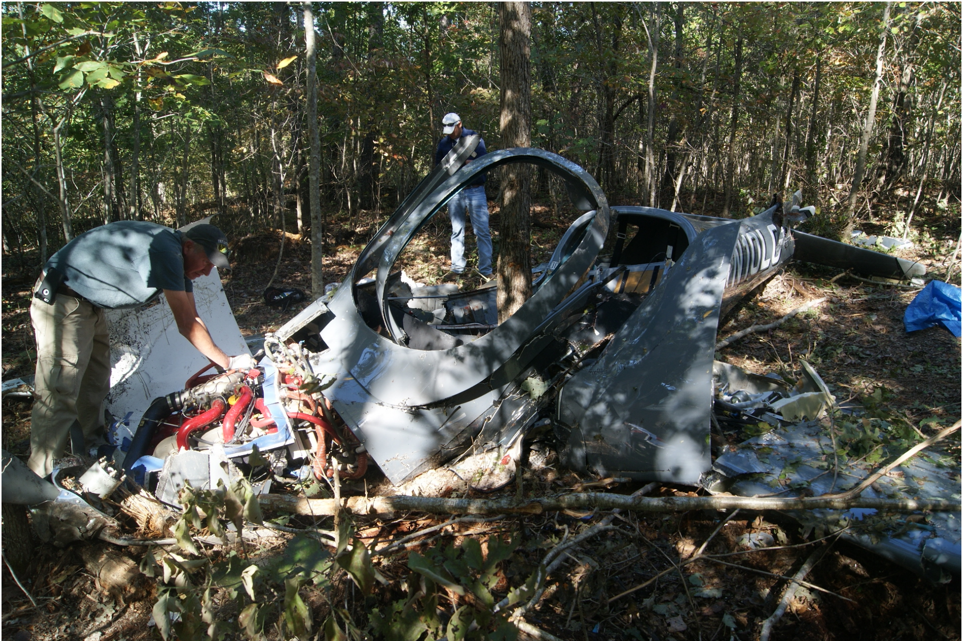
Photo 3 – Left front of airplane. Note engine is skewed to the right (NTSB photo)
