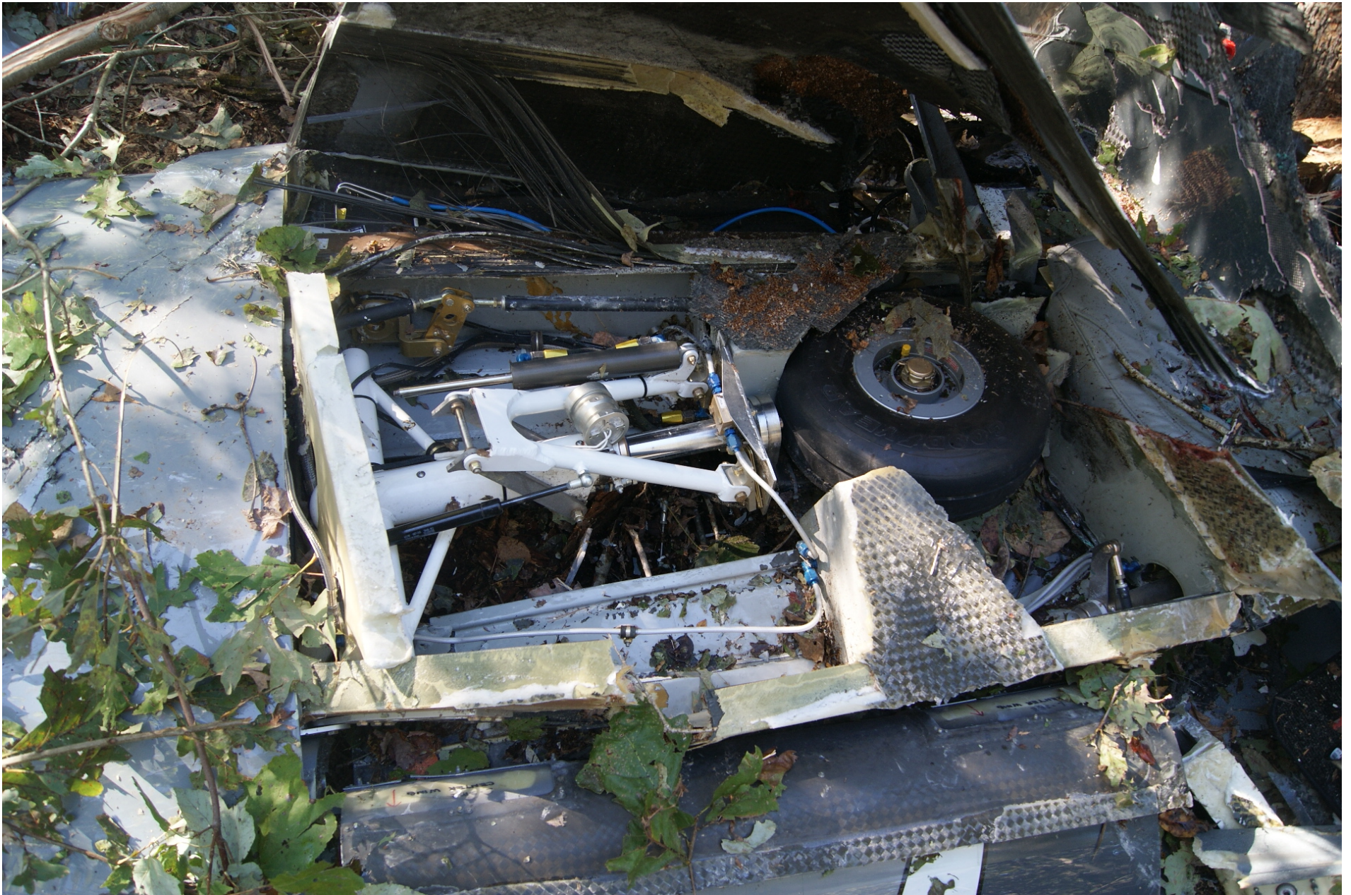
Photo 11 – Retracted left main landing gear and inverted wing (NTSB photo)
