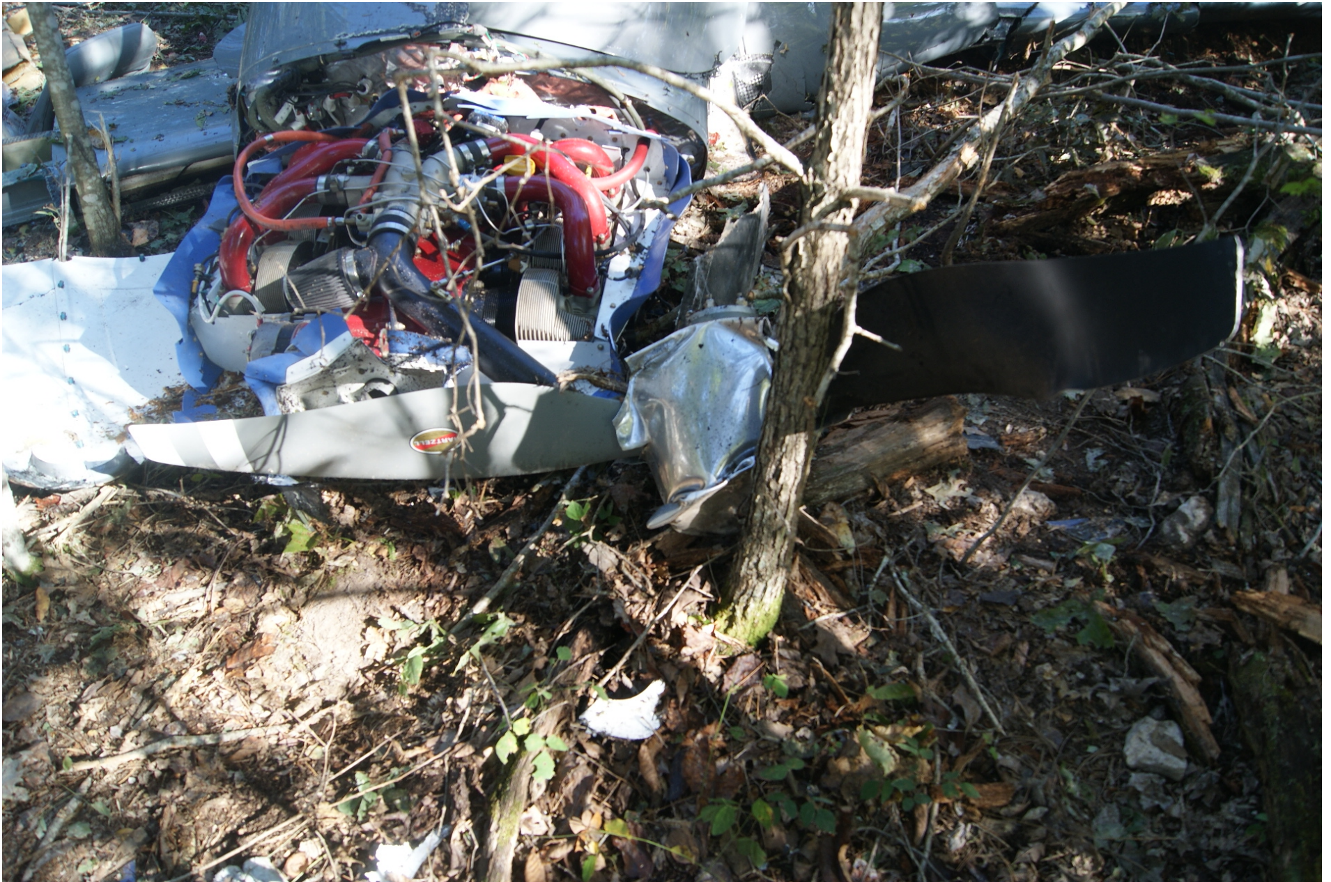
Photo 7 – The engine and separated propeller assembly (NTSB photo)
