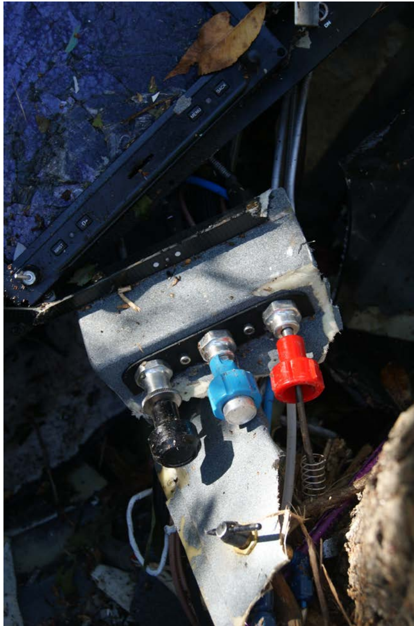
Photo 15 – Throttle, propeller, and mixture controls were found full forward (NTSB photo)
