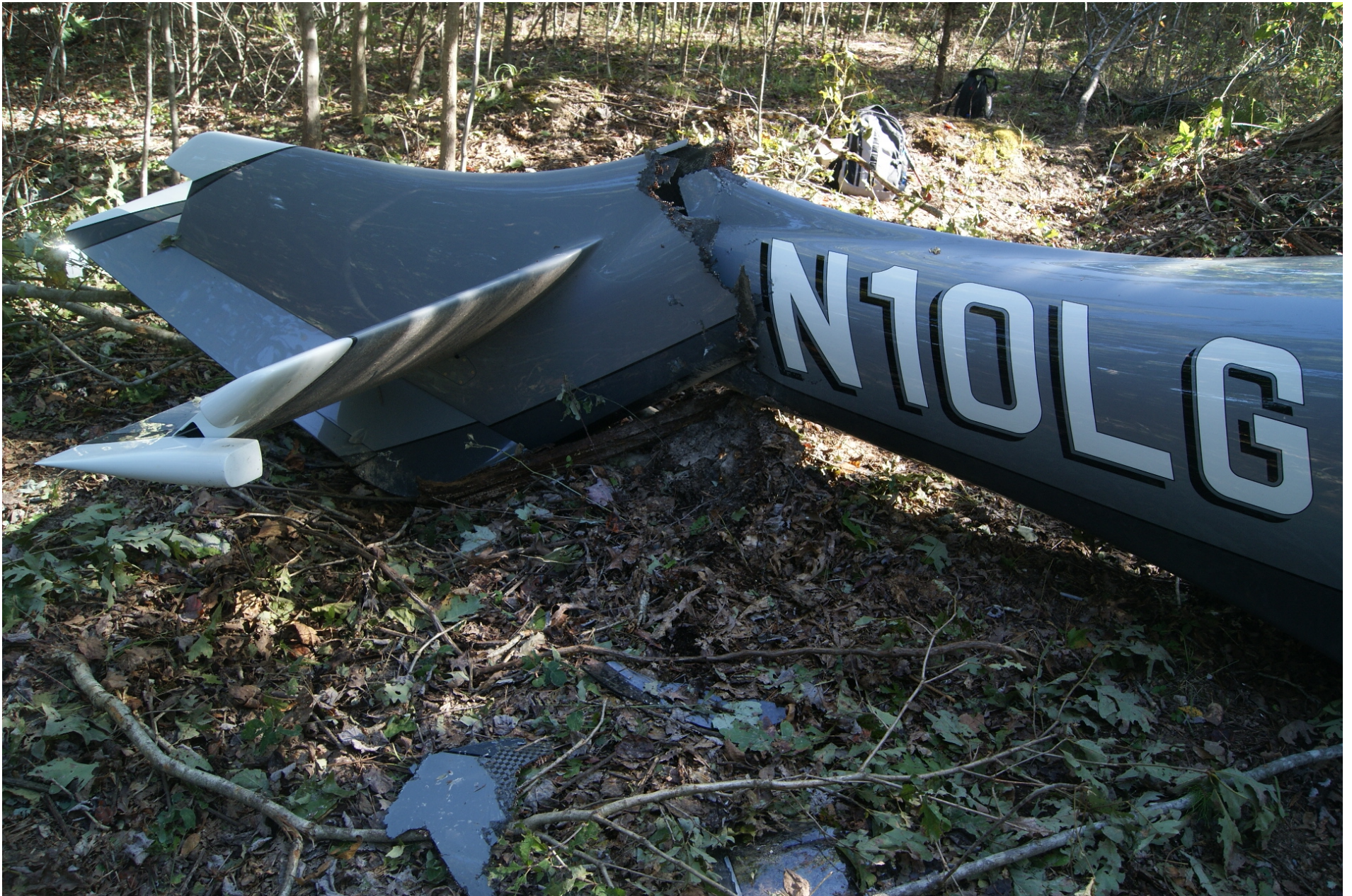
Photo 4 – Aft portion of the fuselage is fractured just forward of the empennage and skewed to the right (NTSB photo)
