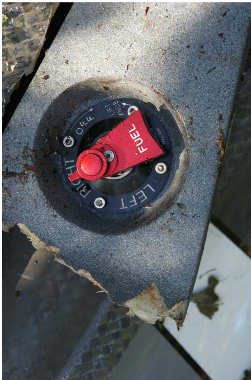
Photo 13 – Fuel selector handle was positioned on the right tank (NTSB photo)
