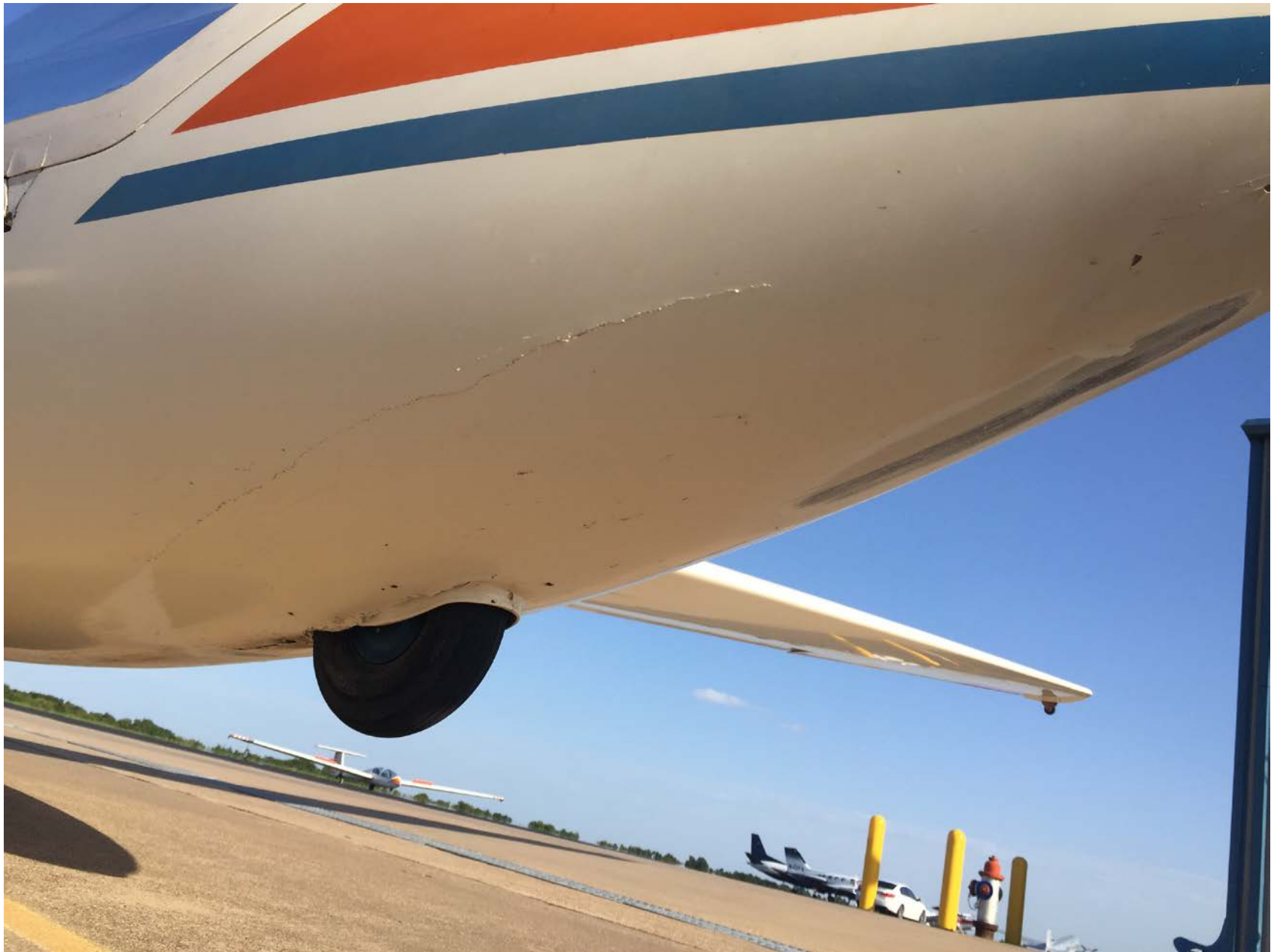
Photo 2 – Cracked fiberglass on right side of nose (FAA photo)
