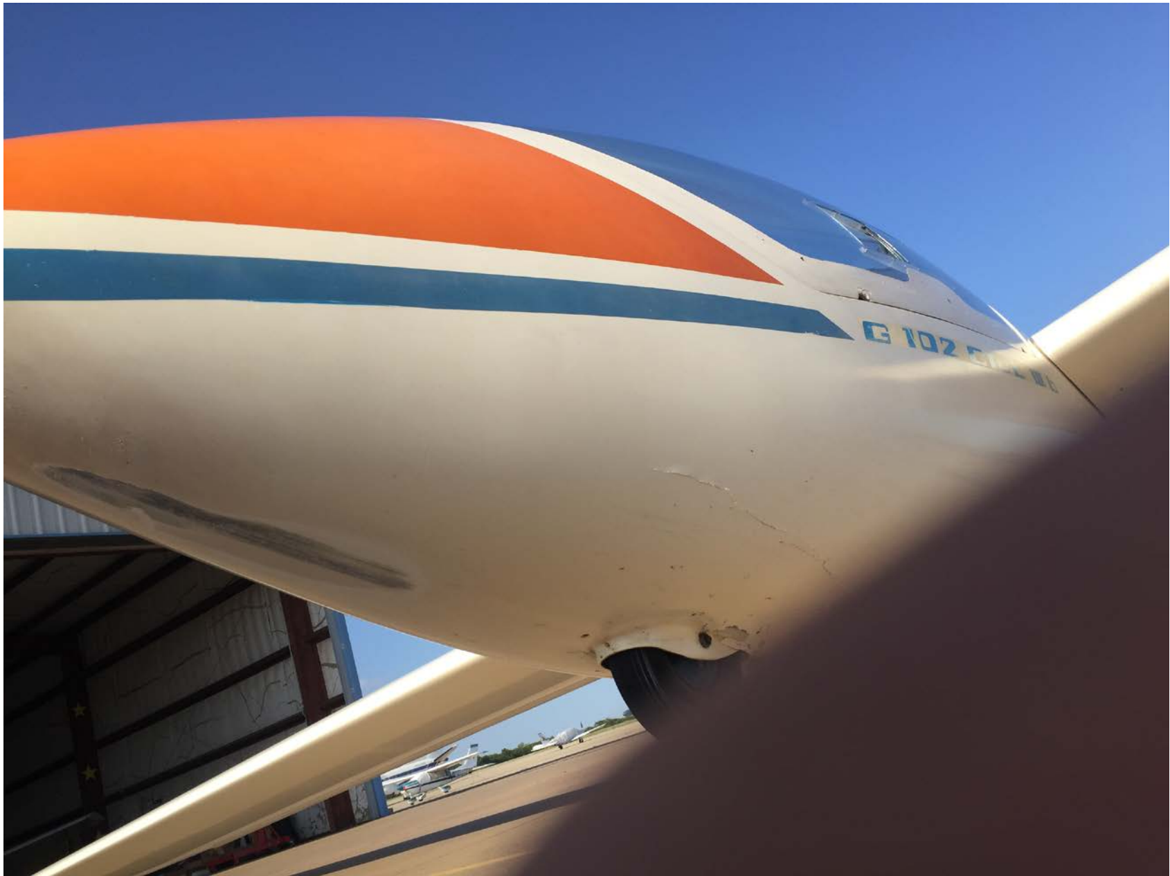
Photo 1 – Scuff mark on nose and cracked fiberglass on left side (FAA photo)
