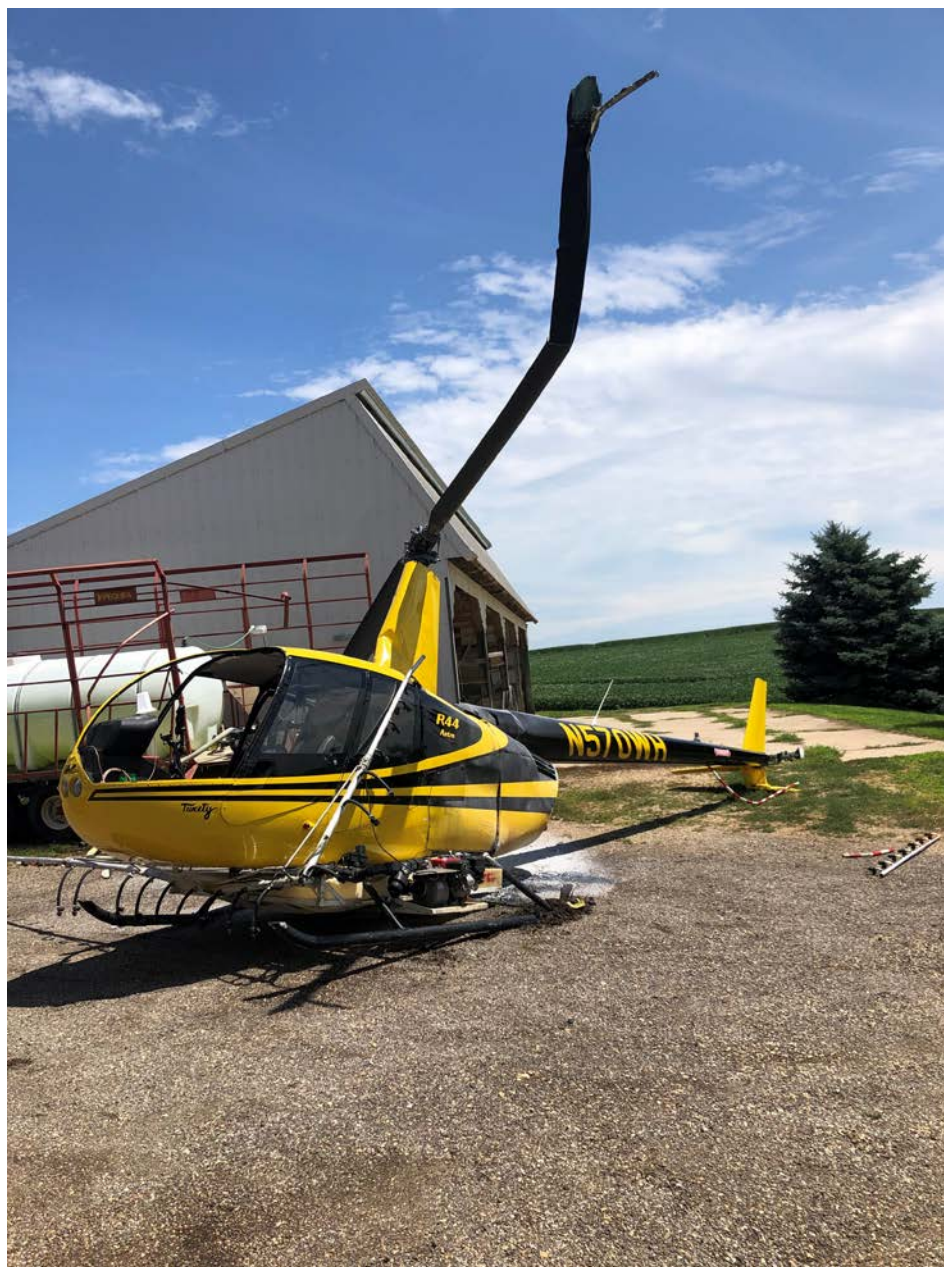
Photo 2 - Supplied photo with a quartering view of the left, front of the helicopter. The helicopter exhibits deformation in fuselage and tailboom skins.
