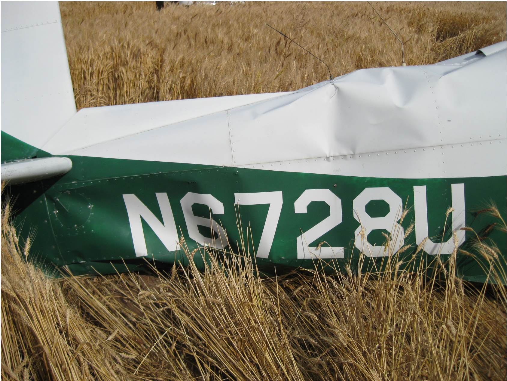
Photo 2 – Closeup of Deformation to Empennage
