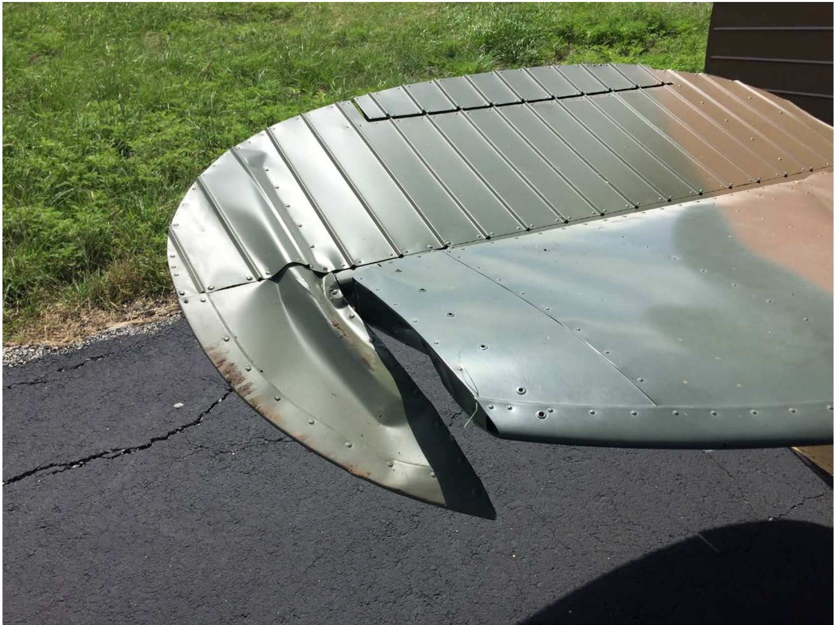
Photo 2 – Right Horizontal Stabilizer and Elevator
