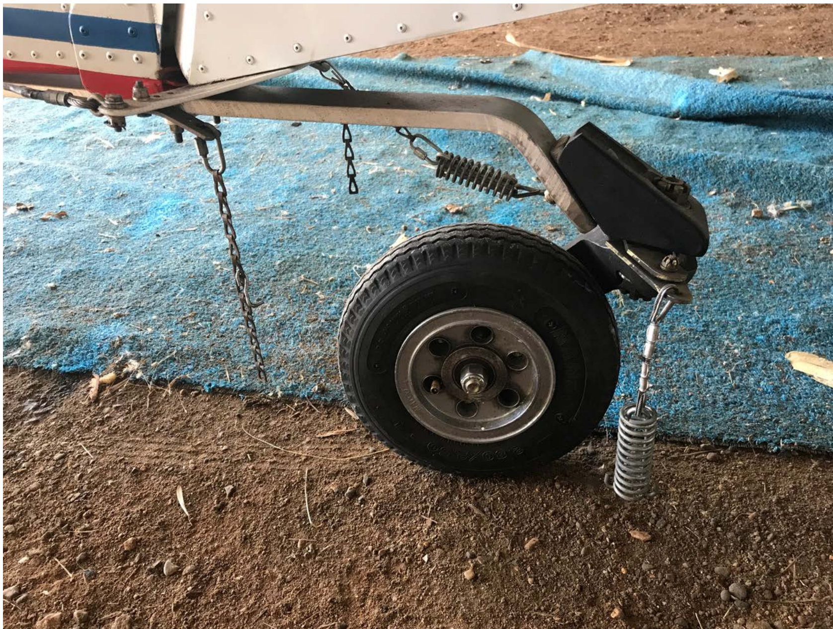
Photo 2 – Broken tailwheel chain
