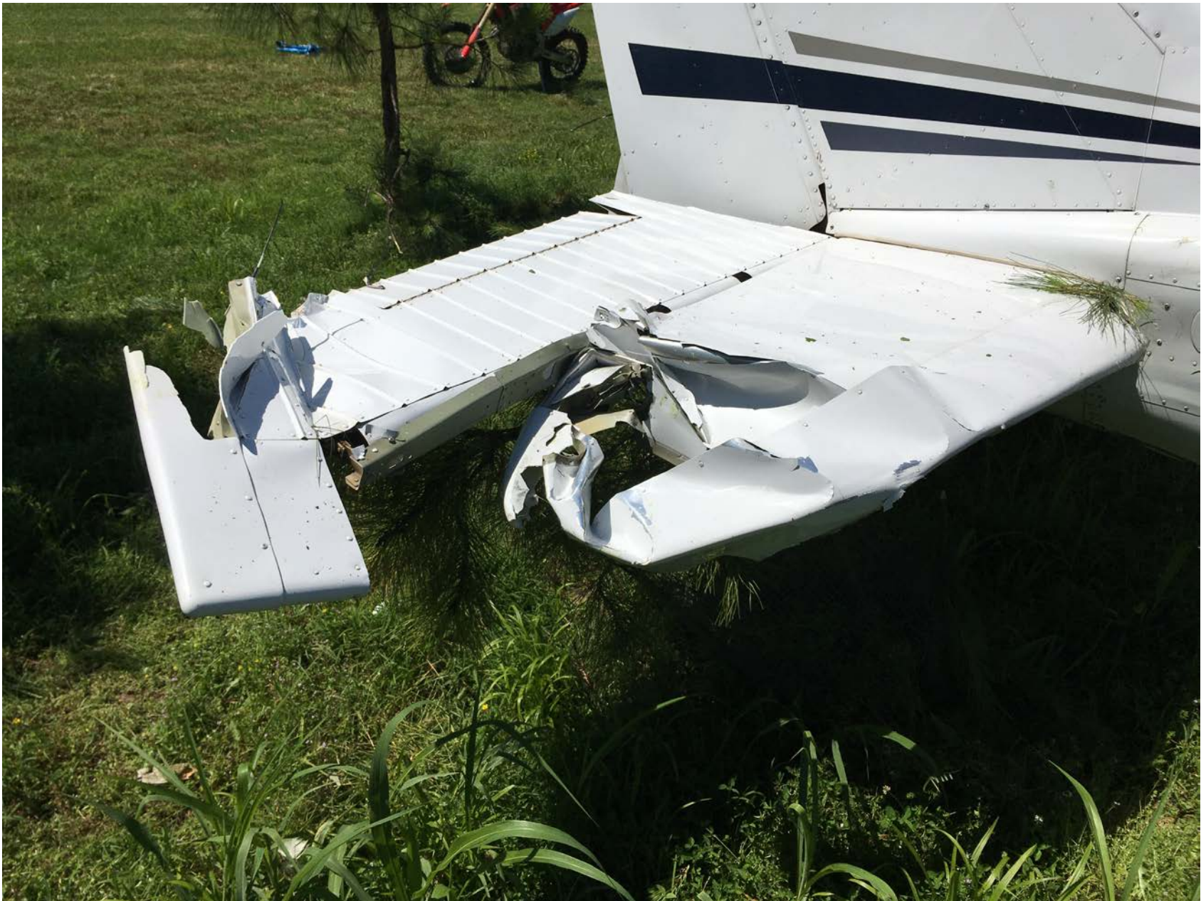
Photo 5 – Right horizontal stabilizer, elevator, and rudder damage and skin wrinkling
