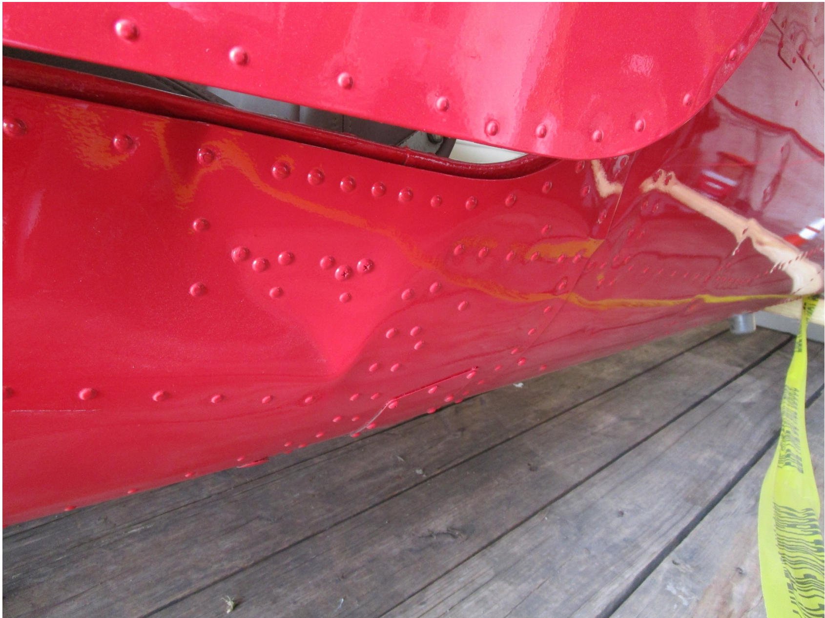
Photo 5 - Supplied view of the deformed fuselage below the pilot's door.
