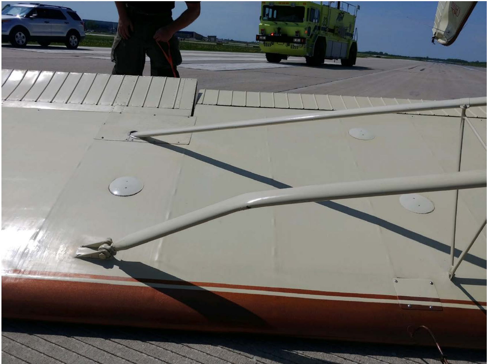
Photo 3 - Wing strut damage
