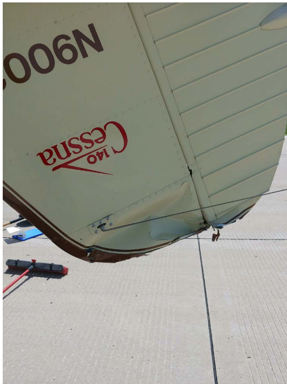
Photo 2 – Damage to the vertical stab and rudder
