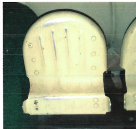
SMAT 1958 C182A N5179D Copilots pedals/1959 C182B example shows contact between carpet and pedal
