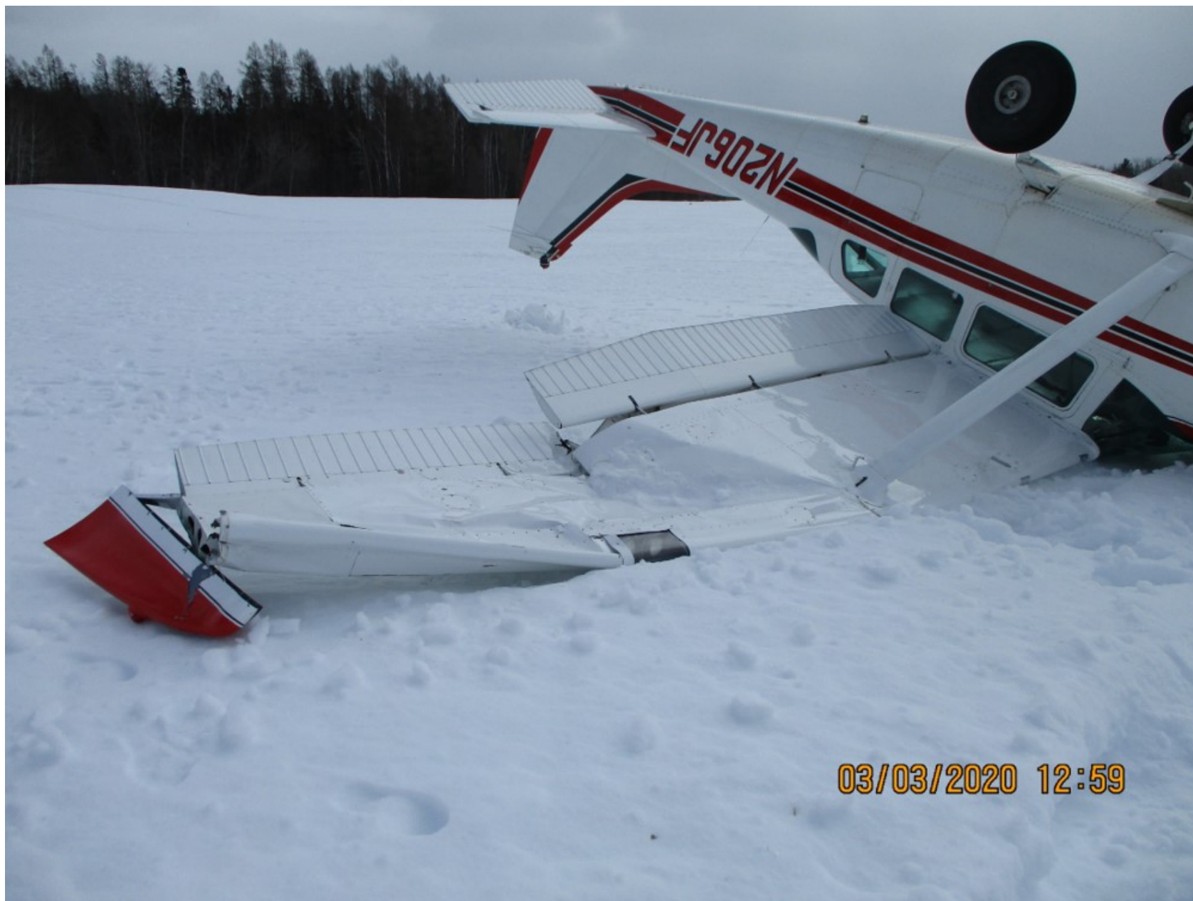
Photo 1 – View of substantial damage to the left wing spar (Courtesy of FAA)
