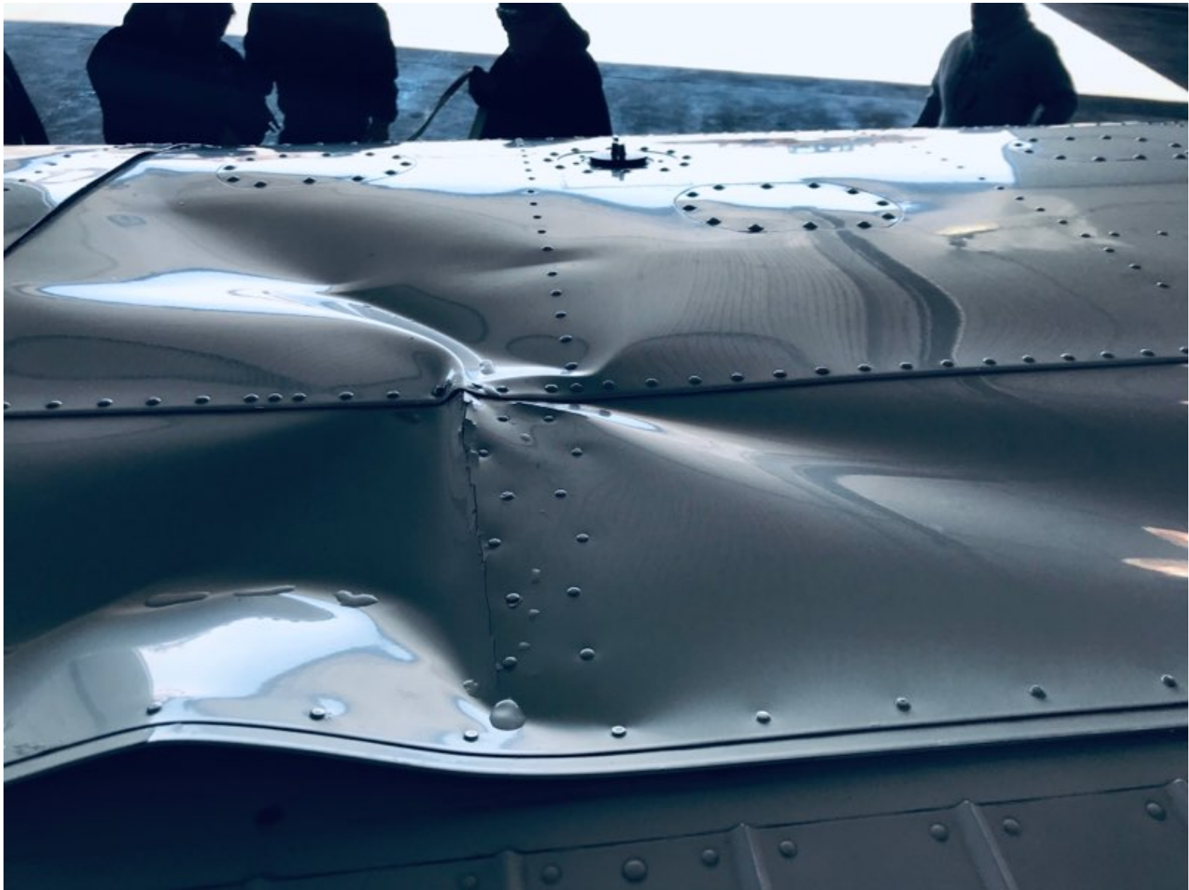
Photo 2 – Right Wing Damage (Airport Operations Photo)
