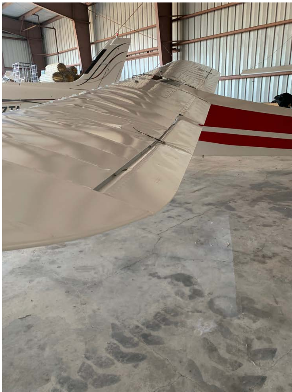
Photo 2 – Left wing damage as seen from the top.
