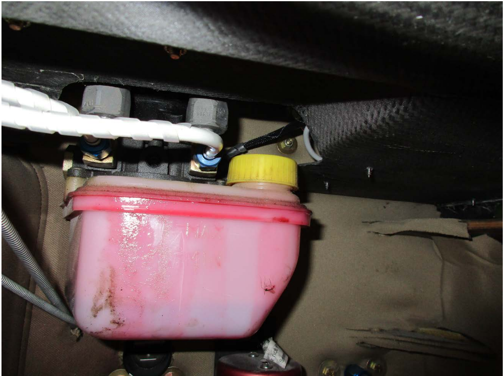
Photo 1 – Hydraulic Reservoir (FAA)
