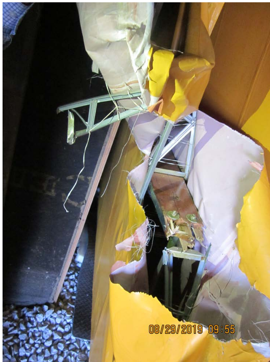
Photograph 2 – Damage Right Rib and Spar (Provided by FAA)
