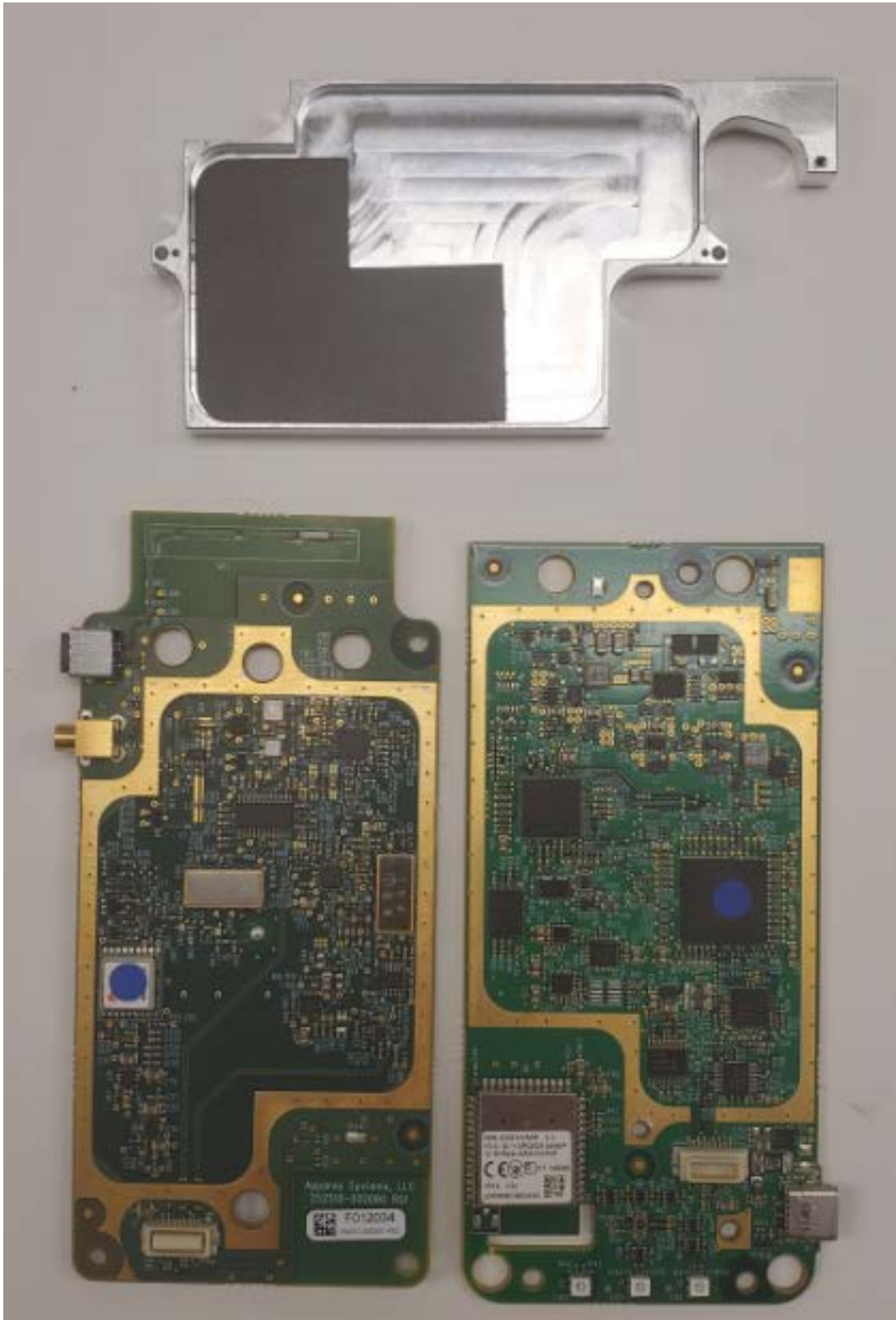
Figure 2: Circuit boards of the Appareo Stratus 2S.
