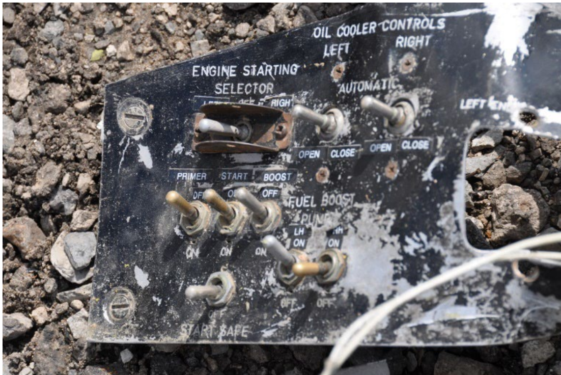
Figure 6 - Engine Starting Selector and Oil Cooler Portion of Panel
