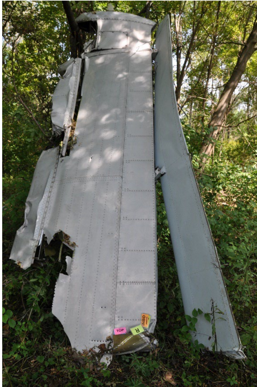
Figure 31 - Outboard Section of Right Wing, in wooded area. Note aileron attached to rear of wing section.
