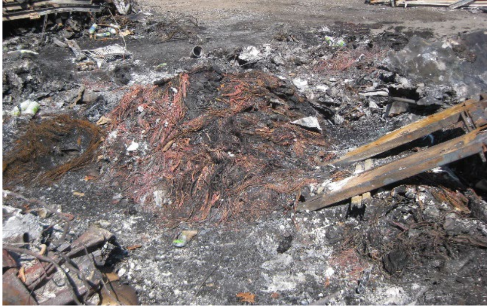
Figure 34 - Mound of Copper Wiring and Melted Plastic from Airplane Cargo
