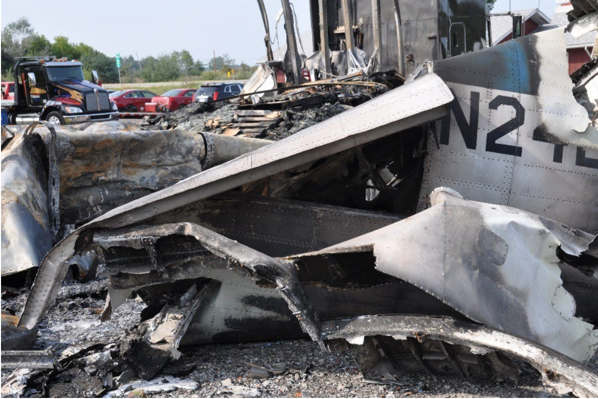
Figure 25 - Main Cargo Door, bent over but still in fuselage doorway.
