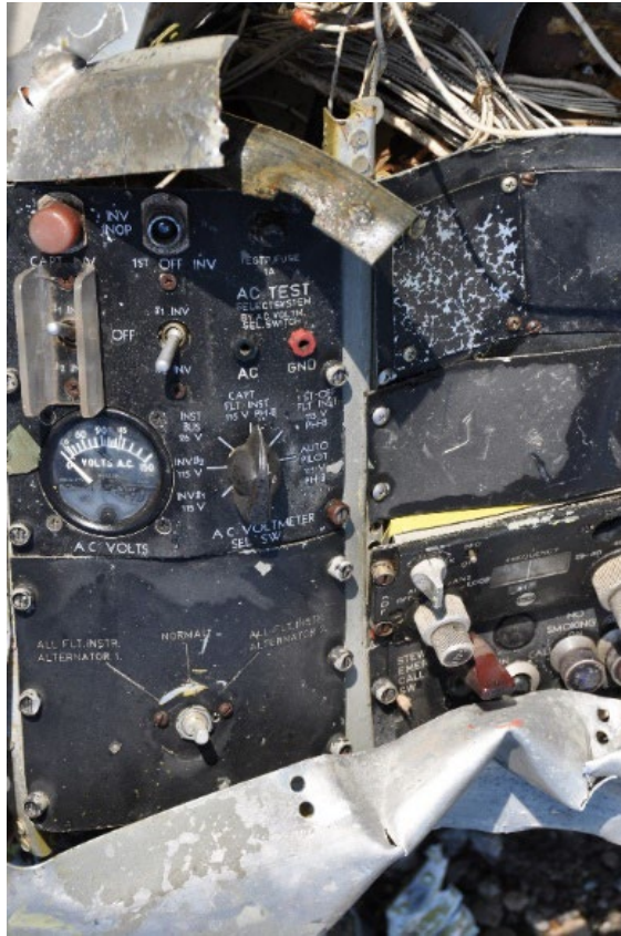
Figure 3 - Inverter Panel Section
