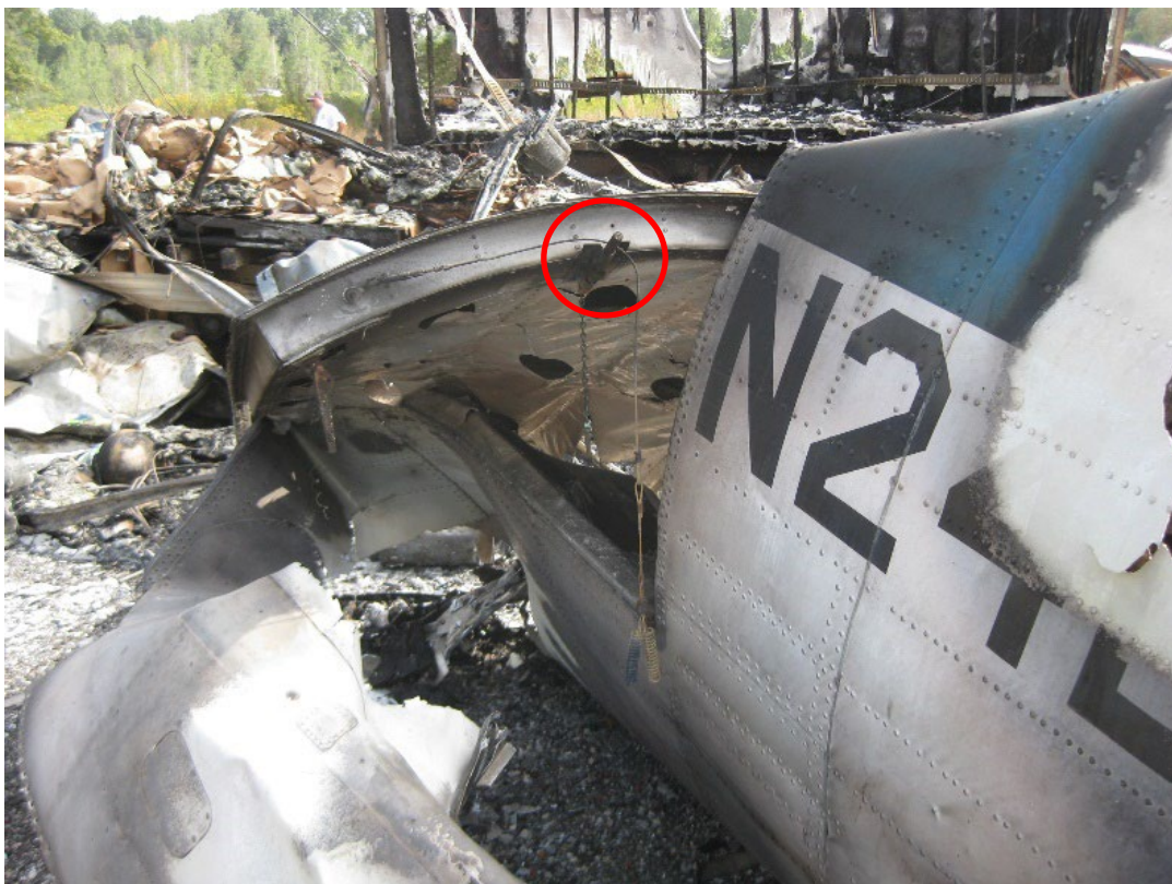
Figure 26 - Side View of Main Cargo Door, with bolt-style latch in red circle.
