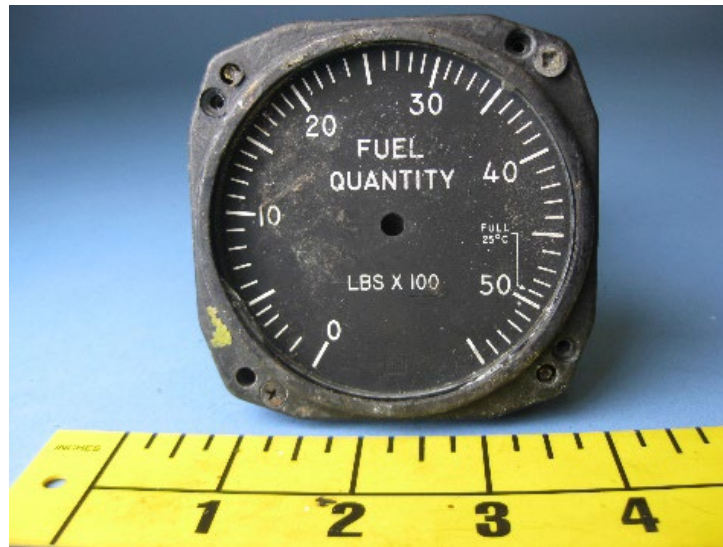
Figure 10 - Fuel Quantity Indicator
