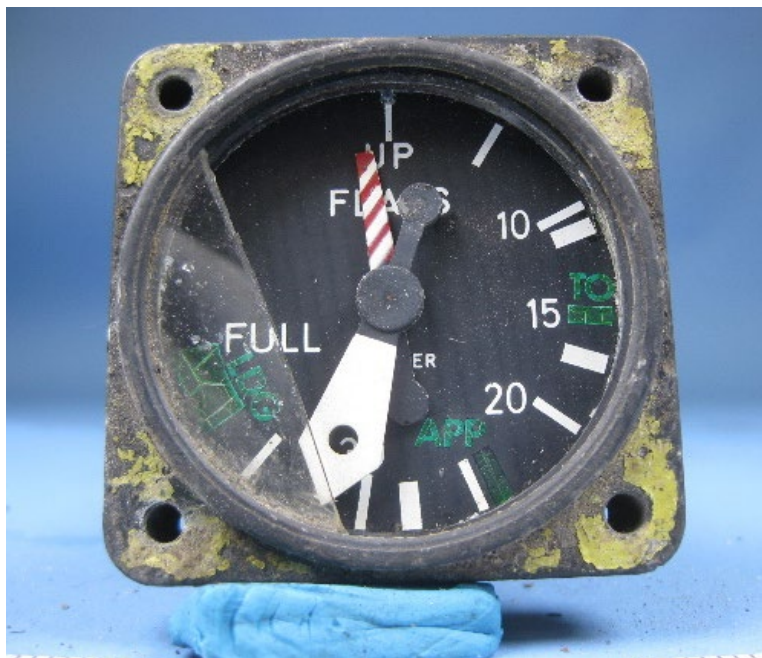
Figure 17 - Flap Indicator, After Glass Face Removed
