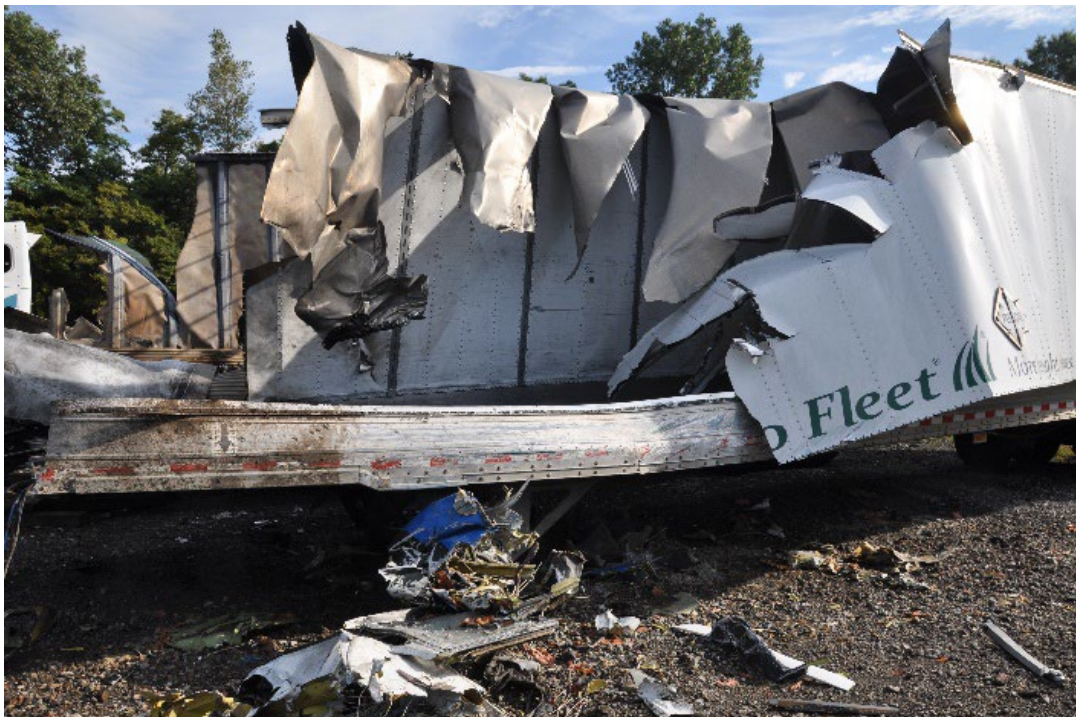
Figure 23 - Side of trailer showing impact strikes and airplane wreckage.
