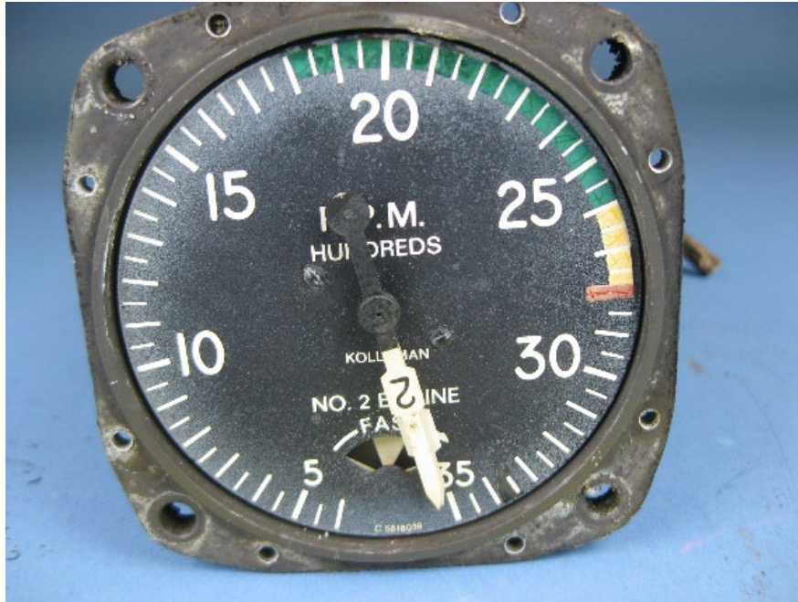
Figure 19 - Engine Tachometer, with Glass Face Removed
