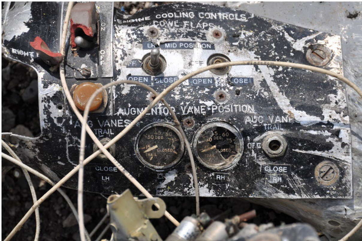
Figure 7 - Engine Cooling Controls Section of Panel
