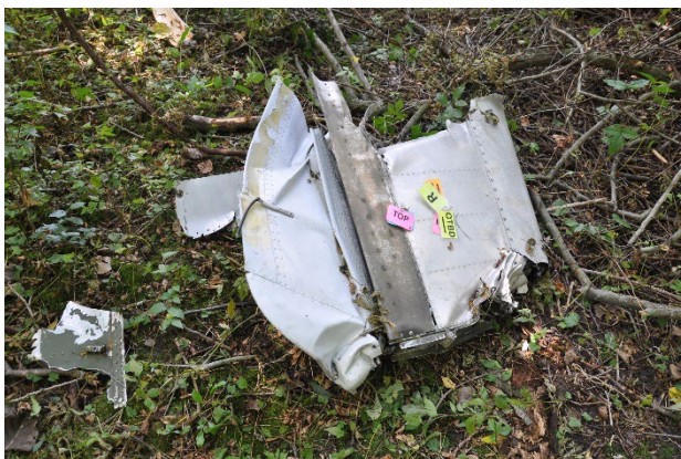
Figure 28 - Outboard Section of Right Horizontal Stabilizer and Elevator
