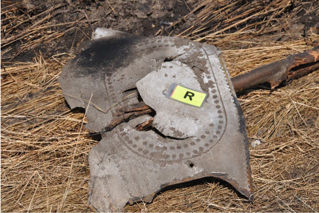
Figure 32 - Wing Access Panel from Right Wing, with tree branch.
