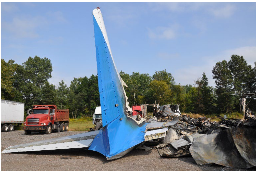
Figure 27 - Airplane Empennage, facing opposite direction of flight. Note missing section of right-hand stabilizer.
