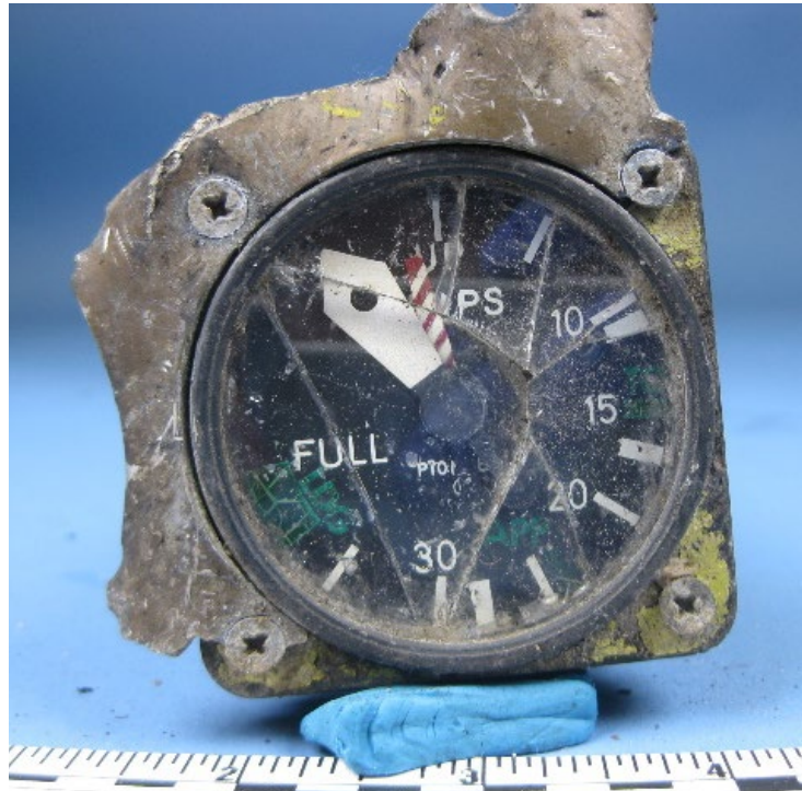
Figure 16 - Flap Indicator, Before Glass Removal
