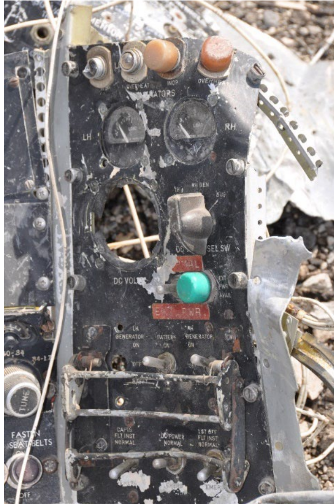
Figure 5 – Generator Section of Panel
