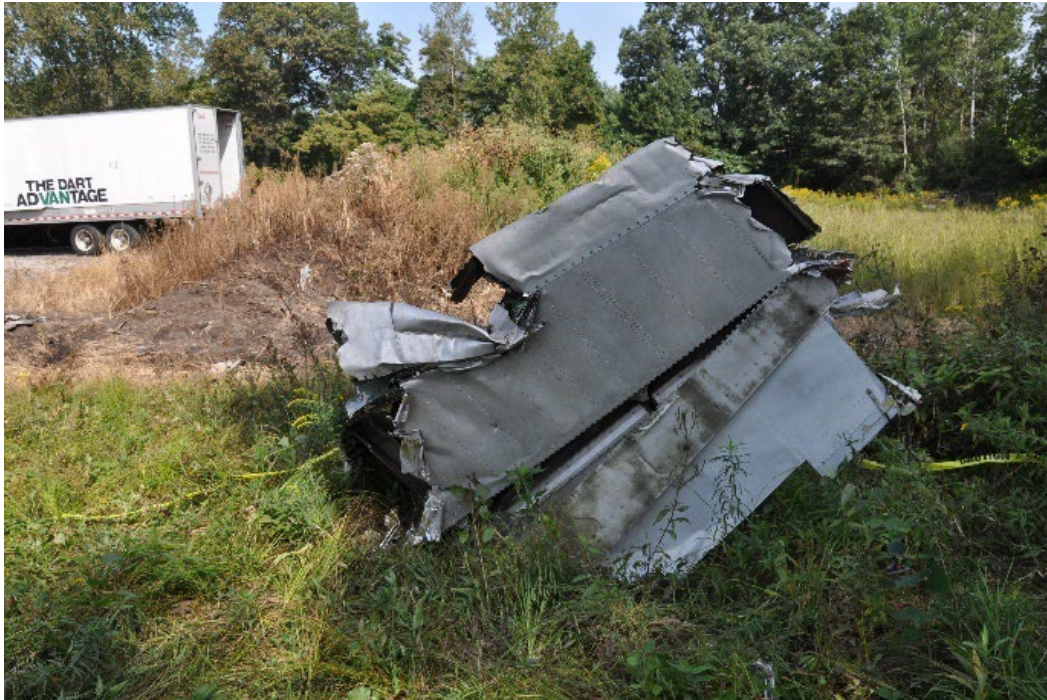
Figure 29 - Section of Right Horizontal Stabilizer and Elevator, stuck in ground. The top of the stabilizer is facing the photographer.
