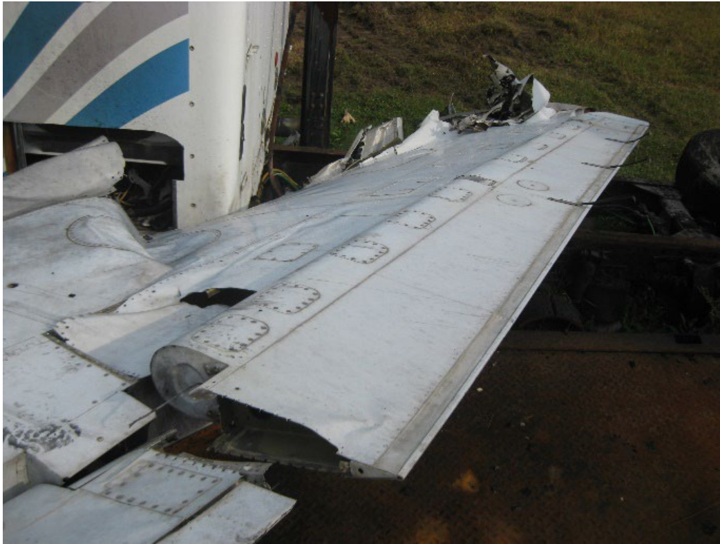
Figure 30 - Outboard Section of Left Wing, found upside down on a truck and trailer.
