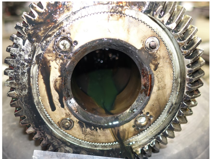
Photo 46- Blades 2 and 3, Bushing Retaining Pin and Screw Damage
