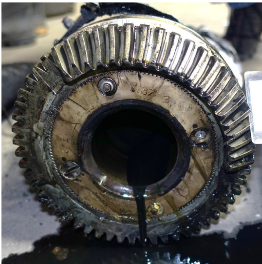
Photo 46- Blades 2 and 3, Bushing Retaining Pin and Screw Damage
