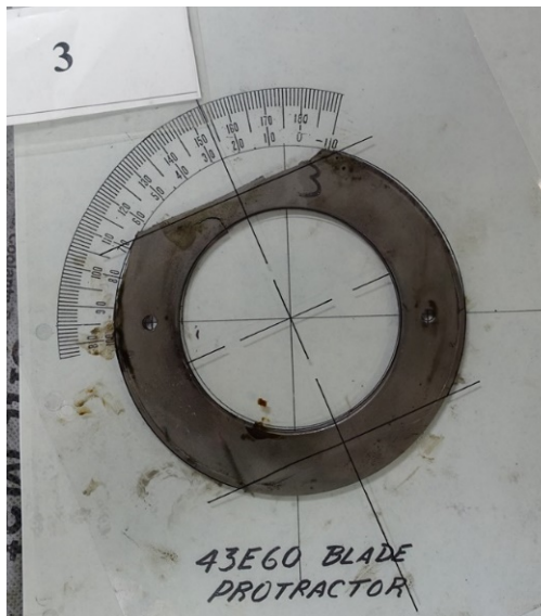
Photo 45- Right Propeller, Blade 3 Witness Marks with Blade Angle Protractor
