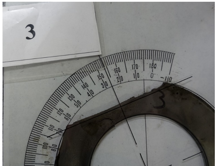
Photo 45- Right Propeller, Blade 3 Witness Marks with Blade Angle Protractor
