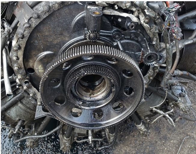
Photo 13- Reduction Drive Gear Deformation and Propeller Shaft Journal Scoring
