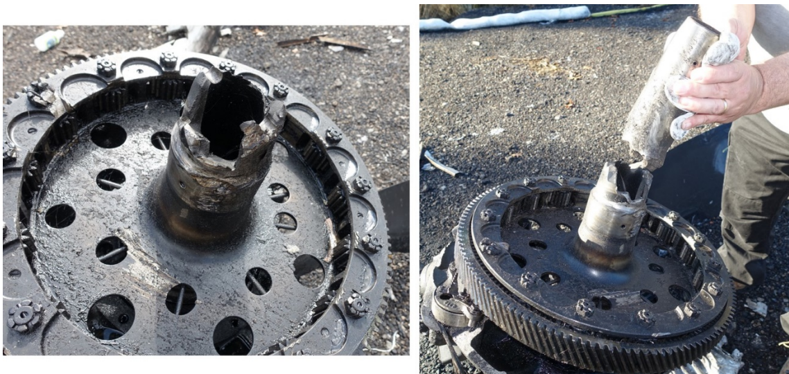
Photo 16- Right Propeller Shaft Separation
