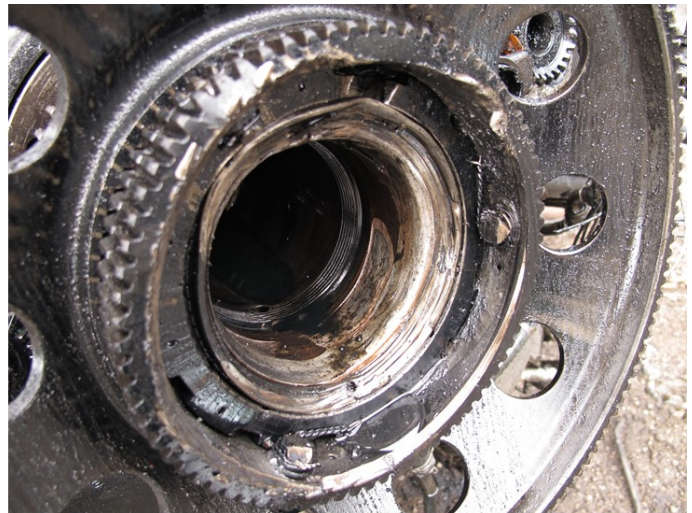
Photo 13- Reduction Drive Gear Deformation and Propeller Shaft Journal Scoring
