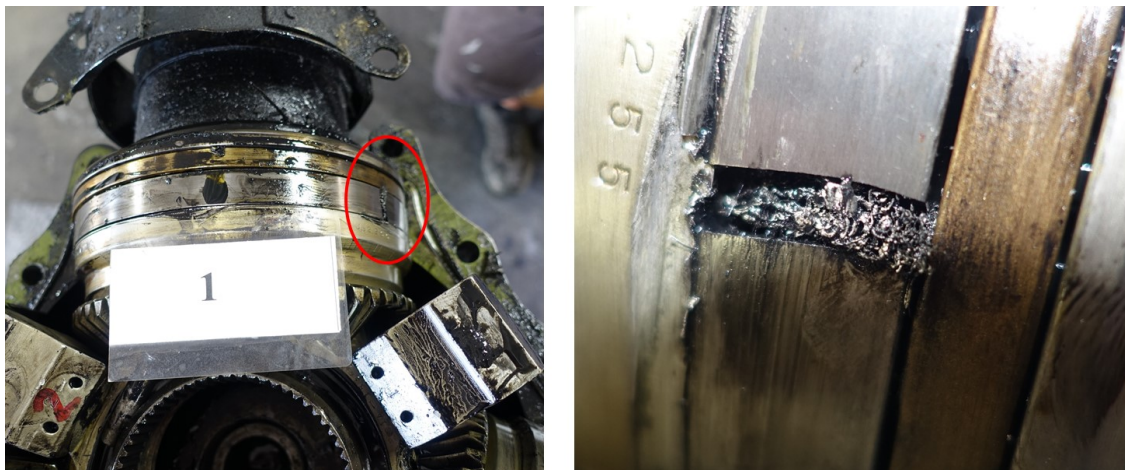
Photo 42- Blade 1 Thrust Bushing Split, (R) Metal Shavings in Split
