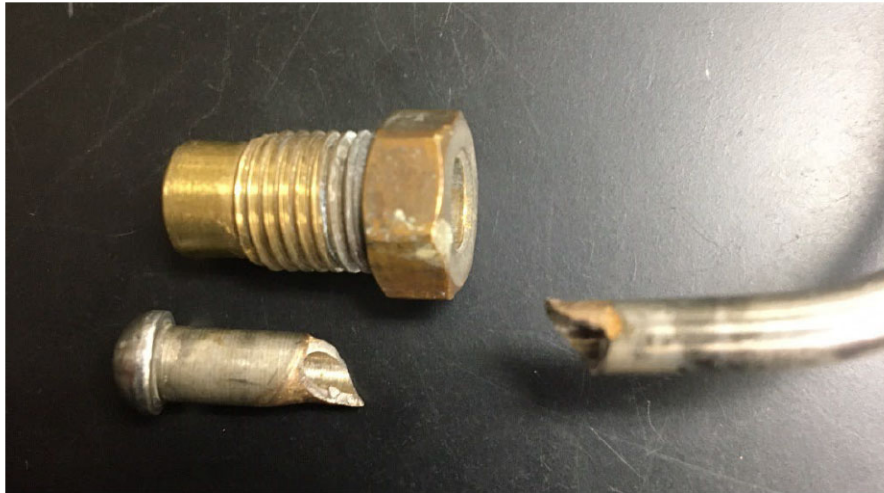
Figure 1 Fractured fuel line assembly with flared end (left) and tube (right)
