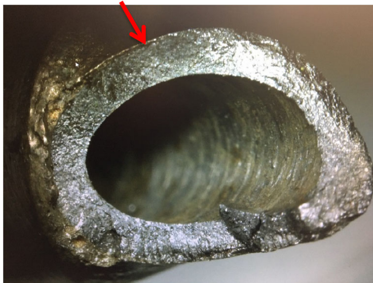
Figure 5 Side view of fitting end fracture with initiation area marked
