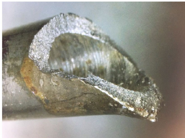
Figure 2 Side view of tube end of fracture
