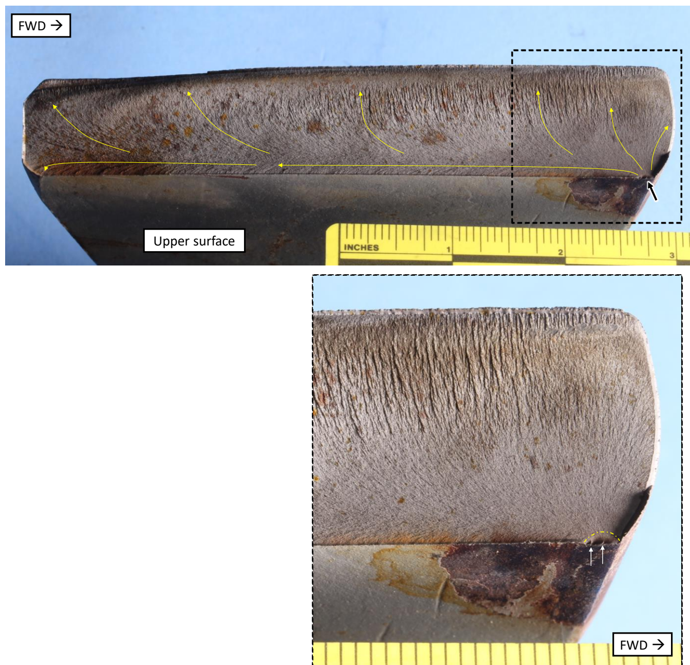
Figure 2: A photograph of the inboard fracture surface is shown above. Chevron patterns pinpointed the fracture origin at the corner of the upper surface and forward edge, indicated by the unlabeled black arrow. From the origin, the crack propagated aft and downward as indicated by the yellow arrows. A closer view of the origin is shown below from the area within the dashed black box, scale markings are 1/16 inch. A relatively flat and smooth thumbnail shaped crack, outlined by the yellow dashed line, and ratchet mark features, indicated by white arrows, were present at the fracture origin, consistent with fatigue initiation from multiple origins. Paint was chipped and absent from the surface adjacent to the origin and brownish-red oxidized metal was visible. Intact paint surrounding this area exhibited a light orange staining pattern.
