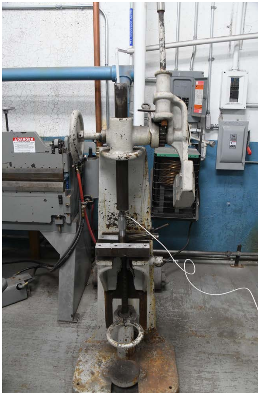
Photo 30 - View of a setup to measure the pressure required to displace connecting rod bushings.
