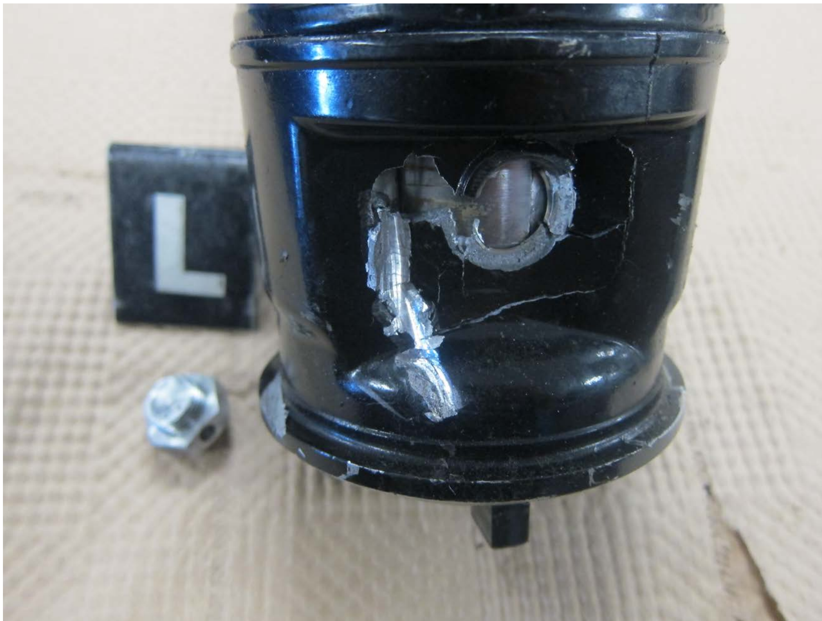
Photo 37 – Supplied view of the left magneto. The magneto exhibits damage witness marks.
