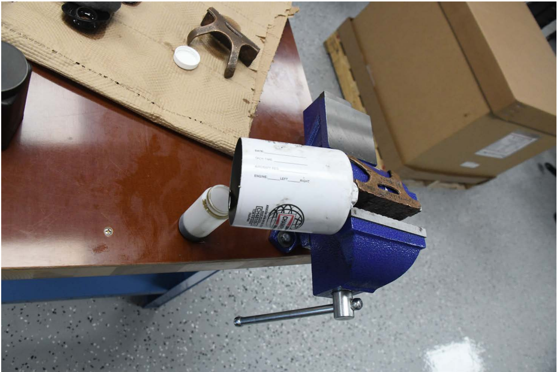
Photo 27 - View of the contents of the oil filter being drained in to the sample container.
