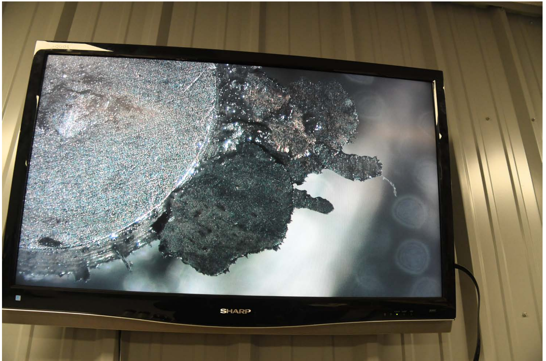
Photo 20 - Magnified view of particles attached to the magnetic plug from the oil sump pan.
