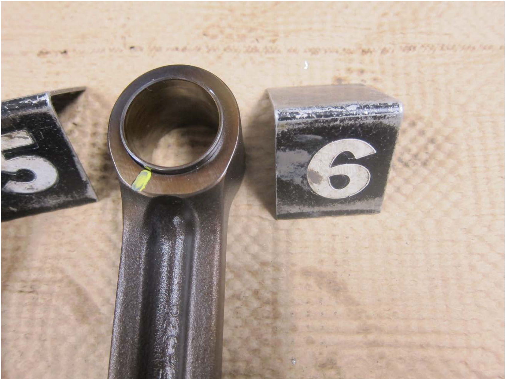
Photo 39 – Supplied close up view of the No. 6 connecting rod. Its bushing split is marked.
