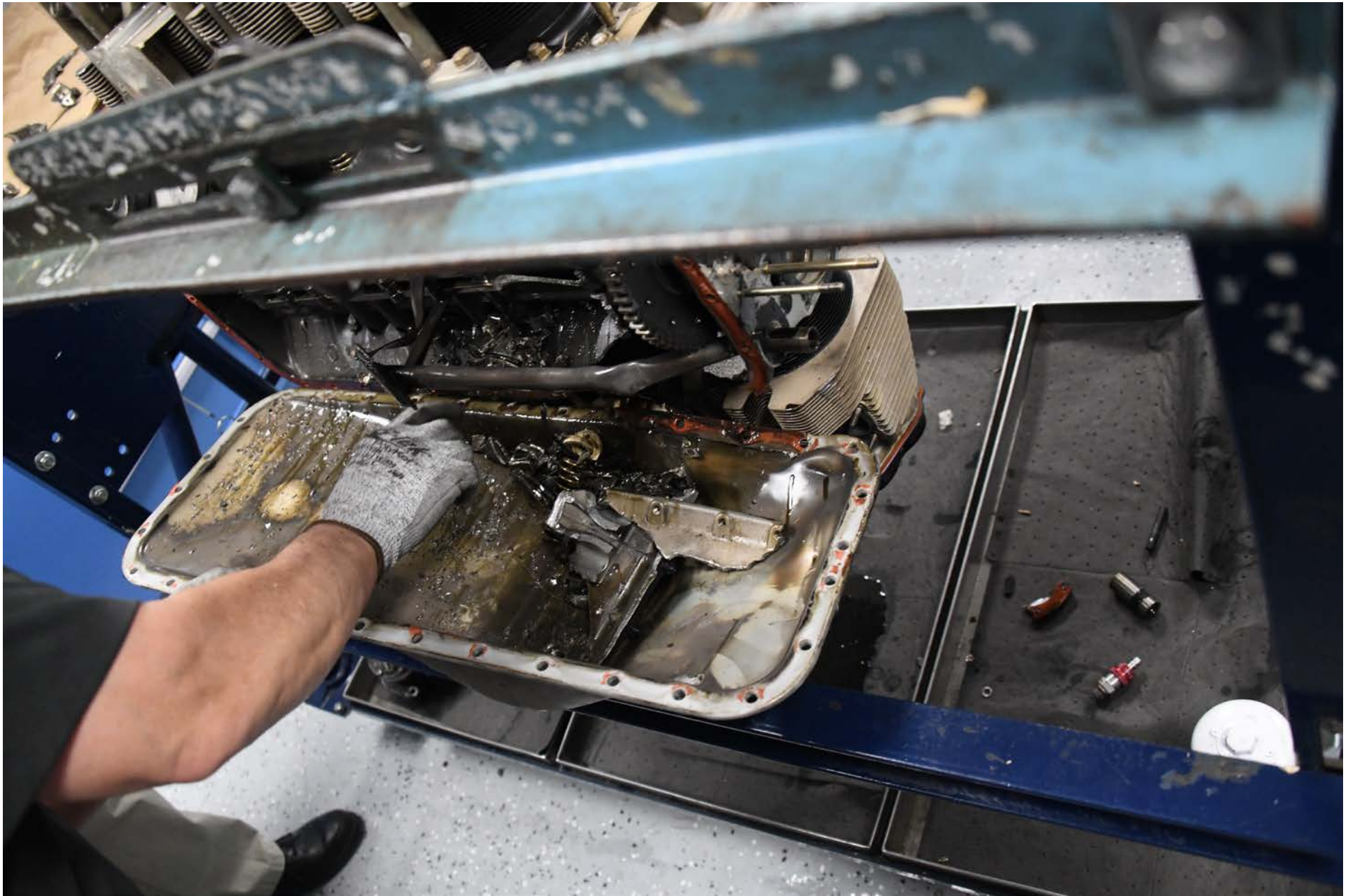
Photo 12 - View of the oil sump pan as it is being removed.
