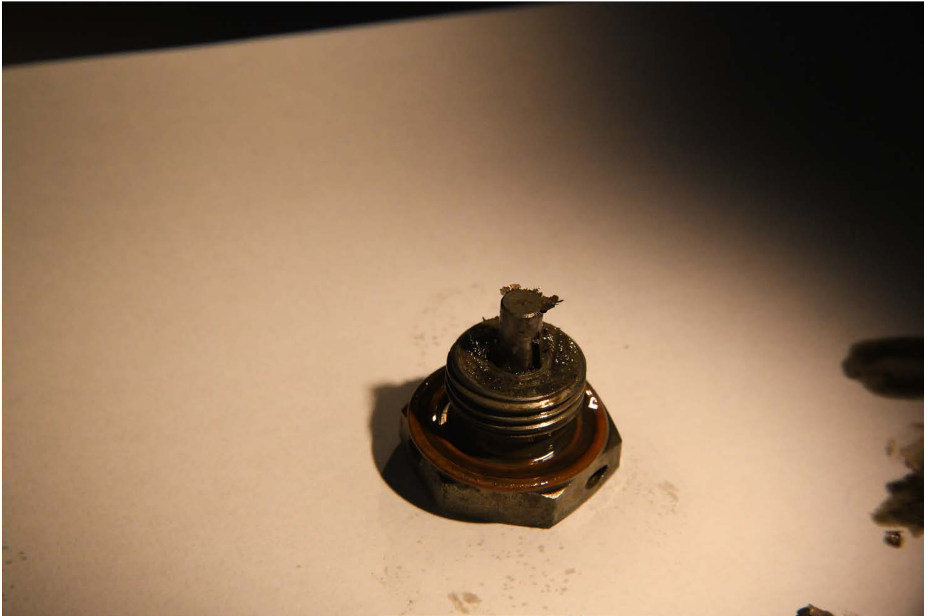
Photo 19 - Close up view of the magnetic plug from the oil sump pan.
