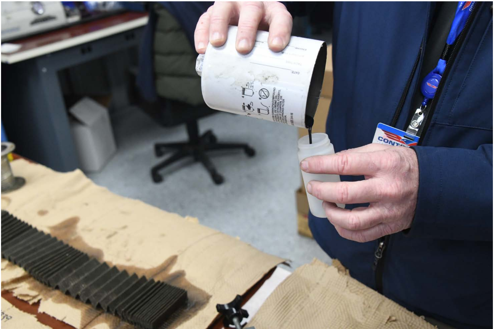
Photo 26 - View of the oil filter contents being poured into a sample container.
