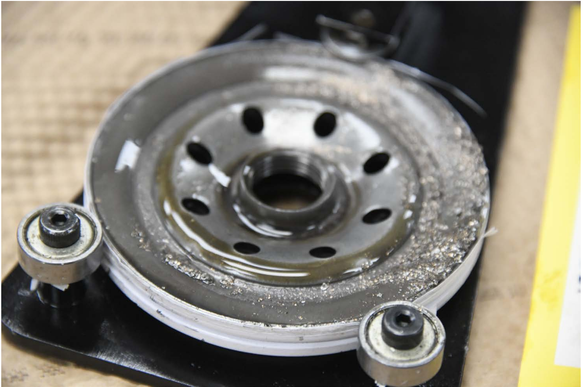
Photo 24 - View of the cut open oil filter. Particles are observed on the internal side of the filter base.
