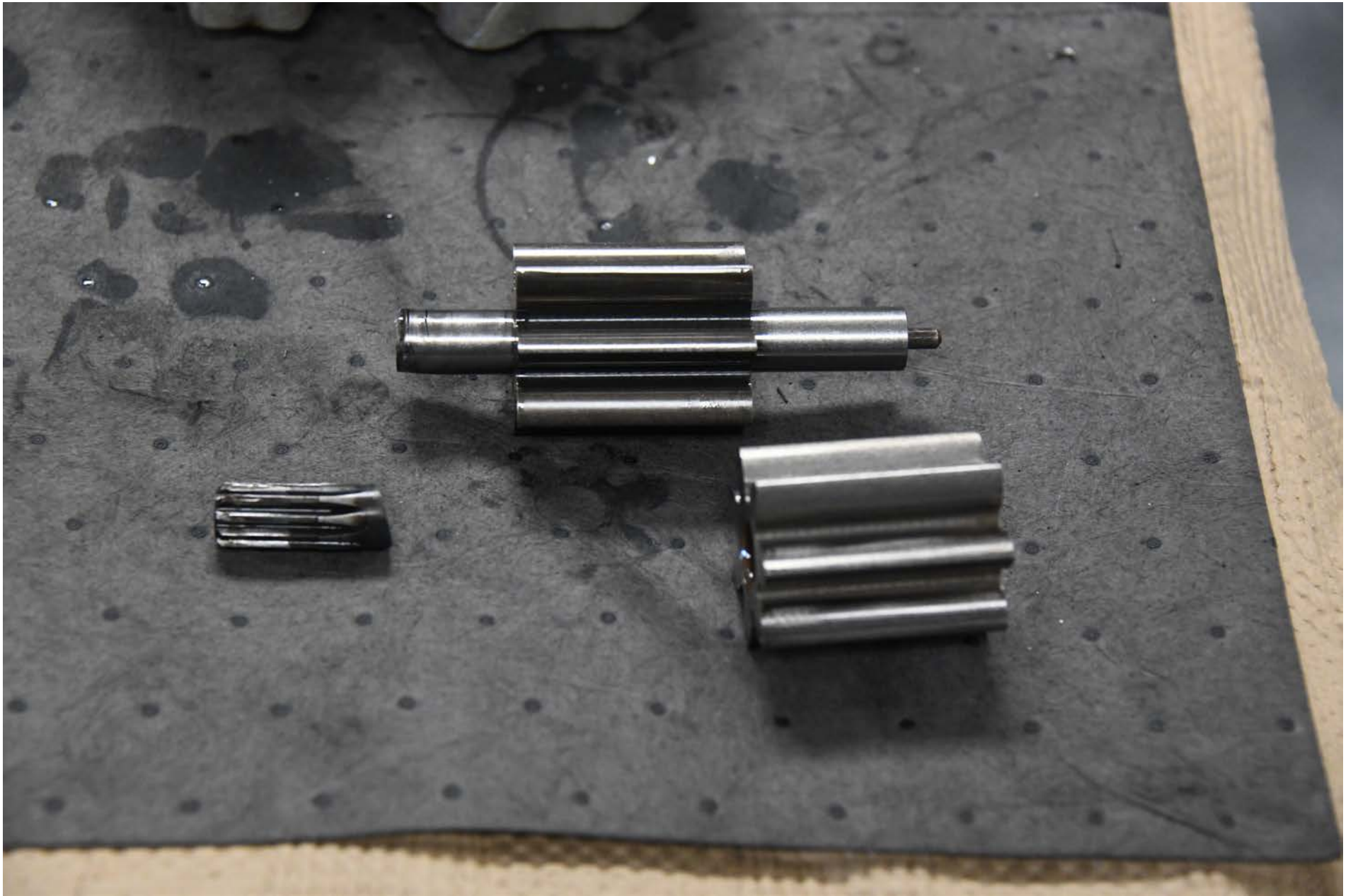
Photo 11 - Close up view of the oil pump's drive and driven gears. No marks are observed on the gear's surfaces.
