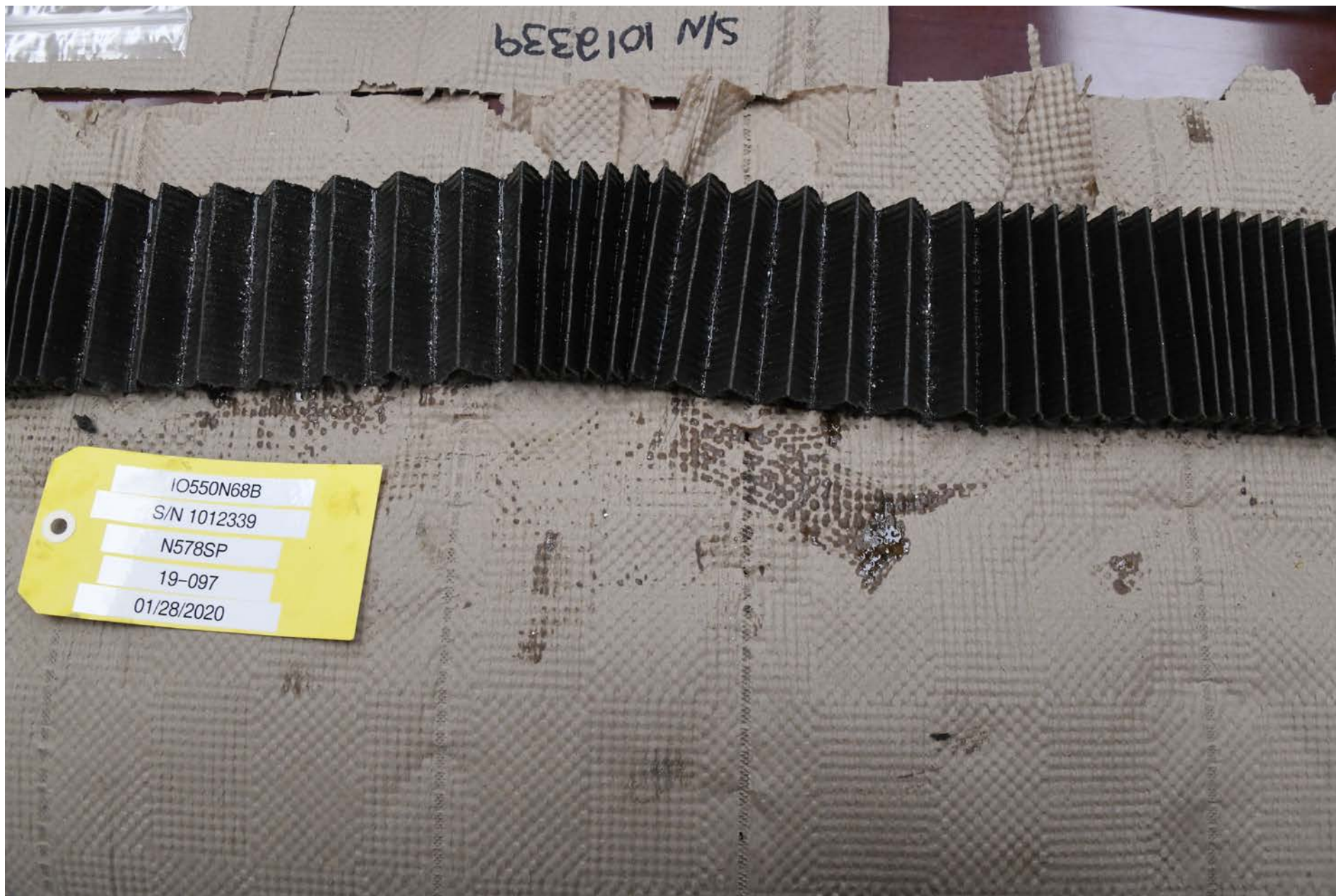
Photo 25 - View of the removed filter element from the oil filter. Particles are observed on the pleats within the element.
