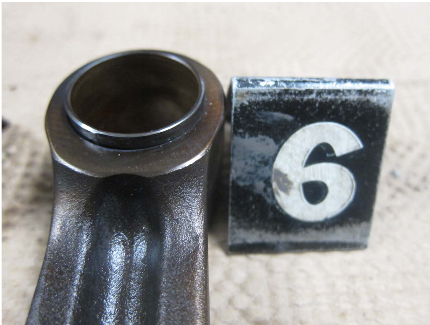
Photo 38 – Supplied close up view of the No. 6 connecting rod. Its bushing is displaced.
