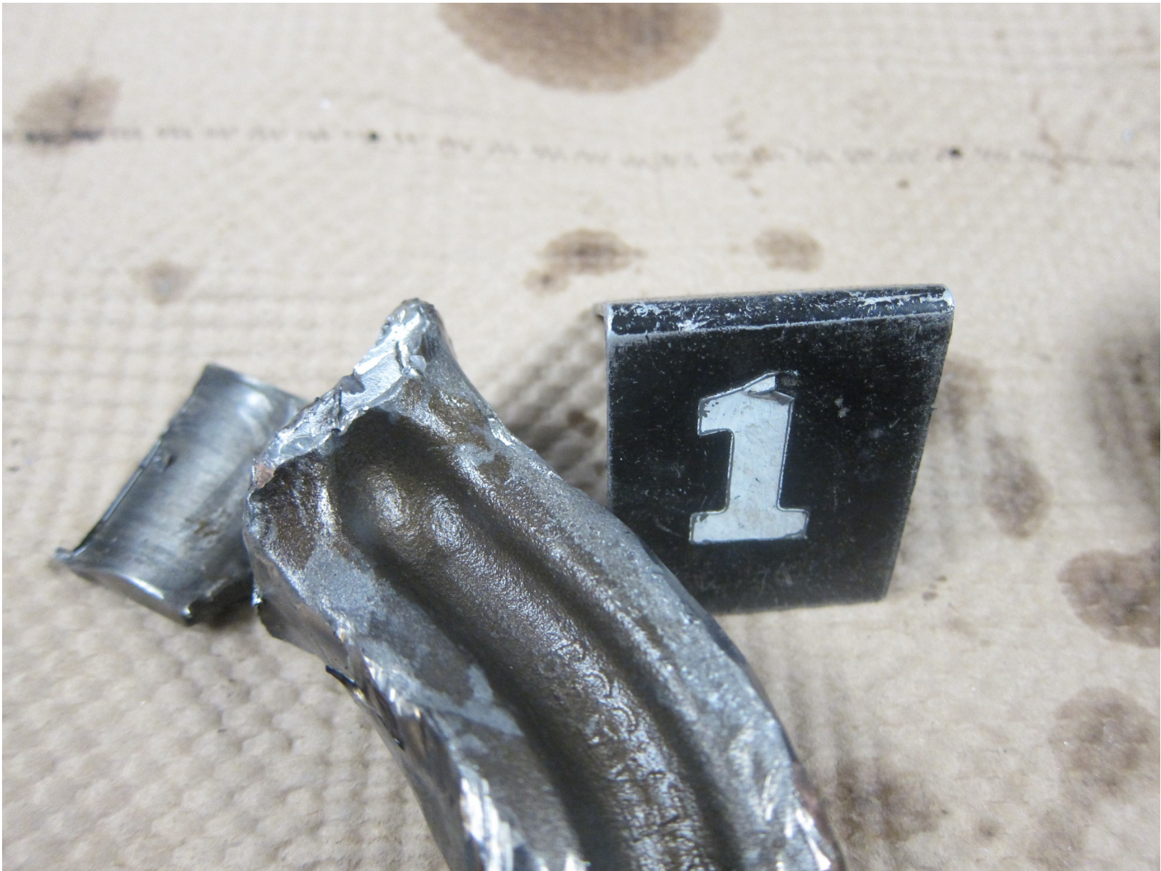
Photo 31 – Supplied close up view of the No. 1 connecting rod and a separated section of its rod end.
