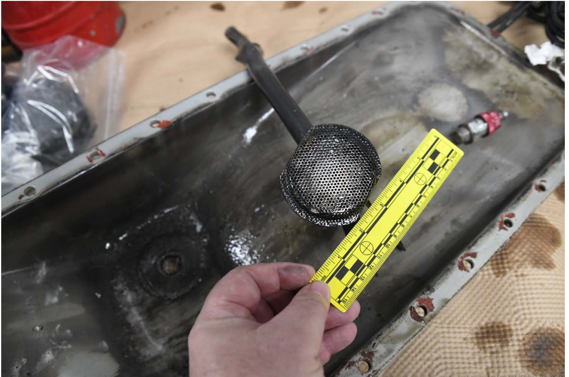
Photo 21 – View of the pickup tube from the oil sump area.
