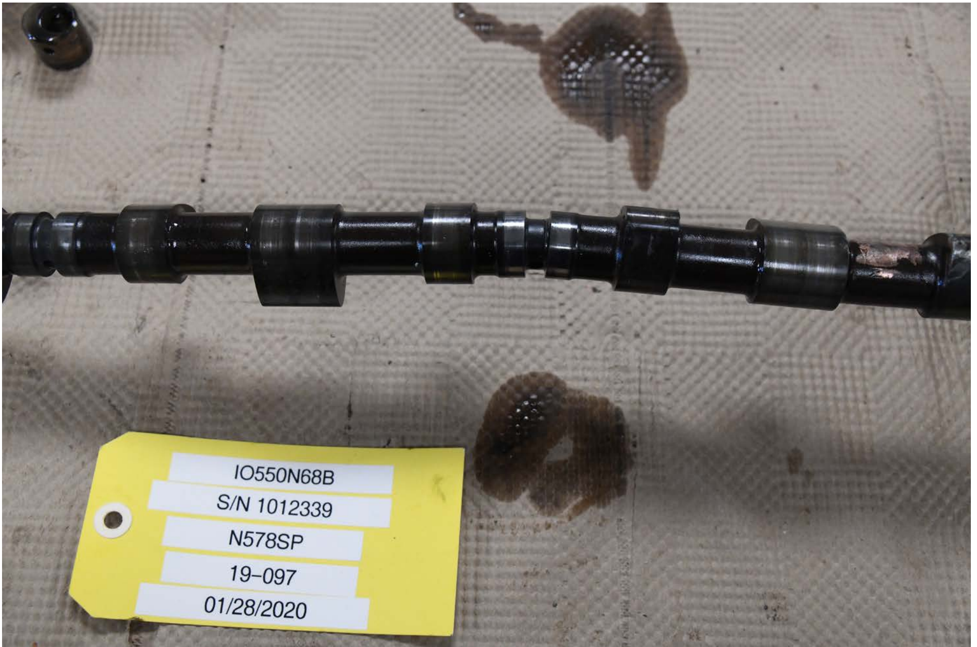
Photo 17 - Close up view of the bent camshaft.
