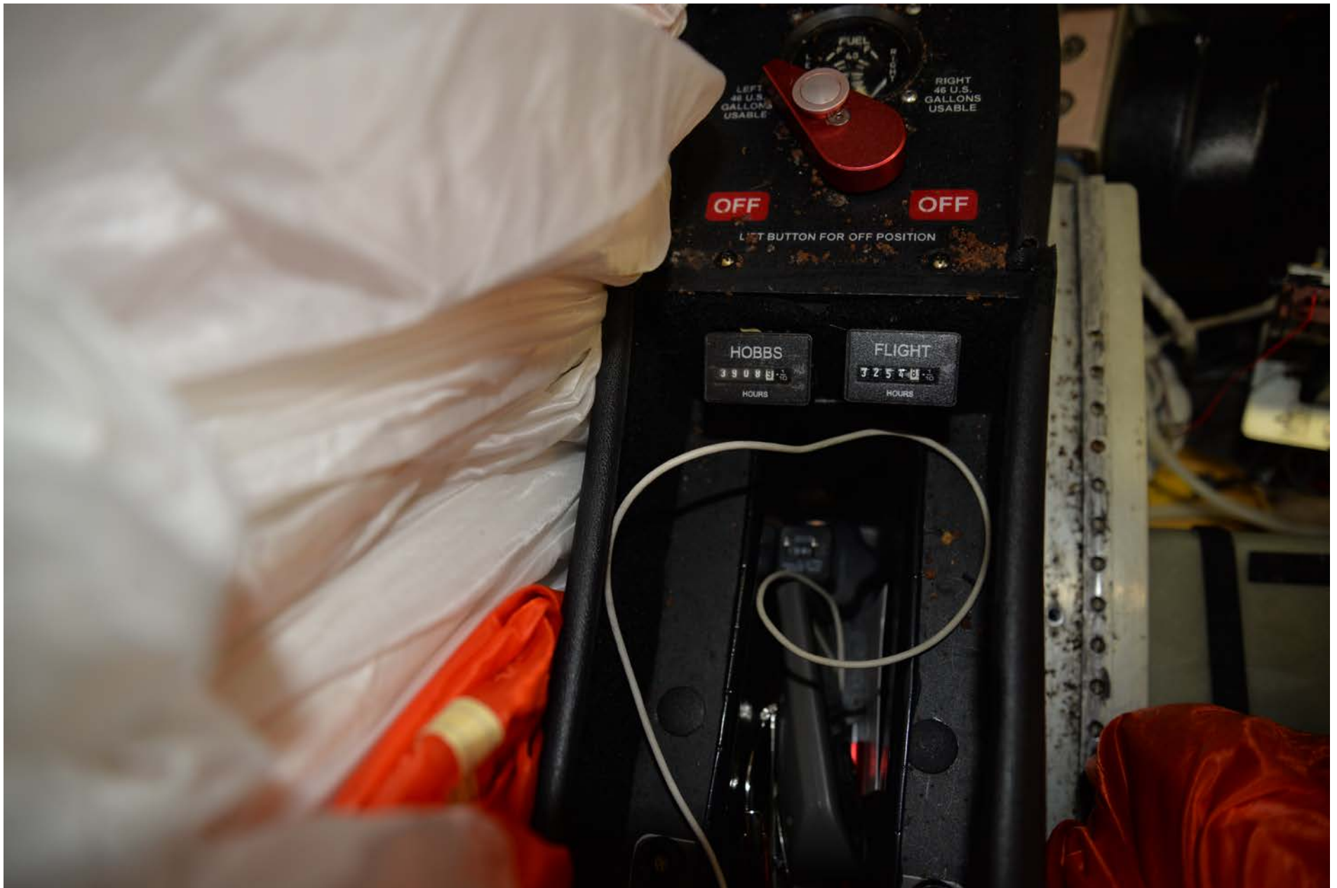
Photo 6 - View of the Hobbs and flight time meters. The Hobbs indicates 3,908.9 hours and the flight indicates 3,254.8 hours.
