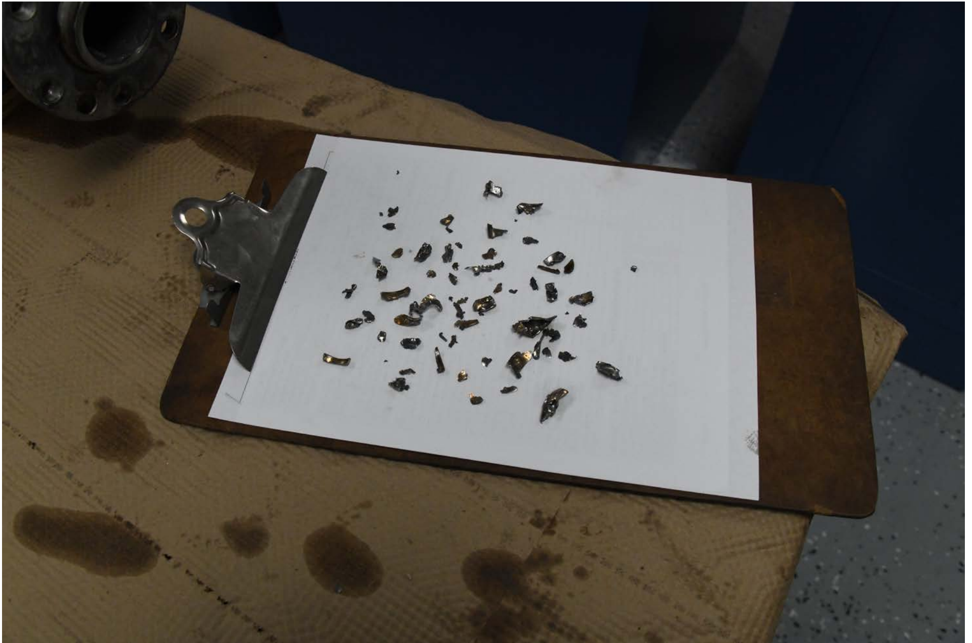
Photo 23 - View of media removed from the sump pan using a magnet.
