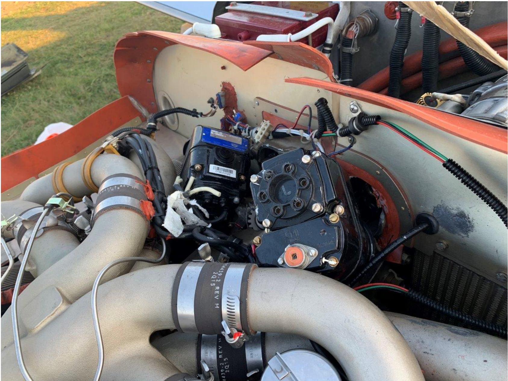
Photo 1 – View of the top of the engine at the accident site. Both magnetos are displaced from their designated locations.
