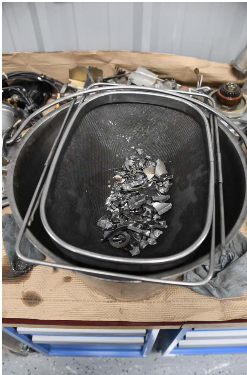
Photo 22 - View of media from the oil sump pan.
