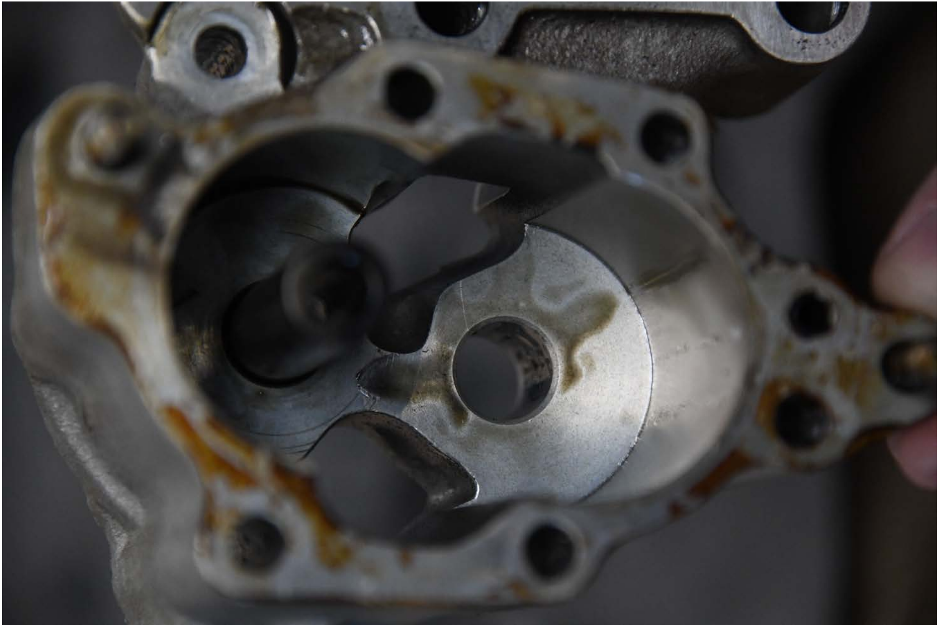
Photo 10 - Close up view of the oil pump cavity. No marks consistent with passage of hard particles are observed on the cavity's walls.
