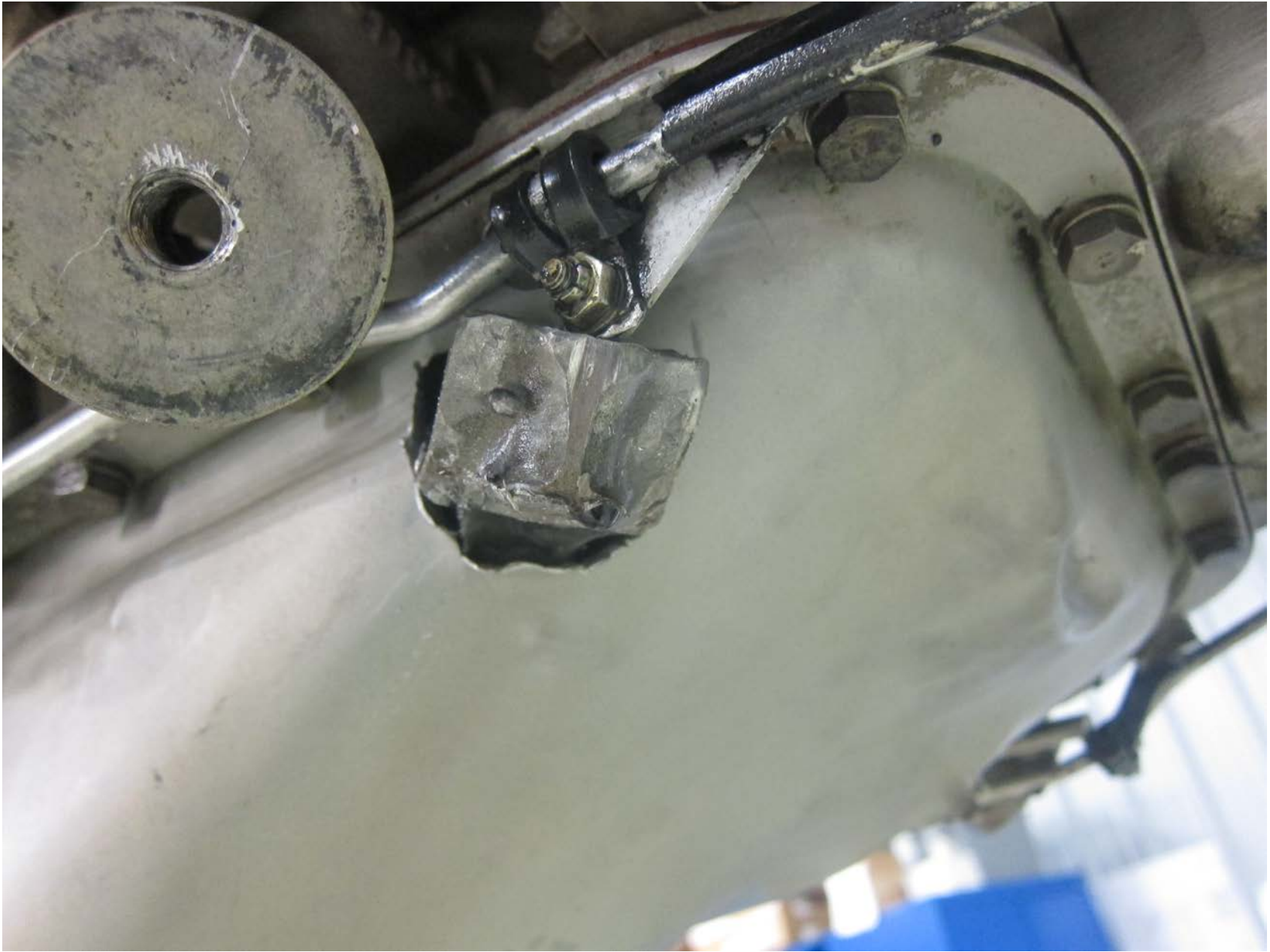
Photo 36 – Supplied view of the oil sump pan. An end of a connecting rod is observed in a hole in the pan.
