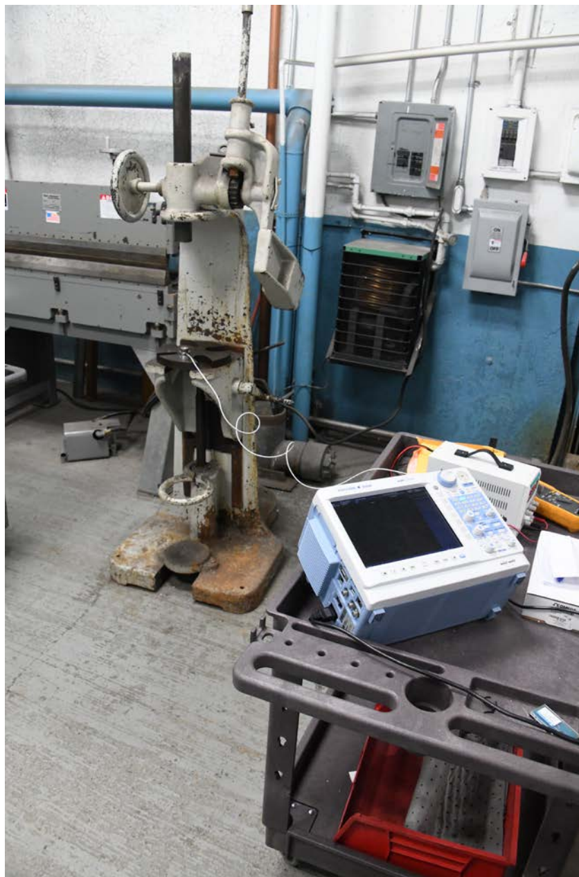
Photo 29 - View of a setup to measure the pressure required to displace connecting rod bushings.
