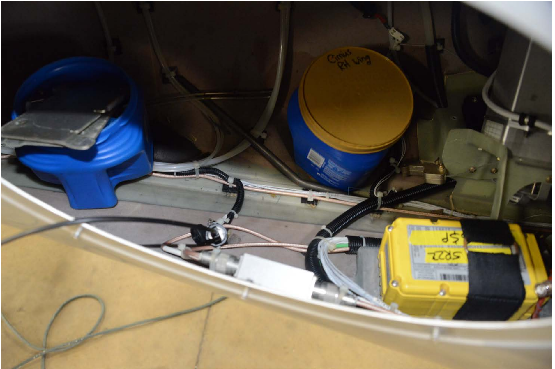
Photo 3 - View inside of the right side of the empennage. A port is viewed through which an RDM download is being conducted.
