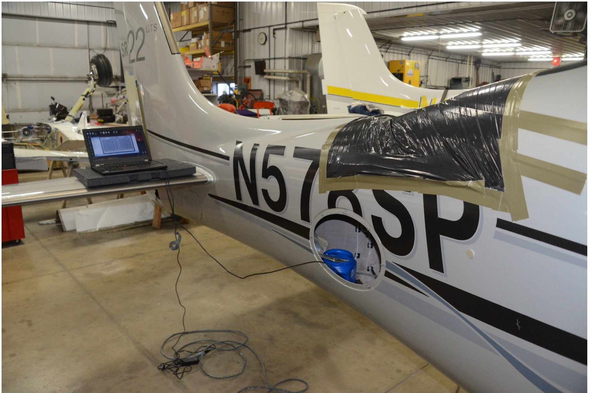
Photo 2 - View of the right side of the empennage in a recovery facility. A computer is viewed performing an RDM download.
