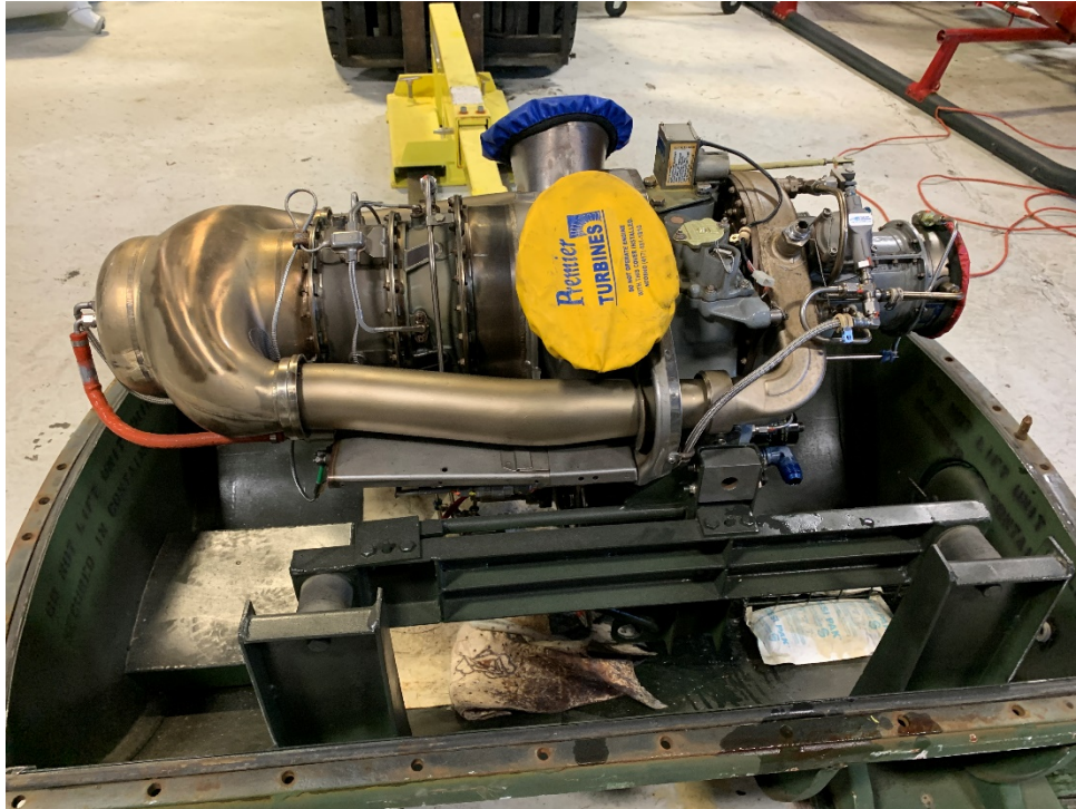
Figure 4: View of the engine installed in the engine shipping container.
