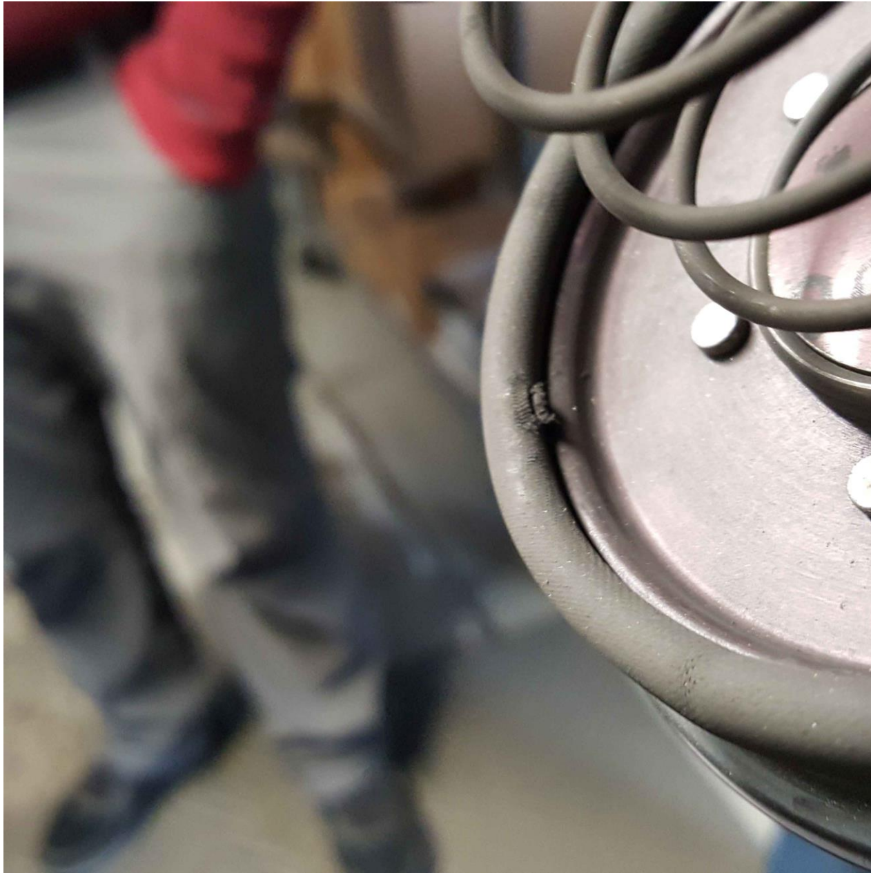
Photo 14 – Wastegate Diaphragm Hole (Merlyn Photo)
