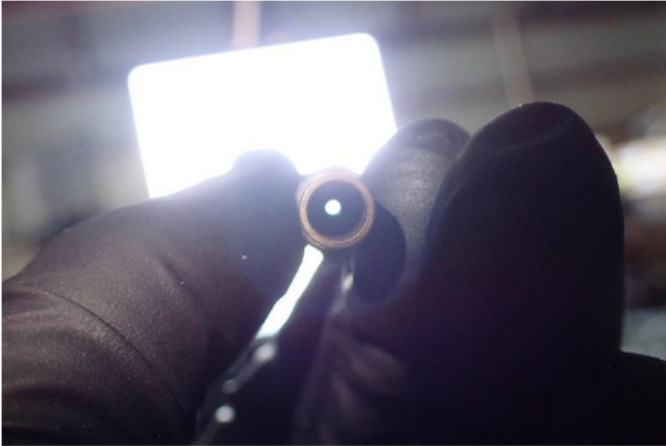
#1 Nozzle (after air was blown through the inlet)
