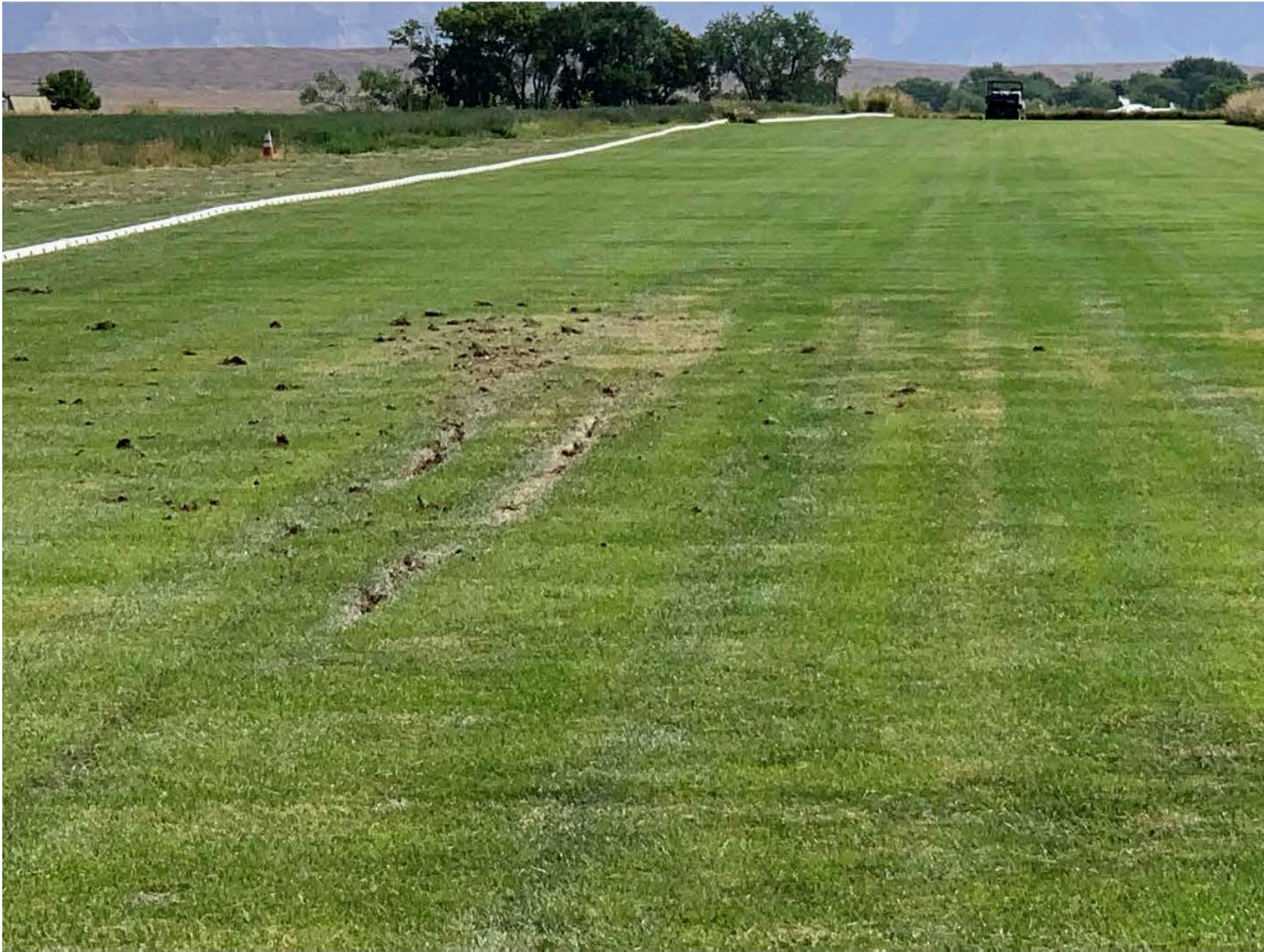
Photo 1 – When N2XF made its forced landing, it went off the end of runway 7. Gouges in the ground were caused by the partially extended main landing gear. Irrigation pipe is at left and aircraft is in background
