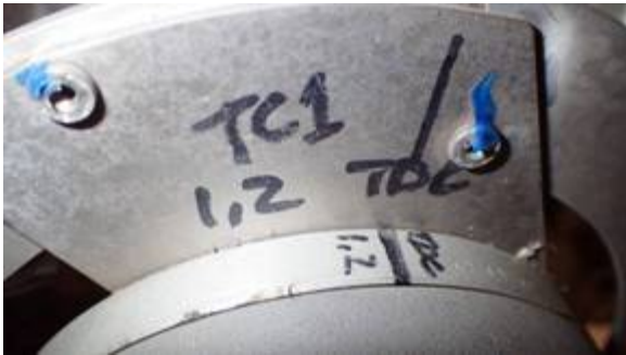
Threaded inserts for screws on back of bracket
