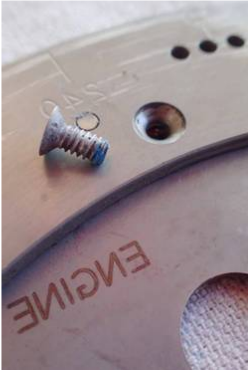
Flush head 6-32 attach screw
