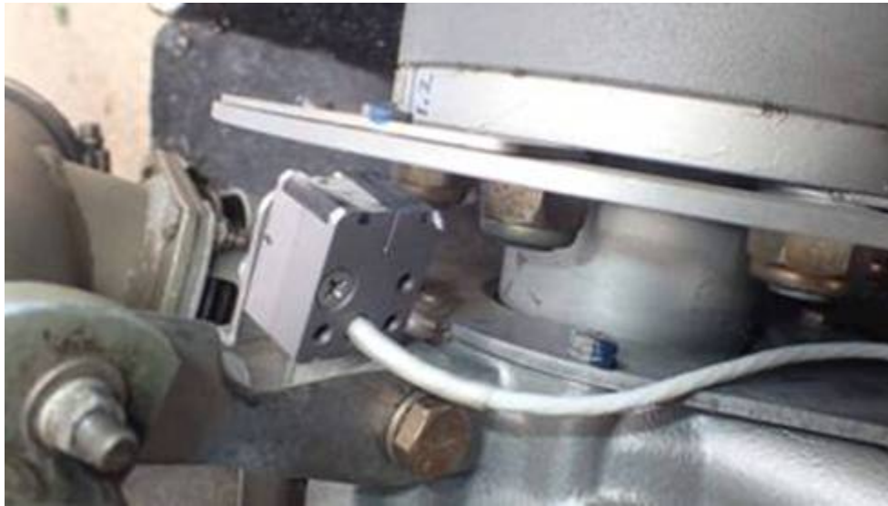
Timing ring loose and separated from bracket
